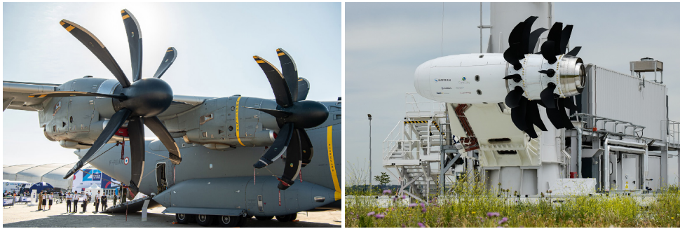
(a) Variable pitch propellers of the Airbus A400M. Copyright: Airbus.
