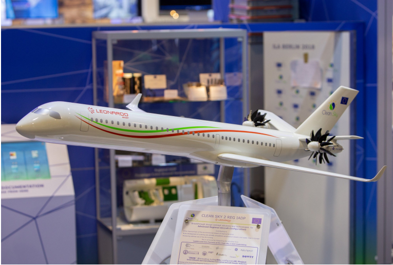
Figure 1.5: The CleanSky IRON configuration with propellers mounted to the horizontal tail. Credits: CleanSky.
