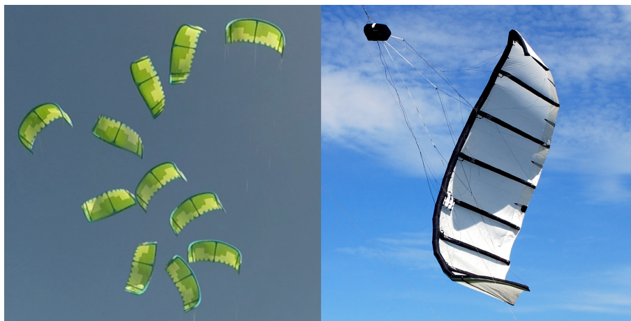
Figure 1. Time-lapse composite photo of a 6 m 2 power kite for sport applications performing a sharp turn to the left and subsequent loop manoeuvre, taken from the towing vehicle, from Lange (2018) (left panel). Photo of a 25 m 2 power kite for airborne wind energy applications performing a turn to the right during a mast-based launch manoeuvre, reported by Oehler and Schmehl (2019) (right panel). Both photos illustrate the spanwise twist deformation exhibited by LEI kites. The extreme deformation in the right photo does not occur in regular flight operations but resulted from mast-based launch attempts, shown here only to visualize the wing twist mechanism.
