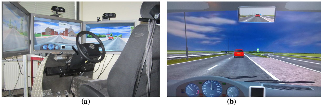
26 FIGURE 1 The medium-fidelity fixed-based driving simulator (a) and the driving simulation 27 environment in the two-lane highway (b).
