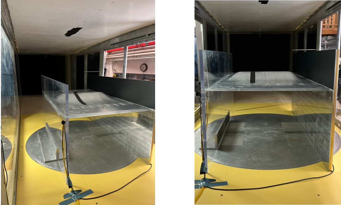
Figure 4.1: Boeing Gaussian Speed Bump model ( L = 0.914 m) installed in the Lucas Wind Tunnel.
