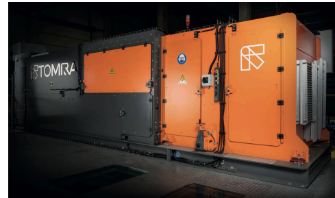
Figure 2.9: TOMRA AUTOSORT™ PULSE dynamic LIBS sorting system [22] .
