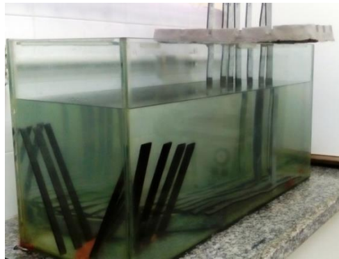
Fig. 3 Specimens in salt water tank
