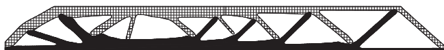
FIGURE 2 Optimized continuum topology as generated by the TopOpt Grasshopper 19 plugin outlined by submitter group A (black—tension, hatched—compression).
