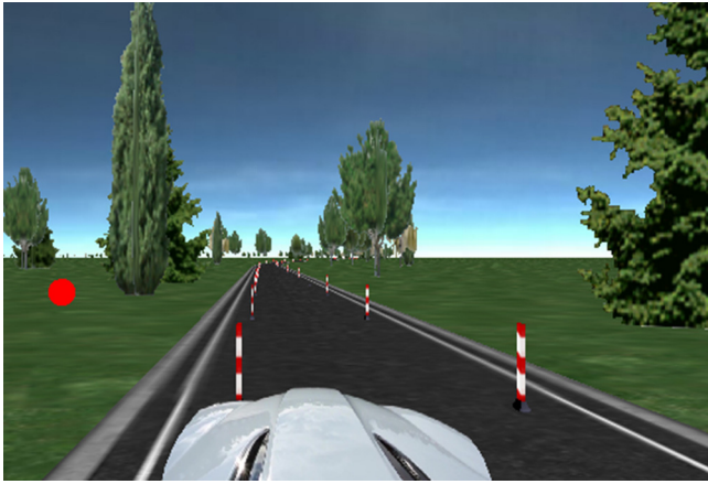
Fig. 1. Simulator environment including the car front and cone hit warning (i.e., red dot). (For interpretation of the references to colour in this figure legend, the reader is referred to the web version of this article.)
