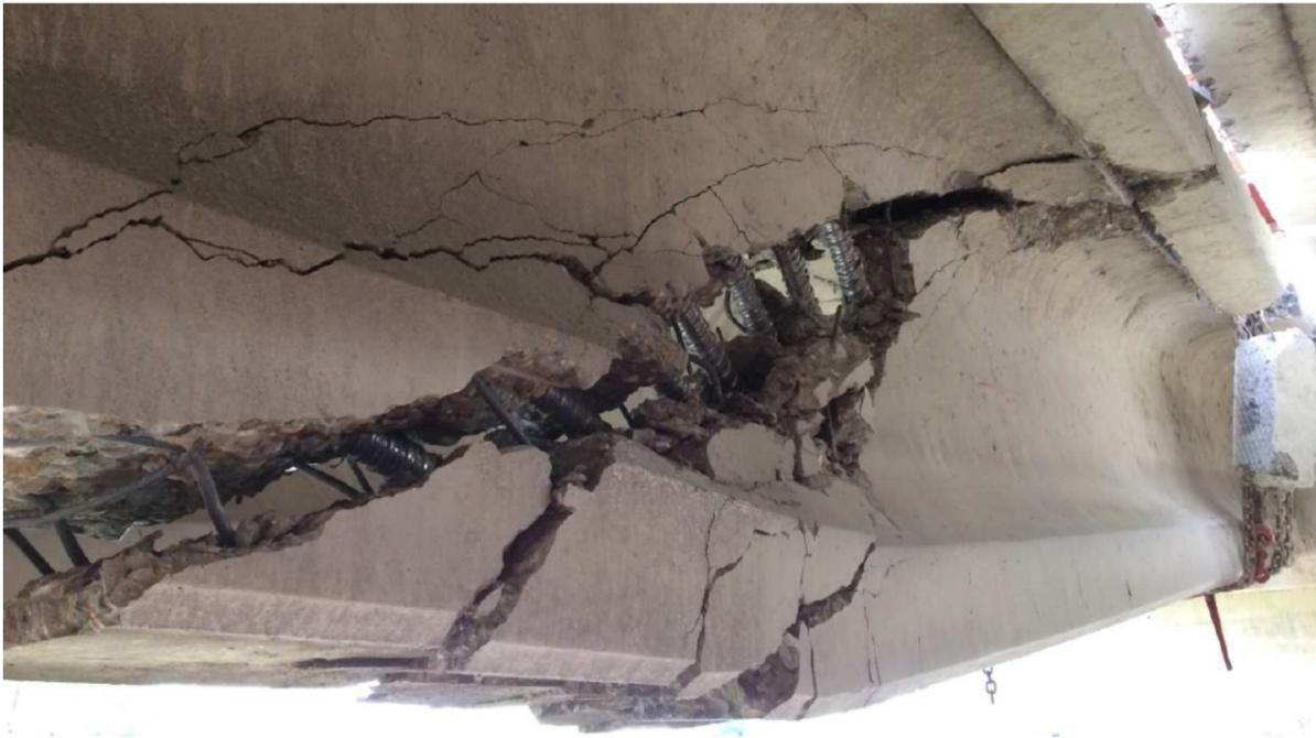
Figure 6.30: Cracks after test 7 [13]
