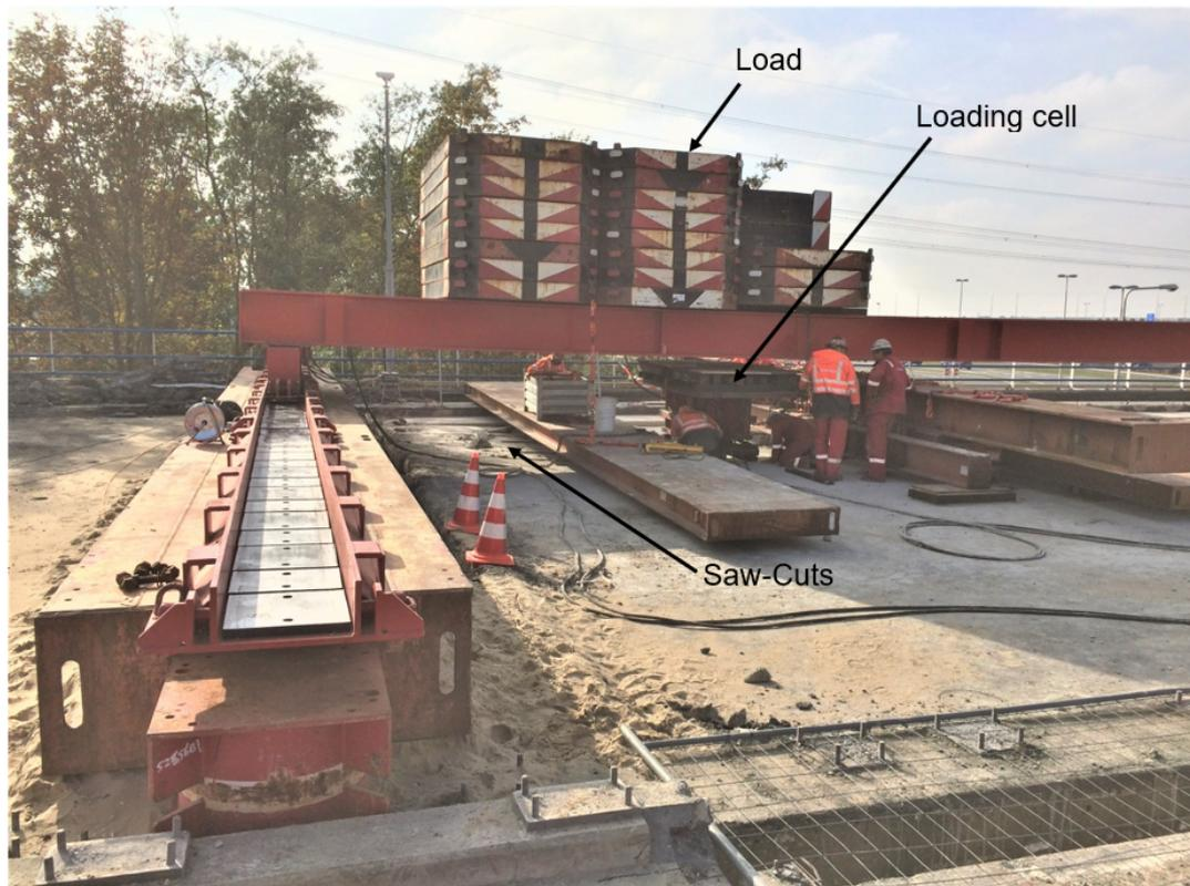
Figure 5.9: Overview of the test set-up used at site
