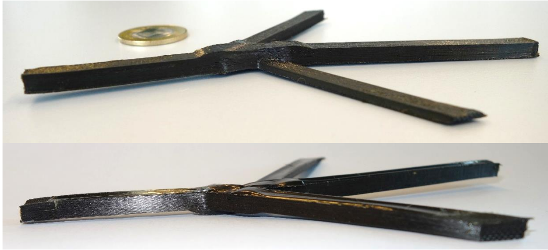
Figure 5.13 Joint test sample V2, showing better compaction and more symmetrical thickness build-up
