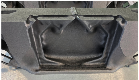
Figure 2.17: The first print attempt, showing the locally overheated and deformed parts, causing recoater damage.
