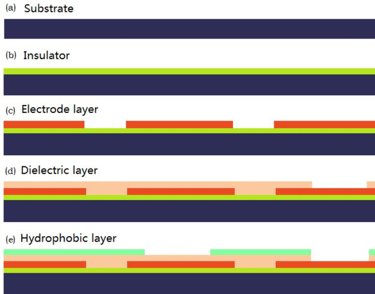
**Figure 4-1** The cross section of the multi-layer fabrication steps
