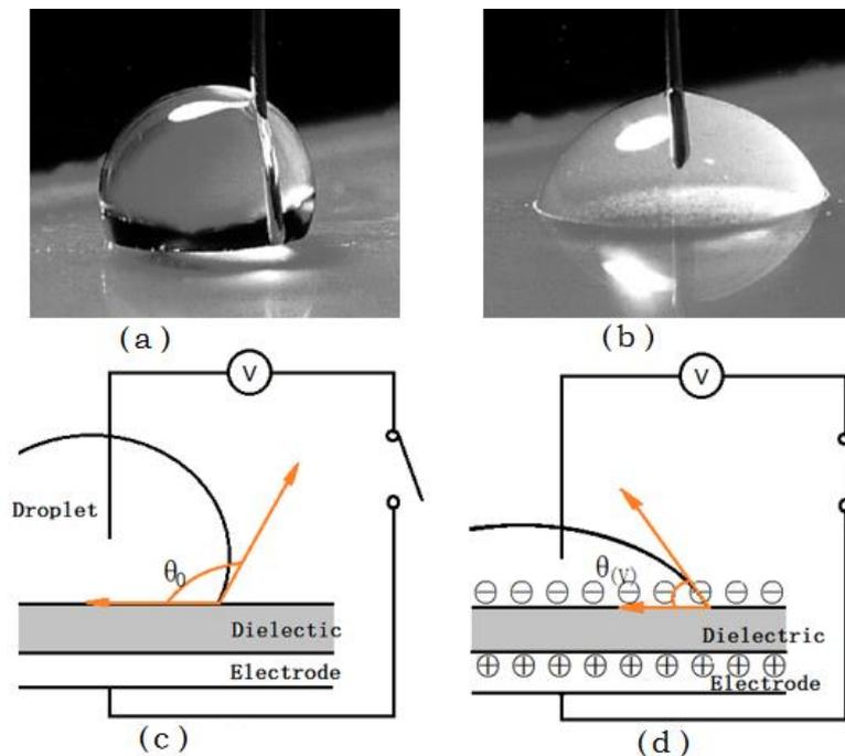
**Figure 2-3** Schematic of electrowetting-on-dielectric. (a, c) No external voltage applied: the droplet is a round shape and contact angle is more than 90 degree. (b, d) External voltage applied: charge density changes so that the contact angle decrease or increase.
