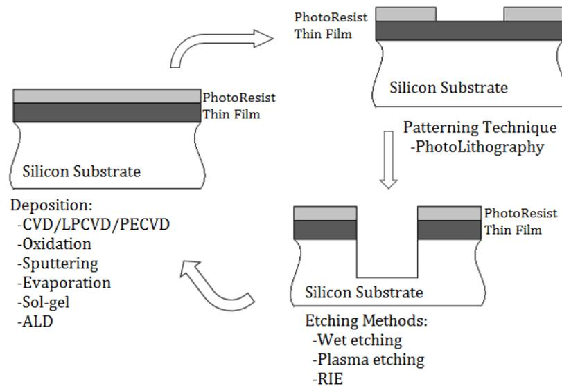
**Figure 4-7** Scheme of basic fabrication processes
