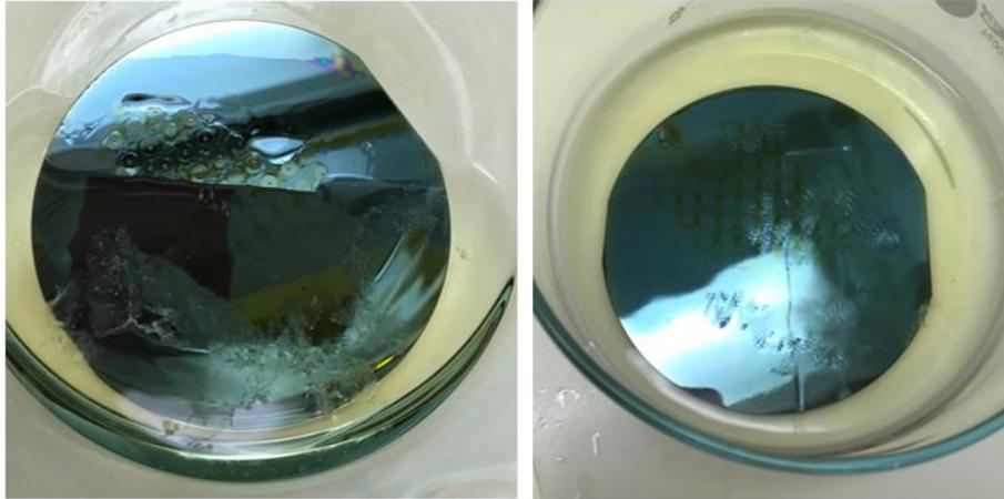
**Figure 4-13** Dipping in the acetone, the whole layer of FluoroPel peels off
