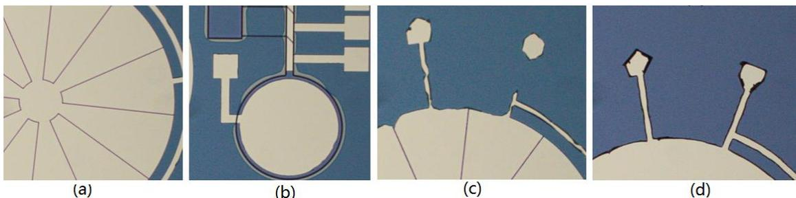
**Figure 4-11** Metal lift-off results
