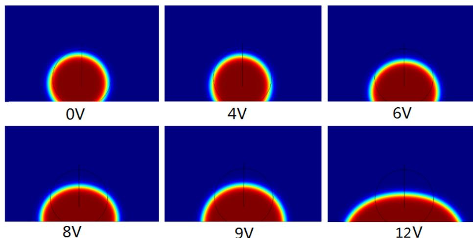
**Figure 3-3** Various stages of the droplet shape simulated by TPF physics
