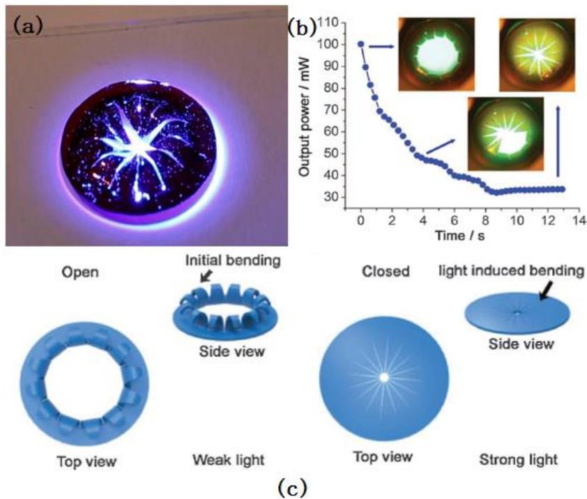
**Figure 1-2** (a) The overview of the LCE (b) Different states of the iris responding to different light power (c) Two boundary states of the pupil: under weak light and strong light. [6]
