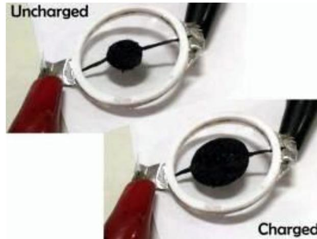
**Figure 1-3** An over-sized prototype pupil made from a dielectric elastomer actuator (DEA) [8] EAP technology makes the combination of the realistic pupil and iris hand-painted possible. However, in this work still much has to be done in size miniaturization as well as reducing the high voltage to a safe range.
