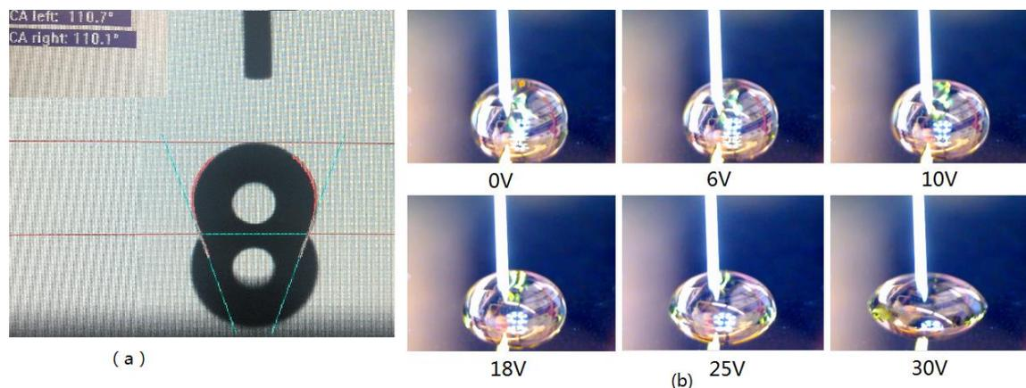
**Figure 5-2** (a) Contact angle of DI water on FluoroPel thin film; (b) images of the droplet (NaCl solution) at different voltages (DC)
