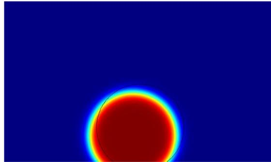
**Figure 3-2** Initial contact angle of the droplet (only effected by gravity)
