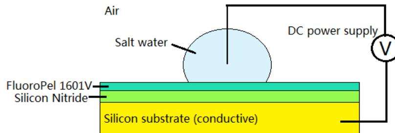
**Figure 5-1** Set up of the test of different thicknesses of dielectric
