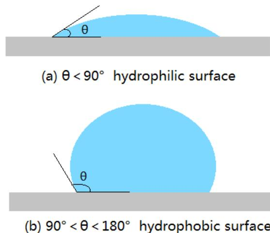
**Figure 2-1** Schematic diagrams of contact angle of a liquid droplet on solid surfaces
