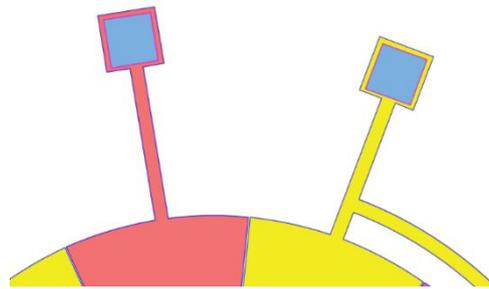
**Figure 4-3** Contact ‘via’ on the mask of dielectric layer (Blue squares).
