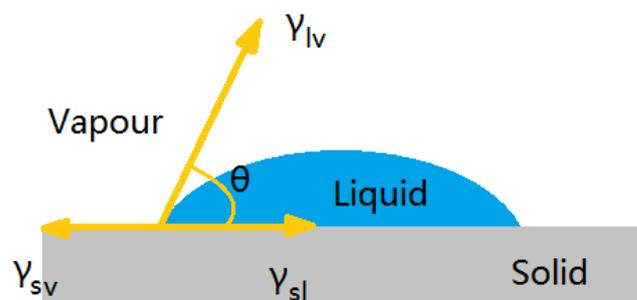
**Figure 2-2** Young's Equation for Three-Phase Interfacial Tension ( $\theta$  is the contact angle,  $\gamma_{sv}$  is the surface tension of solid-vapour surface,  $\gamma_{sl}$  is the surface tension of solid-liquid surface,  $\gamma_{lv}$  is the surface tension of liquid-vapour surface)
