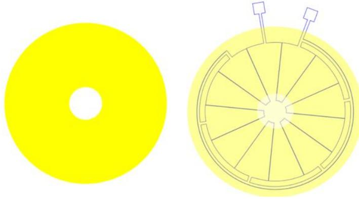
**Figure 4-4** Hydrophobic layer mask of version two (Yellow part).
