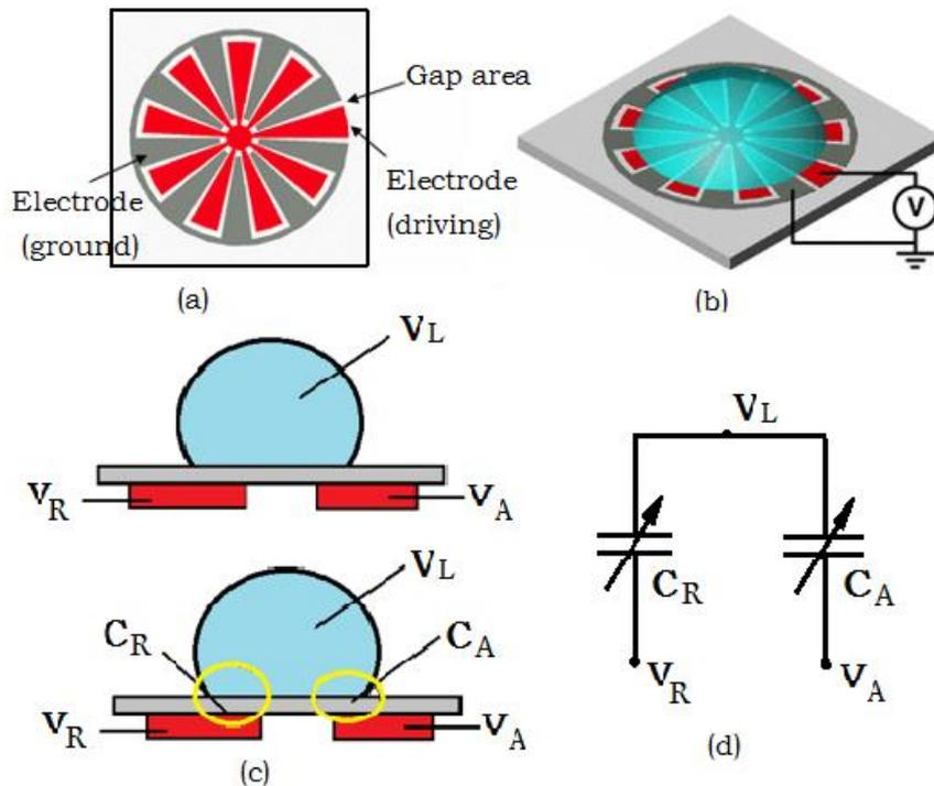
**Figure 2-7** EWOD of a droplet on single-side coplanar electrodes: (a) top view of the electrode arrangement [49]; (b) contact angle change with the applied voltage [49]; (c) cross-section view ( $V_A$  is the applied voltage,  $V_R$  is the ground voltage,  $V_L$  is the voltage of the droplet,  $C_A$  and  $C_R$  is the capacitance of the insulator between droplet and driving electrode or reference electrode, respectively); (d) equivalent circuit.
