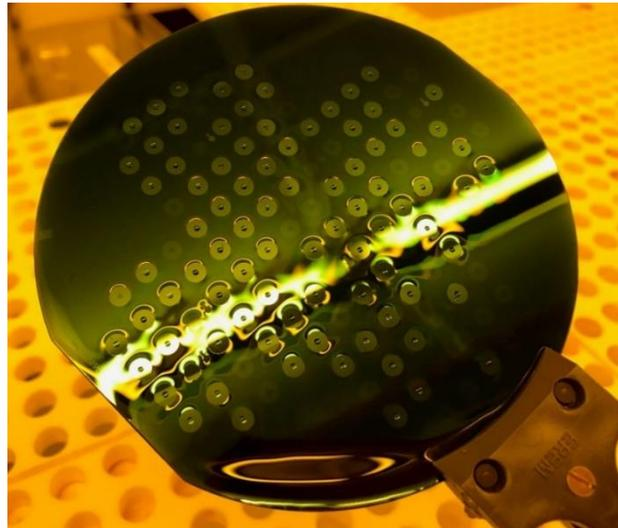
**Figure 4-15** after rinsing with water, the hydrophobic and hydrophilic area can be seen
