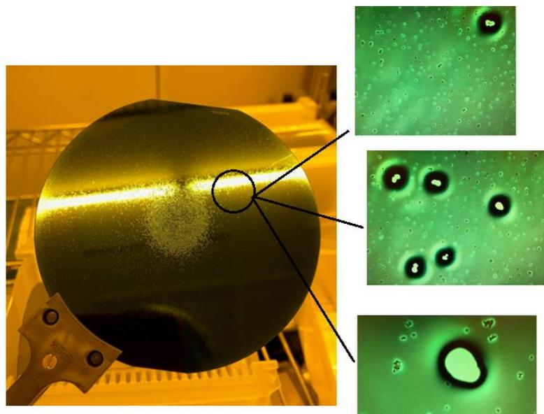
**Figure 4-14** Bubbles and holes on spray coated Photoresist results (1 layer)
