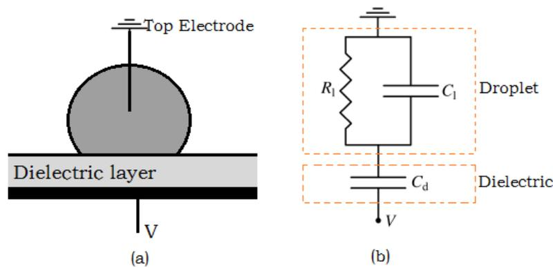
**Figure 2-5** (a) A droplet with separate electrodes EWOD configuration (b) equivalent simplified circuit diagram.
