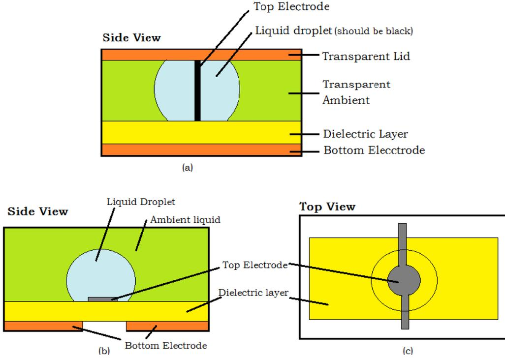
**Figure 2-6** (a) side view of the setup with a standing through probe; (b) side view of the setup with a patterned electrode on the substrate; (c) top view of (b), where the outer circle represents the droplet. The two connecting parts should be coated by a hydrophobic layer
