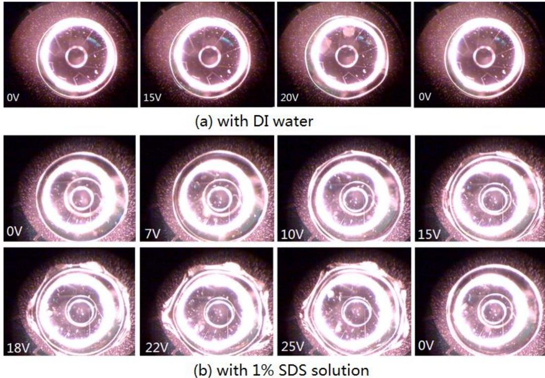
**Figure 5-4** Top view of the droplet surrounded by air over 30nm Al<sub>2</sub>O<sub>3</sub> and electro wetting electrodes. (a) DI water droplet images under different voltages (DC); (b) 1% SDS solution droplet images under different voltages (DC).
