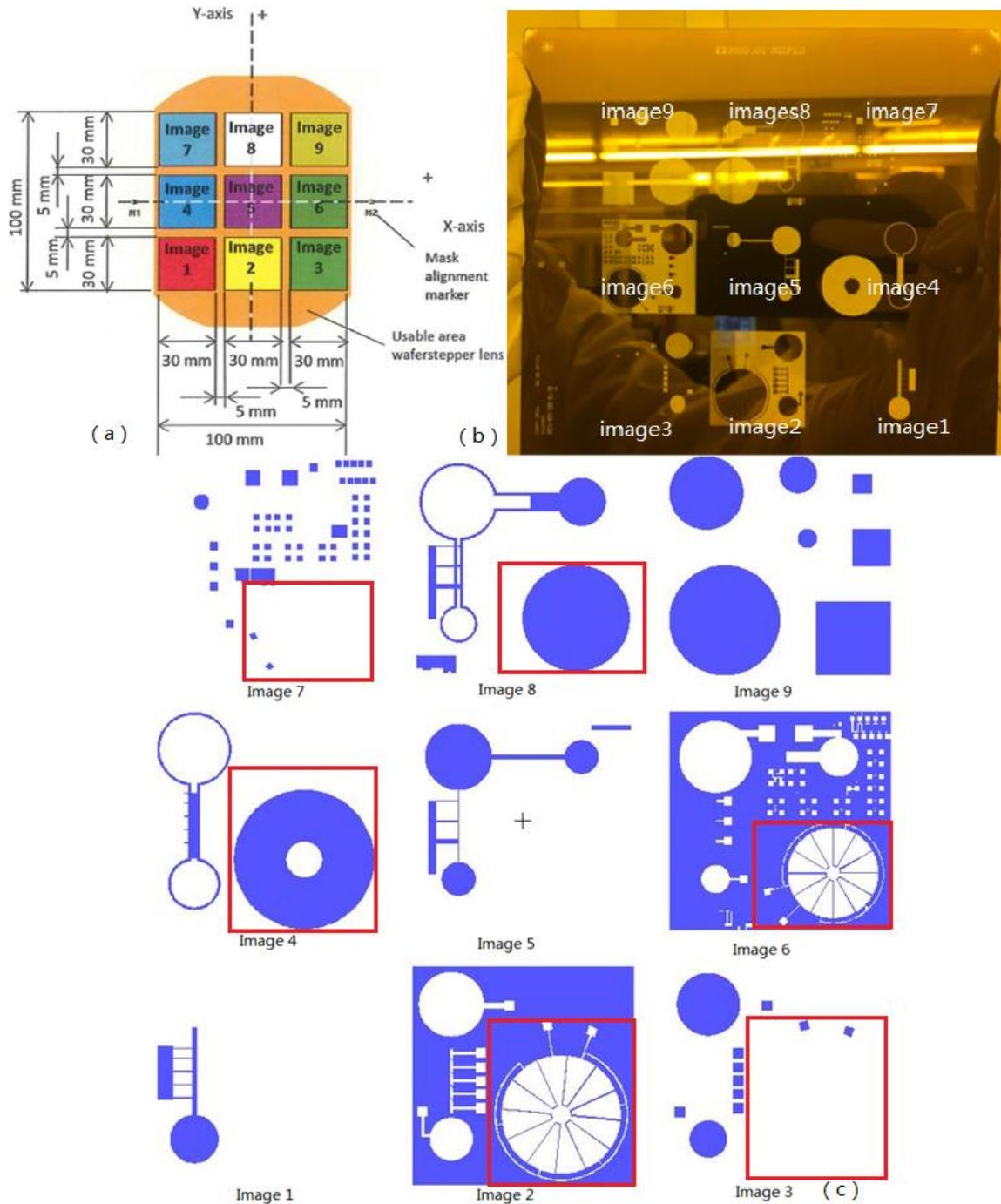
**Figure 4-6** (a) Mask layout with dimensions; (b) The mask product used for waferstepper; (c) Mask pattern overview
