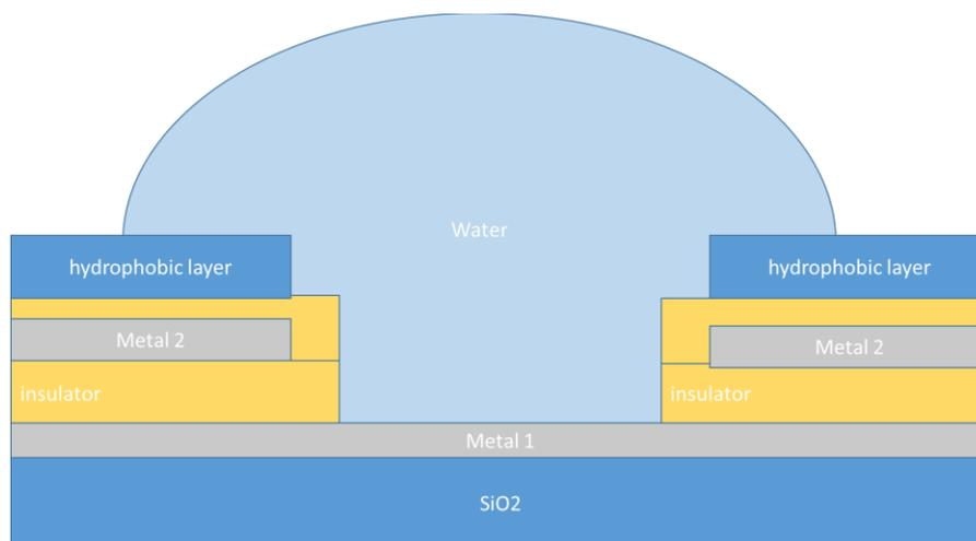
**Figure 6-1** Proposed design with concentric electrodes.
