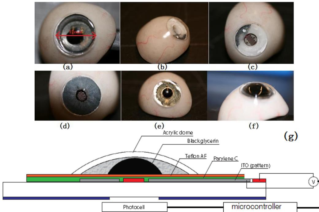
**Figure 1-4** The show model prototype schematic and assembly (a) The dimension of the iris; (b) Drilled and milled out prosthetic eye; (c) Light sensor placed inside the eye; (d) A hand-painted iris attached; (e) The electrowetting device placed; (f) Side view of the whole prosthetists; (g) The structure and details of the electrowetting device.
