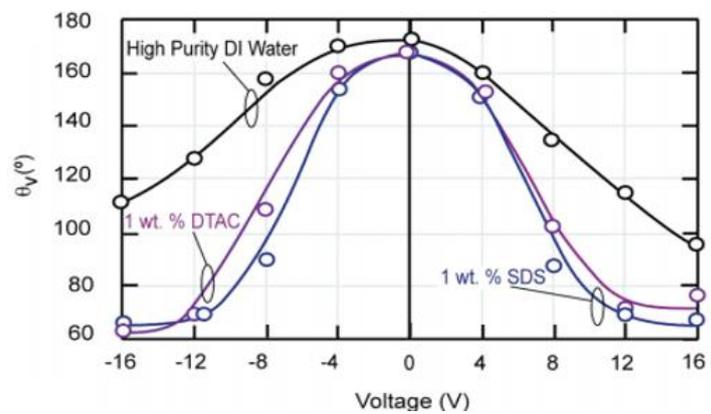
**Figure 2-4** Plot of contact angle vs electrowetting voltage for conventional solutions. [42]
