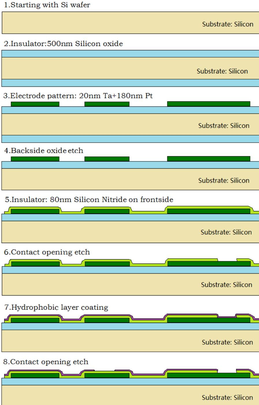
**Figure 4-9** The cross-section of main process steps
