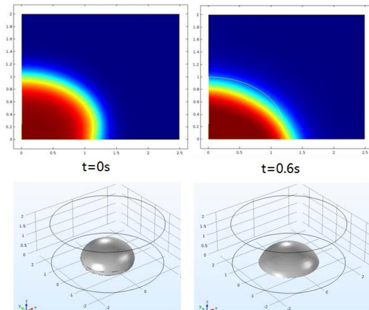
**Figure 3-5** The 2D and 3D plots of the droplet shape at  $t=0s$  and  $t=0.6s$  simulated by CIR, ES and TPF physics for a voltage of 70V
