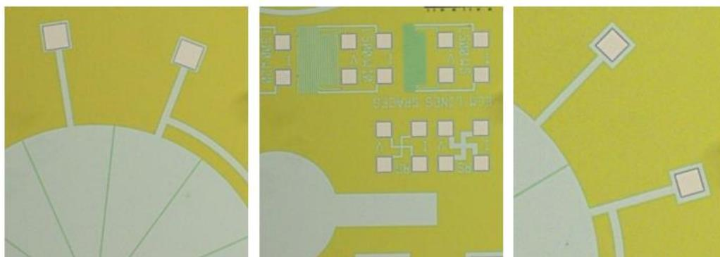
**Figure 4-12** Plasma etching results of contact opening on dielectric layer
