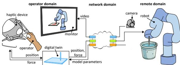
Figure 1: Overview of the whole environment. Our proposed solution for liquid simulation is located in the Operator Domain
