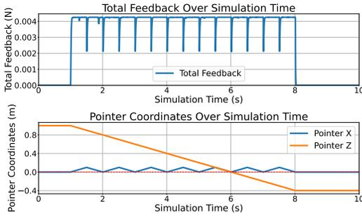
Figure 6: Body moves towards negative Z axis, alternating its direction in the X axis. Due to direction changes the tail cannot build up.
