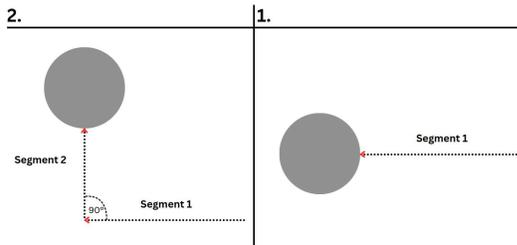
Figure 2: Movement of a body with a position tail in two steps. After a 90 degree turns, a new segment is created and the old one stays in place. Directions of each segment are highlighted in red.
