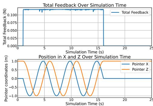
Figure 3: The body performs three perfect circles within a viscous liquid and is affected only by the drag equation.
