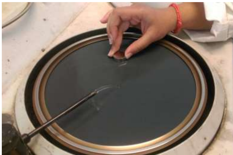
Figure 2.2. Ti6Al7Nb sample ground with SiC abrasive paper using water as a lubricant prior to PEO treatment.
