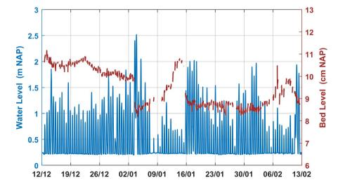
**FIGURE 6** The water level (blue) and the relative bed level (brown) from the start of the experiment until February 13. Two storm events with high water levels in January (3rd and 16th) caused sediment surface erosion. A calm period in between storms resulted in sediment accretion
