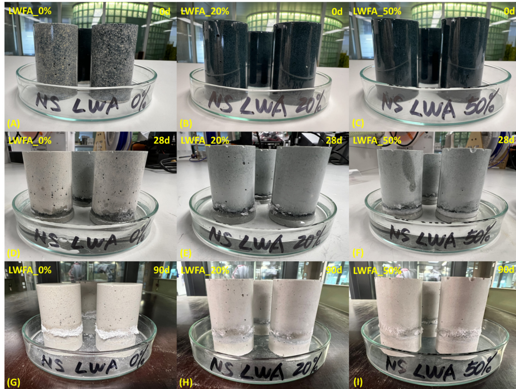
Figure C1. Visual observation of efflorescence of NS mortars with time.
