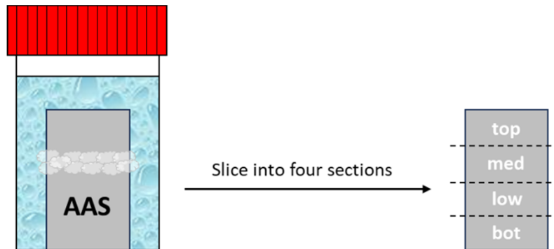
Figure 8.3. Sample preparation before paste characterisations. The 7 d sealed cylinders after 28 d of efflorescence under ambient conditions are first ultrasonically cleaned, and then are sliced into four sections, designated “bot”, “low”, “med” and “top”.
