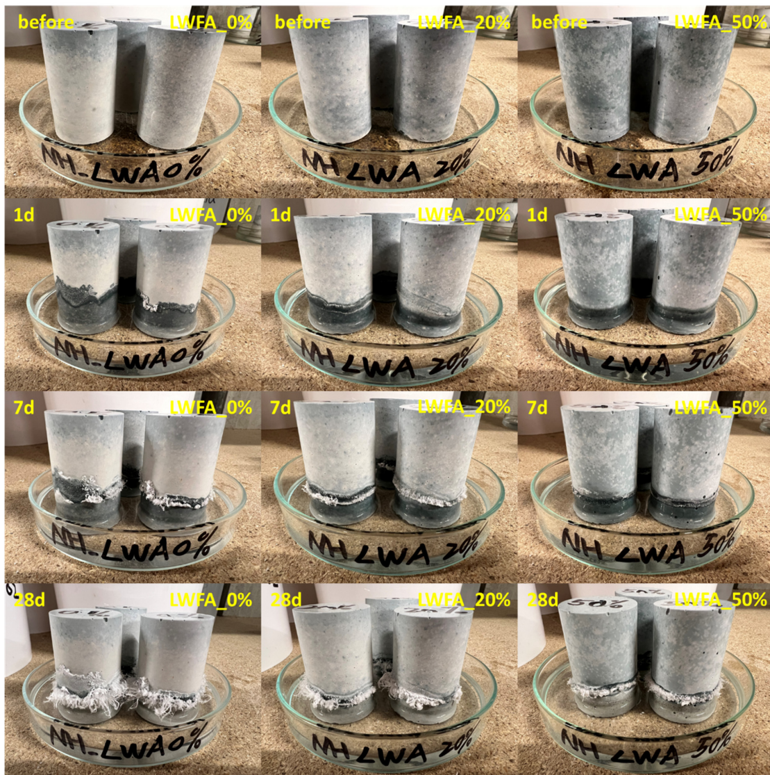
Figure 9.3. Visual observation of the efflorescence of AAS mortar cylinders with time.
