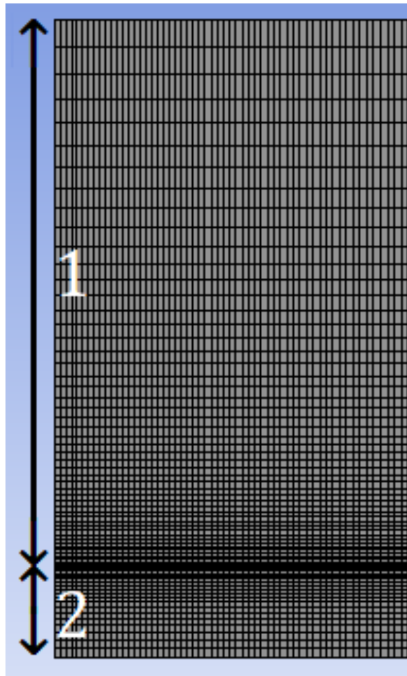
Figure 3.5: Inlet boundary conditions where 1 represents the free-stream inlet and 2 inlet condition that is the engine outlet
