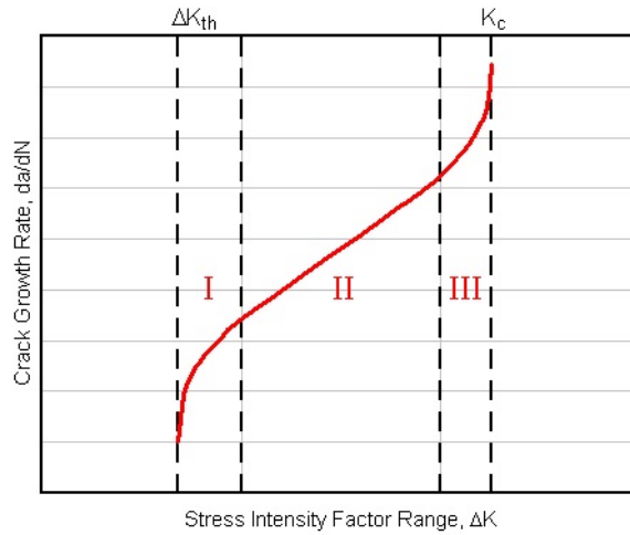
Figure 2.4: The three different crack growth regions on a log-log scale plot.
