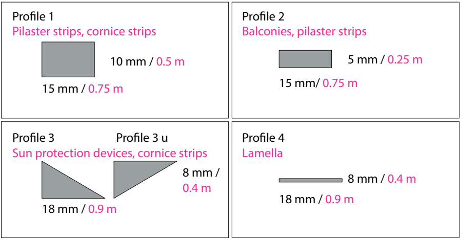
FIGURE 5.6 Section of profile rods used for building the detachable façade models.
