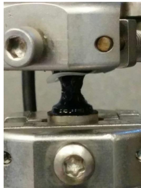
15 FIGURE 5 a. Specimen Fixed in Bottom Clamp in DSR b. Specimen After Testing at 10°C.
