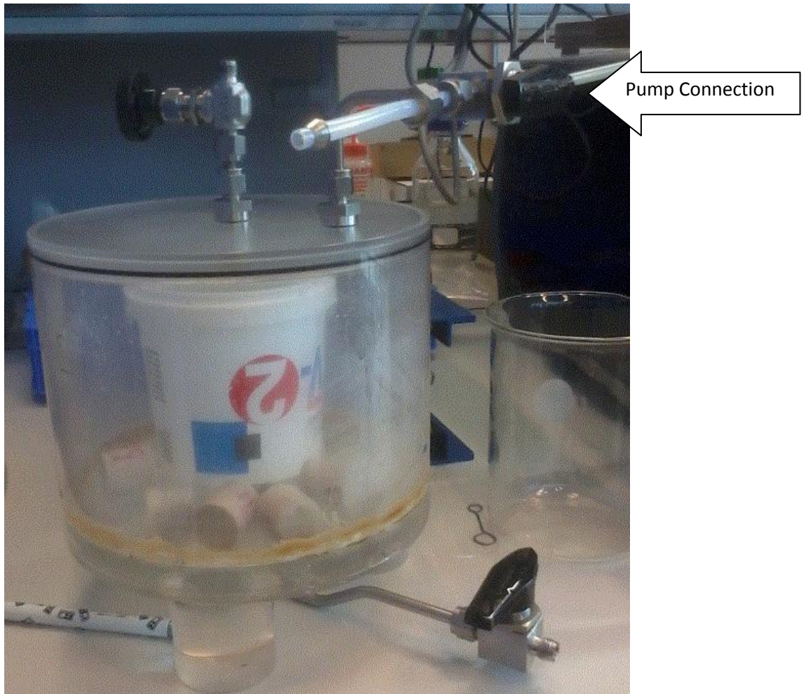
Figure-15: Wet test alignment, based on submersed samples to determine porosity
