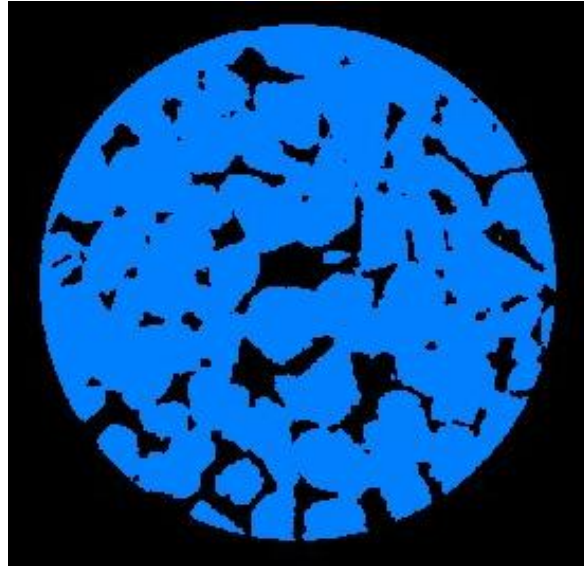
Figure-38: Binary of silica grains of 'no' carbonate deposition (blue)
