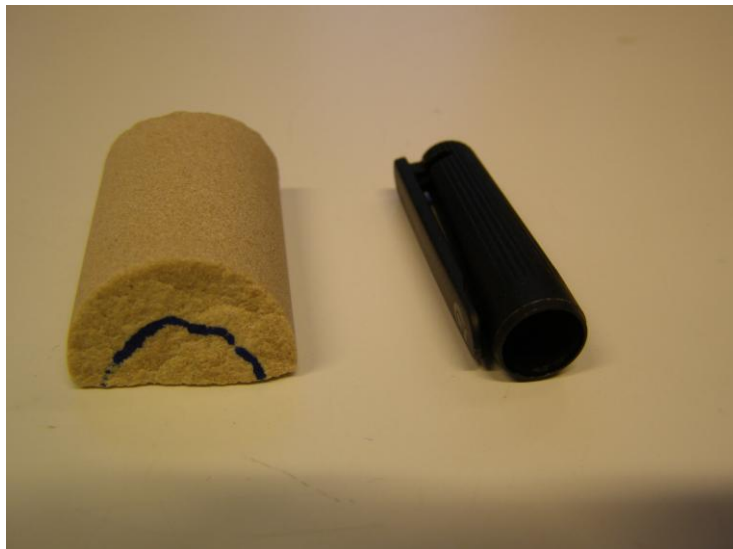
Figure-45: Fractured sample; blue line indicates fracture plane
