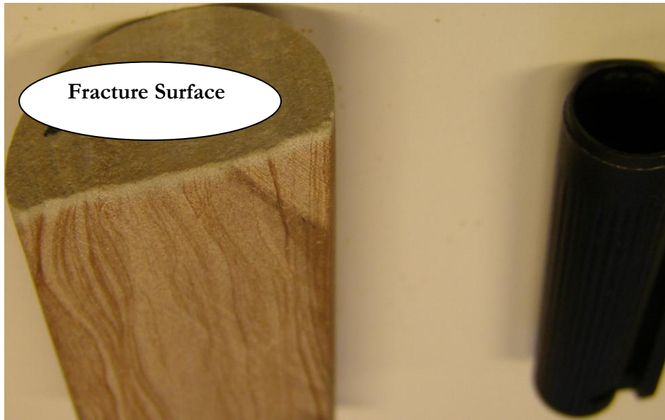
Figure-74: Carmel (CAR-614-FR) sample with fracture plane
