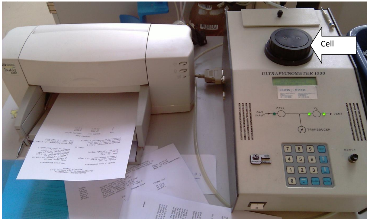
Figure-14: Ultra Pycnometer 1000, used to determine porosity
