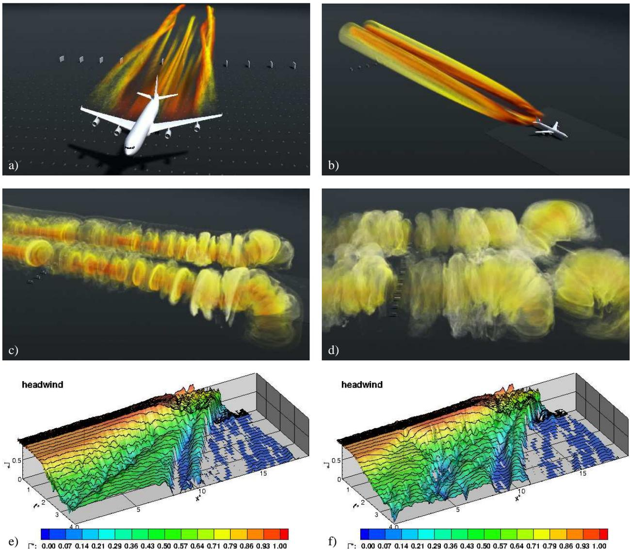
**Figure 1.** Hybrid LES of landing, a),b) initial wake, c) ground effect with vortex bursting, d) plate line effect aground linking. Normalized vortex circulation development for the entire upwind vortex, headwind case, without plate line e), plate line f).
