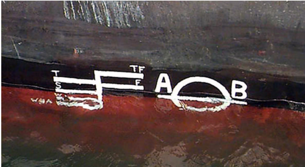
Figure 2.3: Plimsoll mark on a floating vessel's hull [Oceanservice, 2020]
