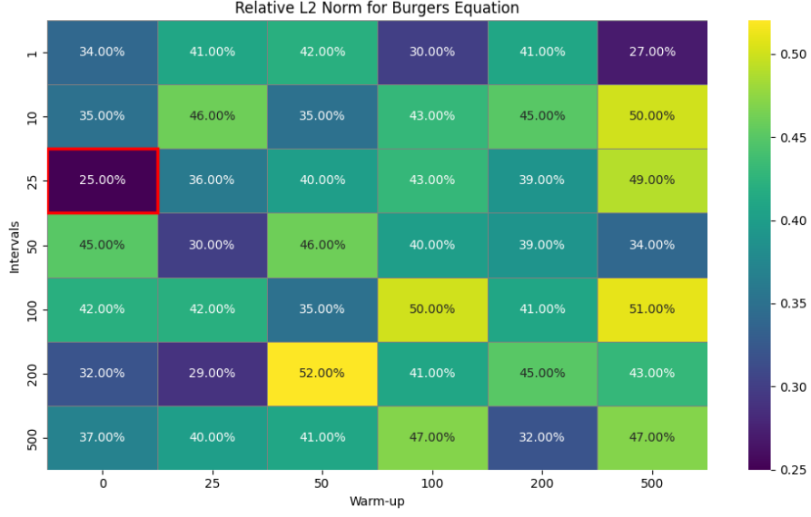
Figure 8: Relative L^2 norm for the 1D Burgers’ equation for different combinations of warm-up W and propagation periods I . Results were obtained using warm-up \gamma = 1e^{-5} , P = 5 , and N_{res} = 1,000 with Gaussian resampling ( \sigma^2 = 0.75 ).
