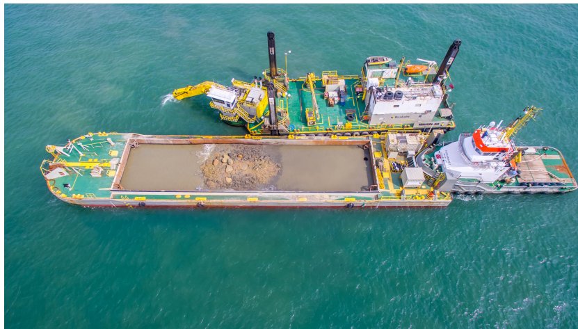
Figure 4.4: Manu Pekka and transporter barge - Environmental dredging (Boskalis)
