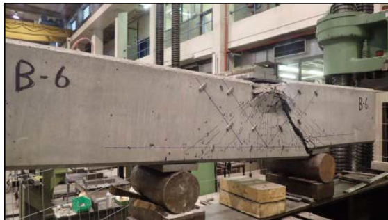
FIGURE 13 Beam B-6 after shear failure
