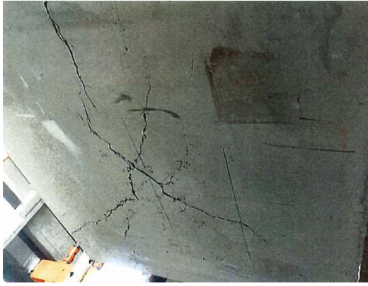
FIGURE 21 Crack pattern at bottom of slab P-3 (with fibers and ties) after the test
