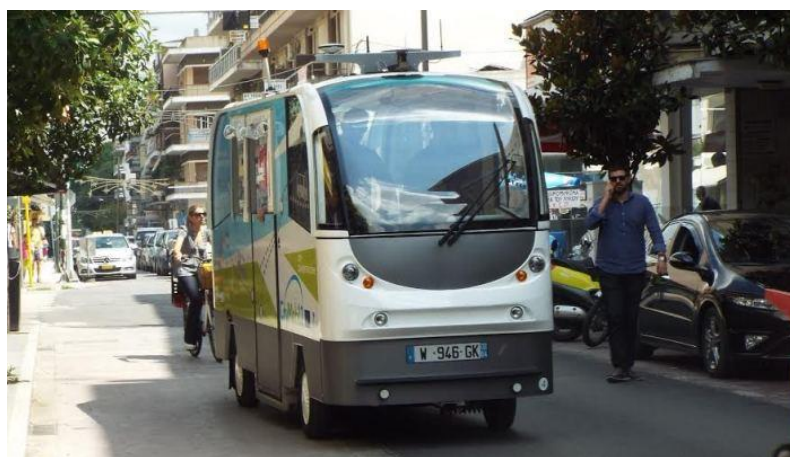
Figure 2. Automated shuttle by Robosoft on a public road in a mixed traffic situation in Trikala, Greece
