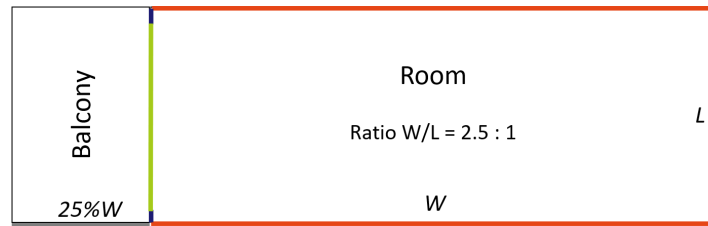
Figure A.8: Definition of lengths of inner and outer walls as well as windows in early design stage for standardized cabin
