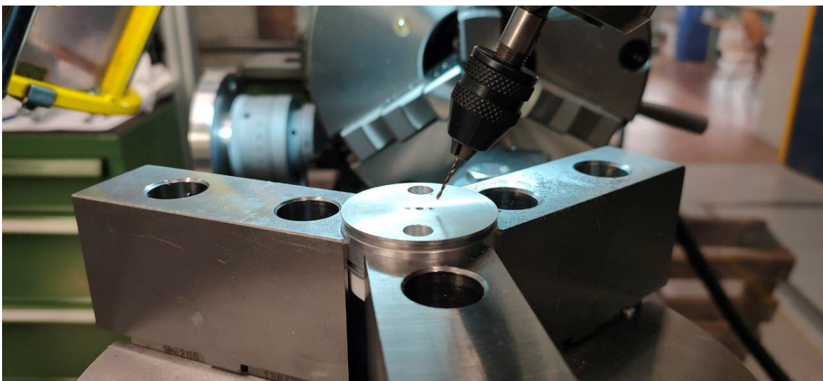
Figure B.1: Close up of the clamping of the manifold and alignment of the diagonal injection hole.
