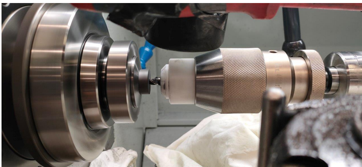
Figure B.6: Machining of nozzle divergent using a conical mill and custom hard stop.
