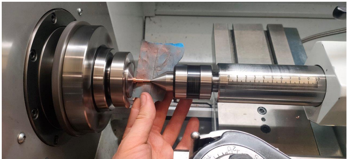
Figure B.4: Sanding of the edges on a HV connector as it is clamped in a collet and suspended in a rotating center
