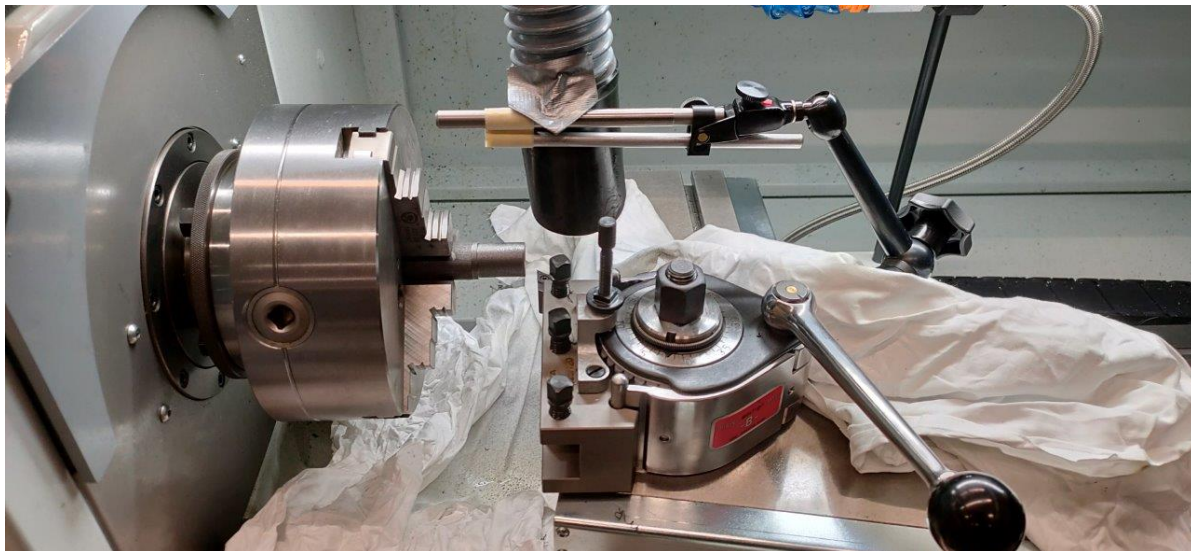
Figure B.5: Graphite dust collection setup on a lathe
