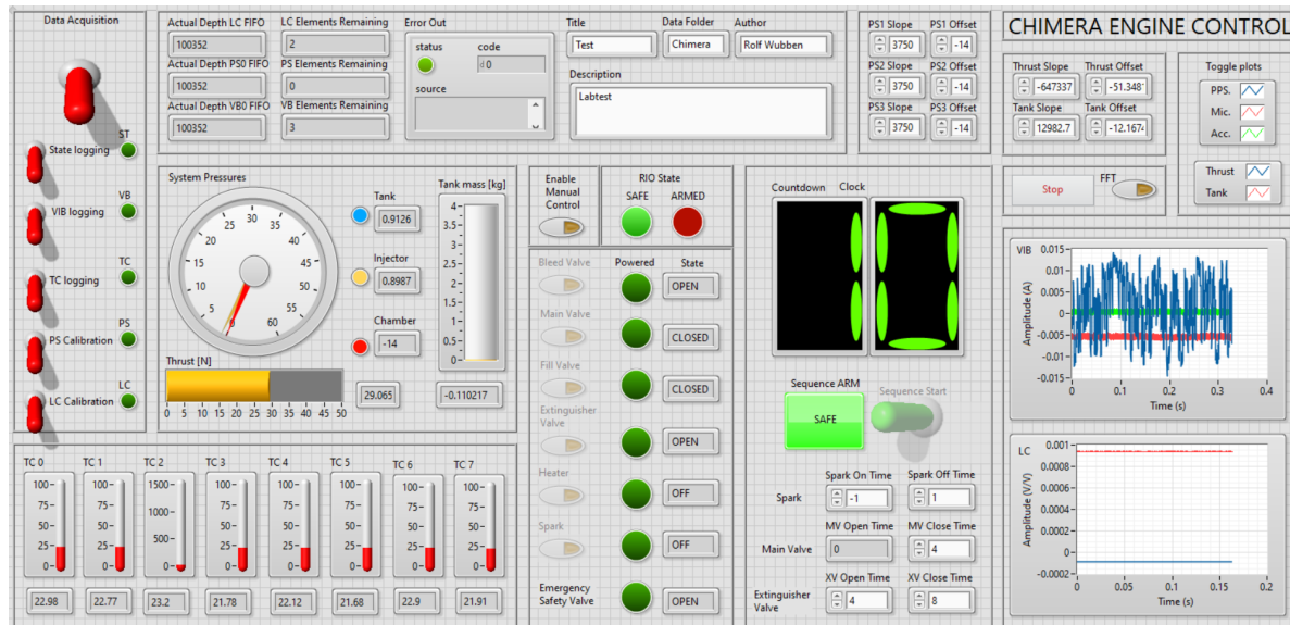
Figure 6.21: GUI used to control the hybrid engine test setup and log data
