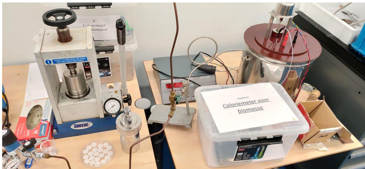
Figure 4.14: Bomb calorimetry test setup. Note the press to assemble benzoic acid discs for calibration purposes. On the right, the bomb water bath with brown top can be seen.
