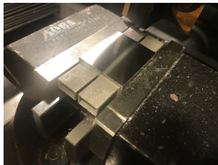
(c) Milling process, where the top layer of the print is removed.
