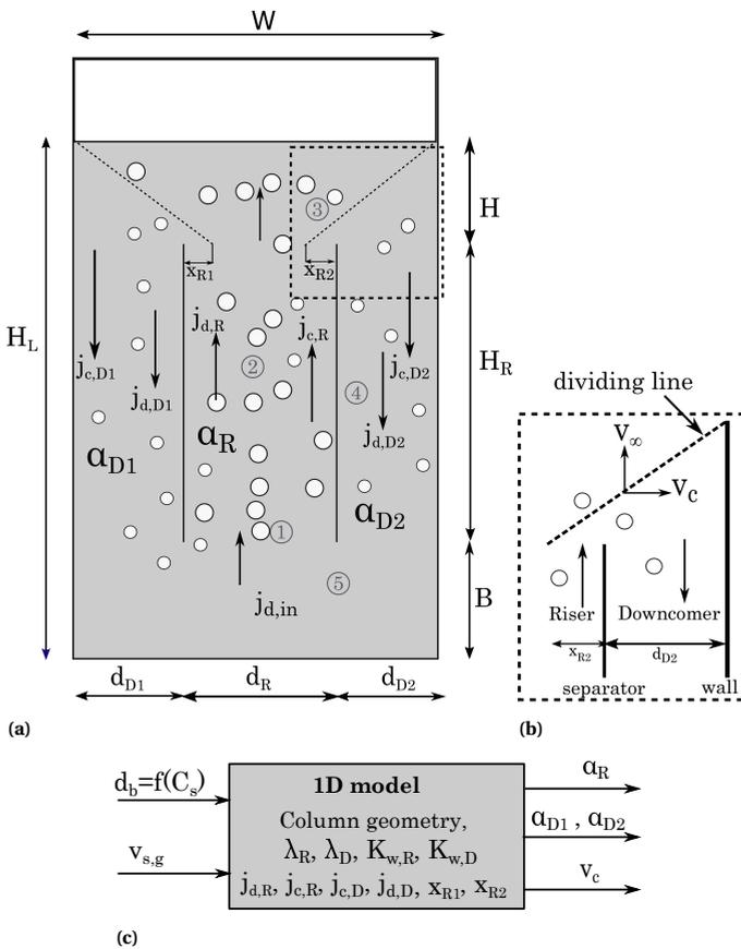
**Figure 2.11:** (a) Schematic of the drift flux model with different zones marked: 1-Sparger section, 2-Riser (above sparger plate), 3-disengagement zone, 4-downcomer section, 5-bottom gas recirculation (b) Modelling of gas-carryover into downcomer section (c) Variables involved in the 1D model (see appendix for equations).
