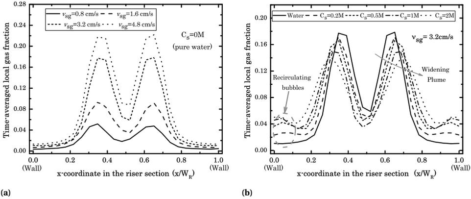
**Figure 2.8:** Gas fraction profile in riser section (measured above the sparger plate, 250 mm from the bottom of the column): (a) Effect of gas flowrate without salt; (b) Effect of salt addition with gas superficial velocity,  $v_{sg} = 3.2\text{ cm/s}$ . Same measurement locations have been used to compare pure water and salt cases.
