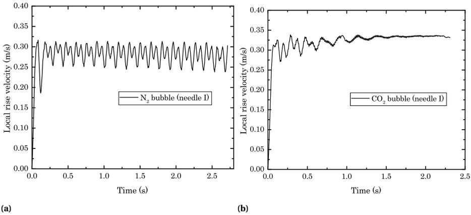
**Figure 4.8:** Time evolution of the local bubble rise velocity of (a)  $N_2$  and (b)  $CO_2$  bubbles generated from a 0.2 mm orifice (Needle I). Due to a higher velocity of the  $CO_2$  bubble, it can be tracked for a shorter time than the  $N_2$  one. Local fluctuations in velocity due to pixel-error in the detection of the bubble centroid is 0.003 m/s ( $\pm 1\%$ ).
