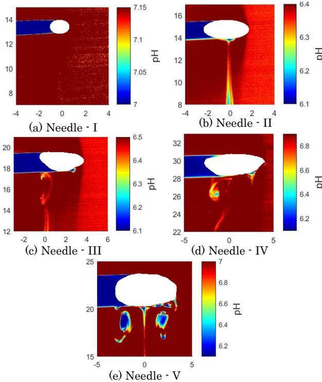
**Figure 4.10:** P-LIF results (a-e): pH profiles showing the  $\text{CO}_2$  distribution in wake of bubbles generated from different needles I-V. Spatial units are in mm and the colour corresponds to the pH value. The bubble location is approximately four bubble equivalent diameters from the tip of the needle (0,0). The location of the bubble is cut out (may not be exact size), to not distract the reader by illogical values obtained due to reflections (Figure 4.4b).
