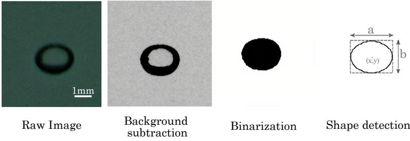
**Figure 3.3:** Image processing steps in FIJI software
