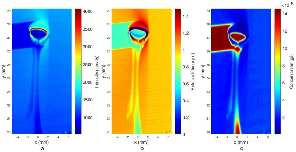
**Figure 4.21:** LIF processing steps: (a) Raw Image (b) Relative intensity image (c)  $\text{CO}_2$  concentration image. Note that there is an extra step between (b) and (c), going from relative intensity to pH.
