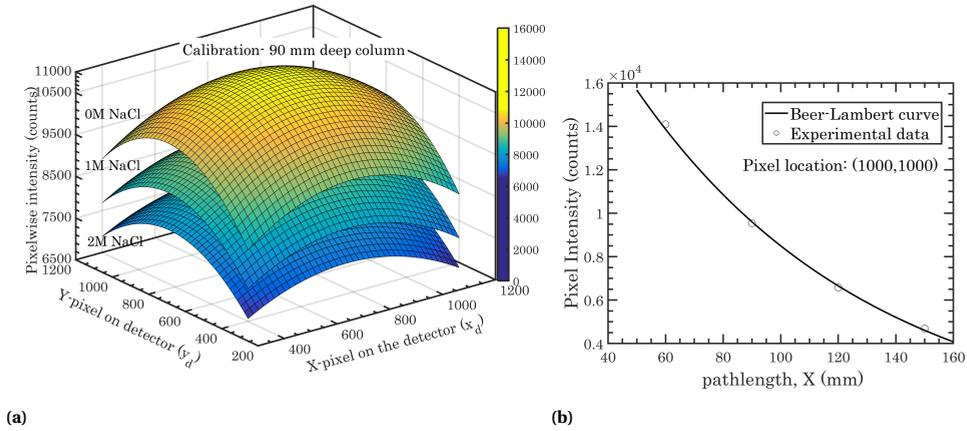
**Figure 2.3:** Pixel-wise calibration of intensity: (a) cone-beam calibration profile for 90 mm deep column for different salt concentrations; (b) comparison of interpolated Beer-Lambert curve with experimental data on a random pixel  $(x,y) = (1000,1000)$  on the detector.
