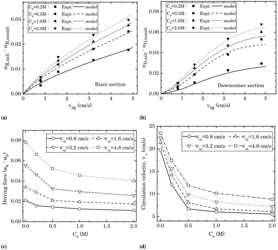
**Figure 2.12:** (a & b) Comparison of the experimental results with the 1D model: gas fraction increase due to salt addition in (a) riser section ( $\alpha_{R,salt} - \alpha_{R,nosalt}$ ); (b) downcomer section ( $\alpha_{D,salt} - \alpha_{D,nosalt}$ ) (c) Overall driving force for recirculation  $\alpha_R - \alpha_D$  (experimental data from X-ray imaging) (d) Liquid recirculation velocity (from 1D model). The input for the model for various salt concentrations is  $d_{b,avg} = f(C_s)$ .
