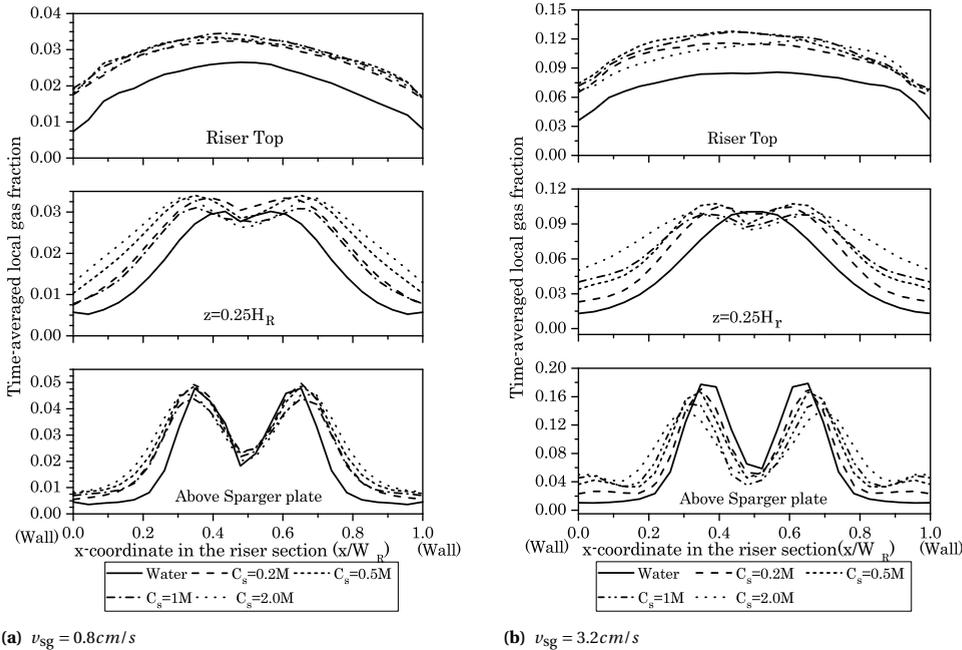
**Figure 2.9:** Gas fraction in the riser section for (a)  $v_{sg} = 0.8\text{ cm/s}$  and (b)  $v_{sg} = 3.2\text{ cm/s}$ . Measurement locations: distance from bottom of the column ( $z$ ), Above sparger plate:  $z = 250\text{ mm}$ ;  $H_R/4$ ;  $z = 340\text{ mm}$ ; Riser top:  $580\text{ mm}$ .
