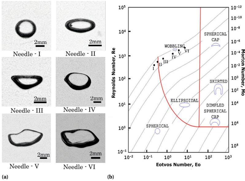
**Figure 4.5:** (a) Typical shapes of N<sub>2</sub> bubbles produced from needles I-VI. (b) Non-dimensional shape regime map with data from Clift *et al.* [9] (Background image reproduced from Amaya-Bower and Lee [32])
