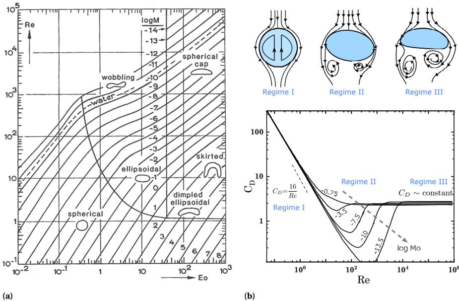
**Figure 1.2:** (a) Clift-Grace-Weber map (adapted from [14]) showing the various regimes in bubble motion in  $Re$ - $Eo$ - $Mo$ . (b) Drag coefficient prediction for a variety of bubbles (adapted from [17]) with a schematic representation of bubble wakes.
