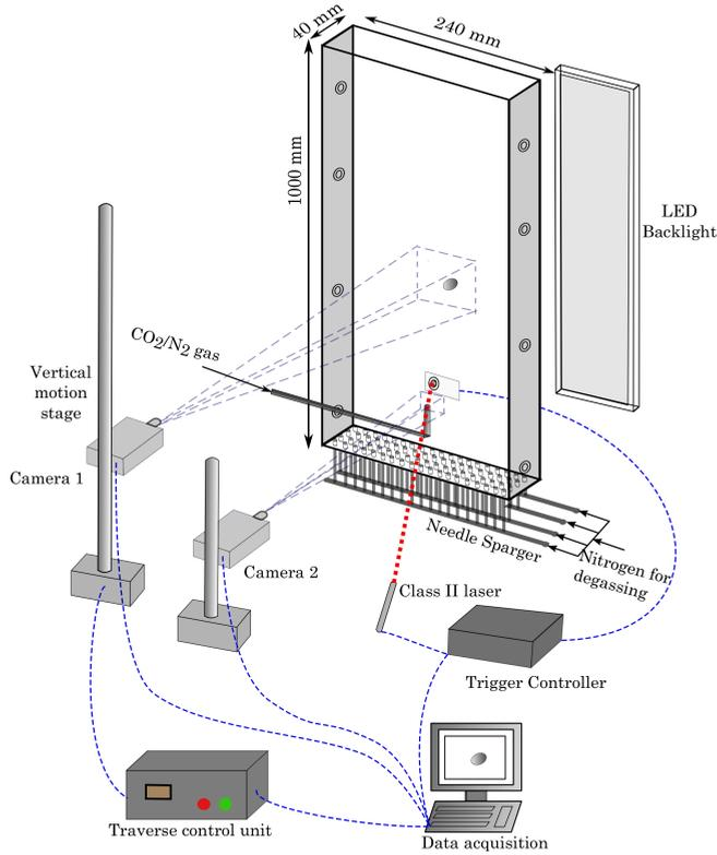
**Figure 4.2:** Schematic of the moving camera setup
