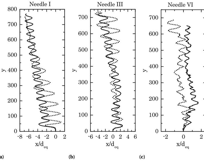
**Figure 4.12:** Bubble trajectories for  $N_2$  (—) and  $CO_2$  (·····) bubbles generated with three different needle sizes: (a) 0.2 mm Needle I (b) 1.0 mm Needle III, and (c) 4.5 mm Needle VI. Three cases chosen here are indicative of three regimes of bubble shapes. Note the relative sizing of the x- and y-axes.
