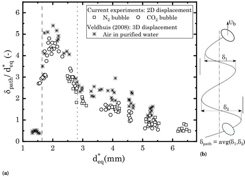
**Figure 4.13:** (a) Non-dimensional displacement in bubble path ( $\delta_{path}/d_{eq}^*$ ) for  $N_2$  and  $CO_2$  bubbles in helical regime. The two vertical lines indicate the onset of path (left: - - - -) and shape oscillations (right: ·····). Note that the data from Veldhuis [40], based on 3D visualization, is the maximum horizontal displacement obtained from the reconstructed top-view. (b) Schematic of the bubble path.
