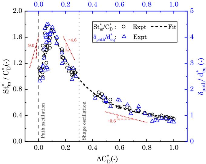
**Figure 4.18:** Ratio of mass transfer- momentum coefficients,  $k_L/h_u$  (represented as  $St_m/C_D$ ) and Non-dimensional bubble path ( $\delta_{path}/d_{eq}$ ) as a function of measured drag coefficient ( $C_D$ ) for  $CO_2$  bubbles. Different measurement points correspond to local bubble data, as described earlier in Figure 4.13a.
