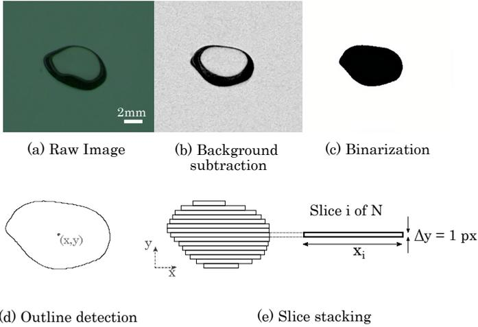
**Figure 4.3:** Image processing steps in FIJI software
