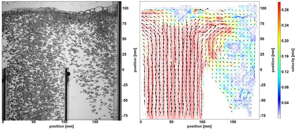
(a) Water,  $v_{sg} = 1.6\text{ cm/s}$
