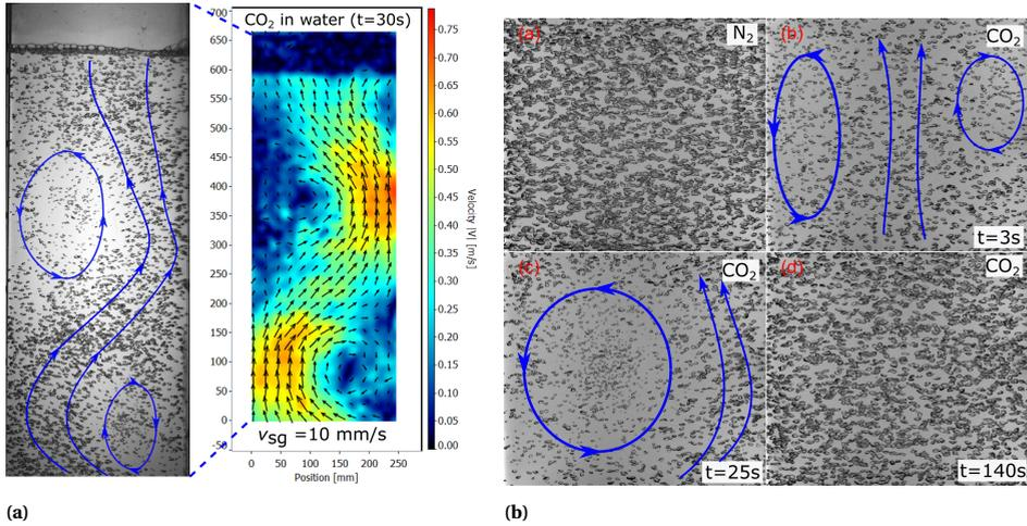
**Figure A.3:** CO<sub>2</sub> bubbles in water at  $v_{sg}=10$  mm/s: (a) Flow profile (blue markings indicating motion of plume and the circulation cells) and bubble velocity profile at  $t=30$  sec (b) Snapshots of bubble images (captured at 400 mm above sparger) comparing N<sub>2</sub> and CO<sub>2</sub> case (at  $t=3$  sec, 25 sec and 140sec). Times stated here are from the start of gas sparging.
