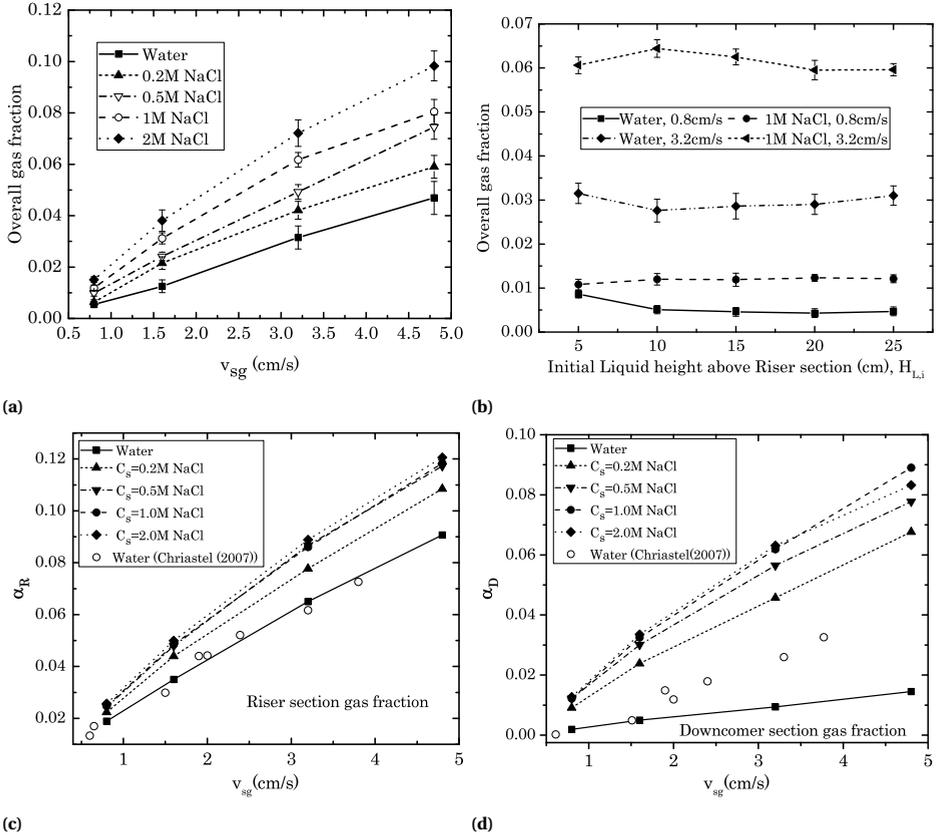
**Figure 2.10:** (a & b) Overall gas fraction as a function of: (a) superficial gas velocity,  $v_{sg}$ , for initial height  $H_{L,i} = 15$  cm; (b) Initial liquid height,  $H_{L,i}$ . (c & d) Section-wise averaged gas fraction (c) Riser section (data for salt concentrations,  $C_s = 0.5$  M, 1.0 M and 2.0 M are close to each other); (d) Downcomer section. Lines are for visual purposes and do not indicate a trend.
