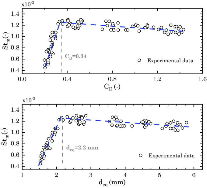
**Figure 4.17:**  $St_m$  as a function of the drag coefficient  $C_D$  and bubble equivalent diameter ( $d_{eq}$ ). Blue lines (---) added to indicate different regimes (do not reflect a correlation) with transition points at  $C_D = 0.34$ , corresponding to a bubble size,  $d_{eq} = 2.2$  mm.
