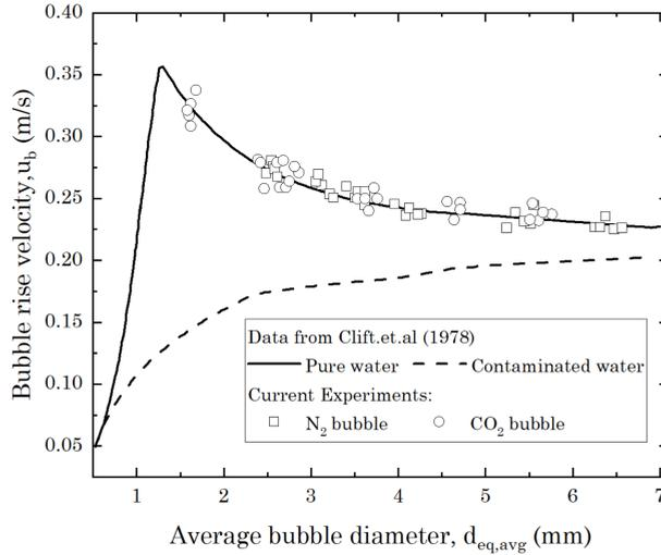
**Figure 4.7:** Average bubble rise velocity,  $u_b$  from current experiments, compared to the empirical data from Clift *et al.* [9, Figure 7.3] for pure and contaminated water.
