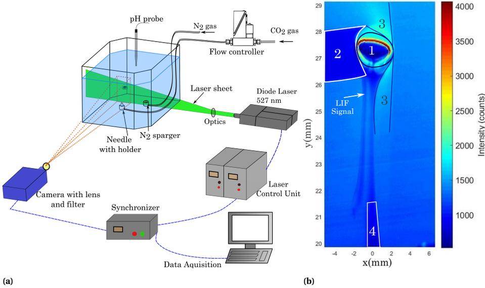
**Figure 4.4:** (a) Schematic of the Planar LIF setup. (b) Raw image from LIF acquisition with regions for interpretation: 1. bubble region, 2. shadow created by the bubble, 3. light cone (reflections of laser light hitting the bubble surface) and 4. region close to the needle, darker due to an accumulation of dissolved CO<sub>2</sub> during bubble generation.
