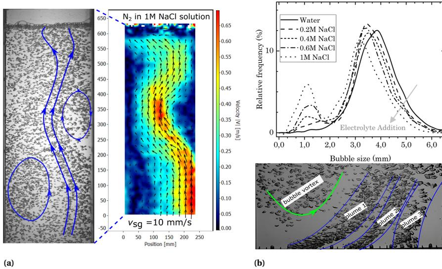
**Figure A.2:** (a)  $N_2$  bubbles in 1M NaCl solution at  $v_{sg}=10$  mm/s: Flow profile (blue markings indicating motion of plume and the circulation cells) and bubble velocity profile (b) top: Bubble size distribution as a function of electrolyte concentration at  $v_{sg}=10$  mm/s; Bottom: snapshot of bubble flow close to the sparger (contrast enhanced) showing interaction of bubble vortex and plume generation from the sparger.
