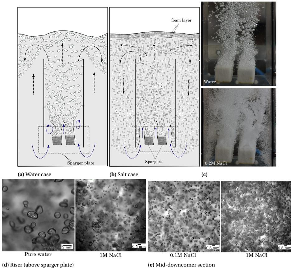
**Figure 2.7:** Schematic of flow patterns: (a) Water case (b) Salt case ; (c) Snapshots of the sparger region at  $v_{sg} = 1.6\text{cm/s}$ , top: Water, bottom: 0.2M NaCl ; (d & e) High speed images of the bubbles at  $v_{sg} = 1.6\text{cm/s}$  (field of view: 17 mm x 17 mm): (d) riser section (above the sparger plate) (e) mid-downcomer section.
