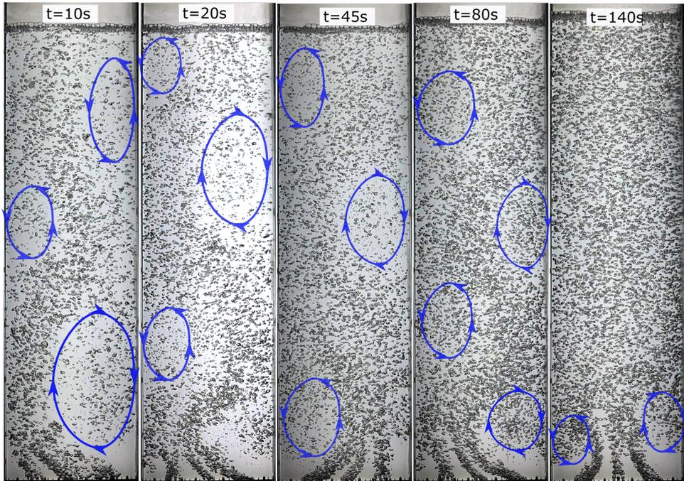
**Figure A.4:** CO<sub>2</sub> bubbles in water at  $v_{sg}=10$  mm/s: Instantaneous flow snapshots at different times during the absorption process (blue markings indicate the circulation cells).
