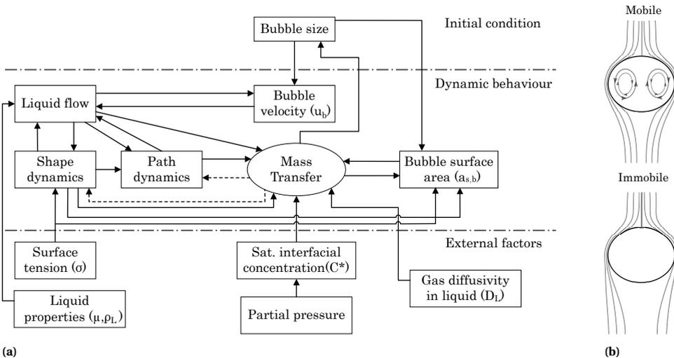
**Figure 4.1:** (a) Interrelations between parameters involved in gas-liquid mass transfer from a single bubble rising in a pure liquid. A dashed line (-----) indicates a weaker influence. (b) Schematic of flow around (top) mobile and (bottom) immobile interface.
