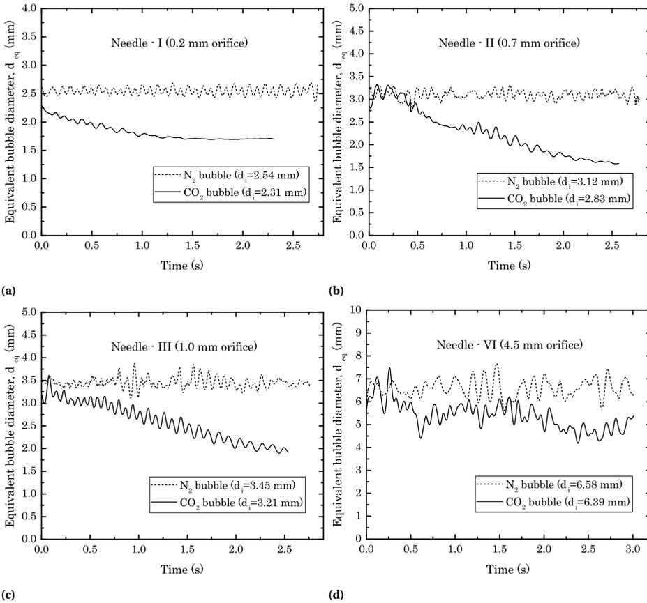
**Figure 4.6:** Time evolution of the bubble equivalent diameters of  $N_2$  and  $CO_2$  bubbles for four different needle cases: (a) Needle I (b) Needle II (c) Needle III (d) Needle IV.  $d_i$  is the initial bubble size obtained from processing images from camera 2
