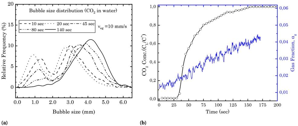
**Figure A.5:** CO<sub>2</sub> bubbles in water at  $v_{sg}=10$  mm/s: (a) Bubble size distribution at different times (as indicated in Figure A.4). (b) Instantaneous CO<sub>2</sub> concentration (measured using a pH probe), normalized with equilibrium concentration  $C^*$  and gas fraction (measured using Digital image analysis). Times stated here are from the start of gas sparging.
