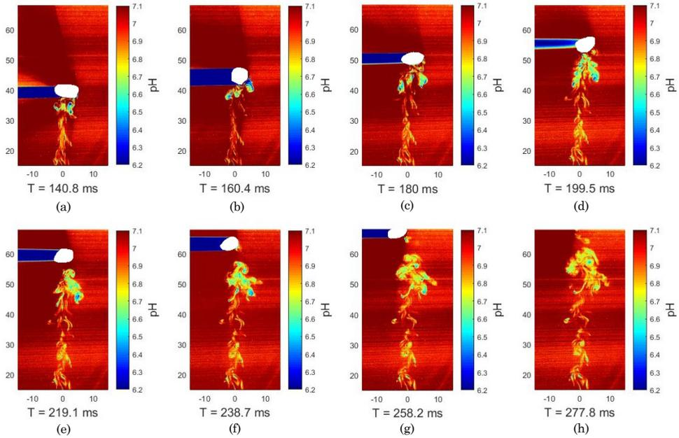
**Figure 4.11:** (a-h) Time evolution of the wake behind a bubble in the zig-zag regime, generated by a needle IV (with inner diameter = 2.2 mm), corresponding to a bubble size,  $d_{eq} \sim 3.7$  mm. The time indicated begins at detachment of the bubble at the needle.
