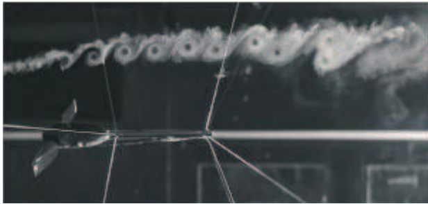
(a) Wind tunnel smoke visualisation showing tip vortex spiral interaction. Source: Alfredsson and Dahlberg [13]
