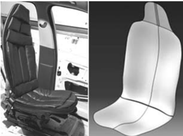
Figure 4.1 New car-seat concept based on the human body contour developed at BMW (Franz et al., 2011).
