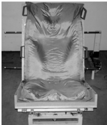
Figure 3.1 Frame with vacuum mattress after imprinting in the lab.
