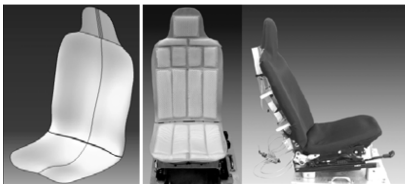
Figure 3.4 Seat shell in CAD software (left), inflatable cushions in the prototype of the light weight body contoured seat (middle), prototype of the light weight body contoured seat (right).
