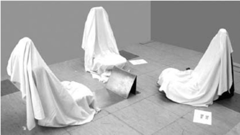
Figure 4.4 Research set-up with covered seats. The seats are deliberately covered so participants are not influenced by the appearance of the seats and focus on the seats' sitting comfort.
