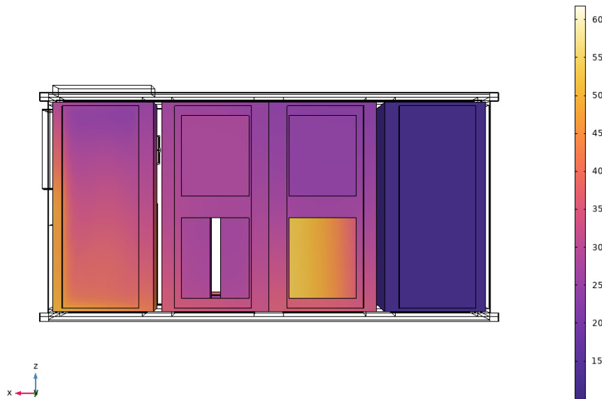
Figure 4.11: Final-design hot-case component temperature distribution at h_p = 130 km and \eta_{\text{pld}} = 20\% , reaching the +40 °C bus structure design target with the 10 °C margin to the 50 °C structure-to-payload interface requirement reserved for input dispersion. Component temperatures range from 21 to 57 °C: the cooler end corresponds to components on the self-shadowed side of the bus, and the warmer end to components near the body-mounted solar panel and front face, where internal dissipation in payload acquisition mode is superimposed on the structural gradient.
