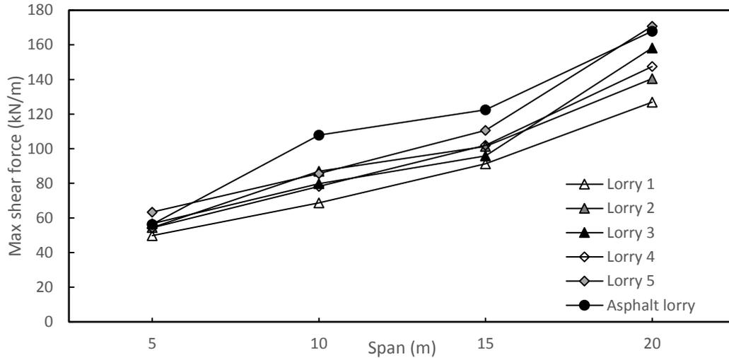
**Appendix Figure 8-5 - Shear force for an edge distance of 3m for different fatigue load models**
