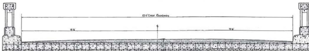
**Figure 3-1 - Example of the cross-section of a reinforced slab bridge (with edge beams)**
