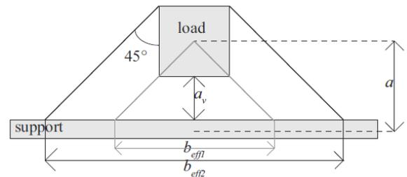
**Figure 4-3 - Horizontal load spreading (2 approaches) [34]**
