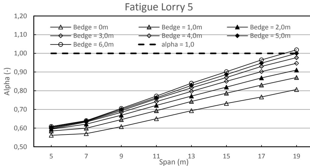
**Appendix Figure 9-4 - A factor (flexural moment) for the comparison of Load Model 1 and fatigue load model 5 for different spans and edge widths**
