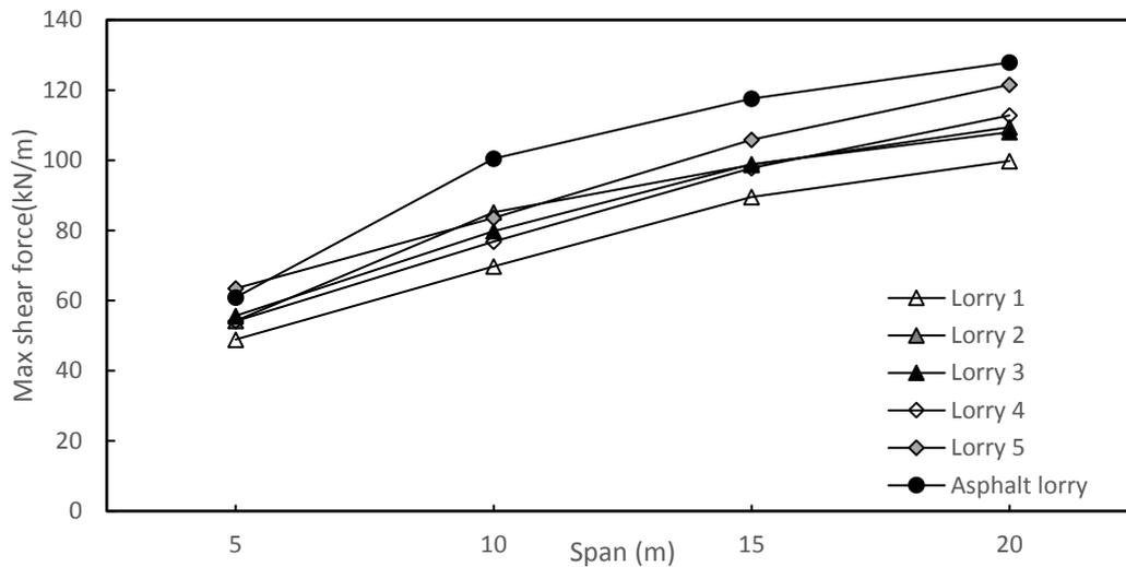
**Appendix Figure 8-6 - Shear force for an edge distance of 6m for different fatigue load models**
