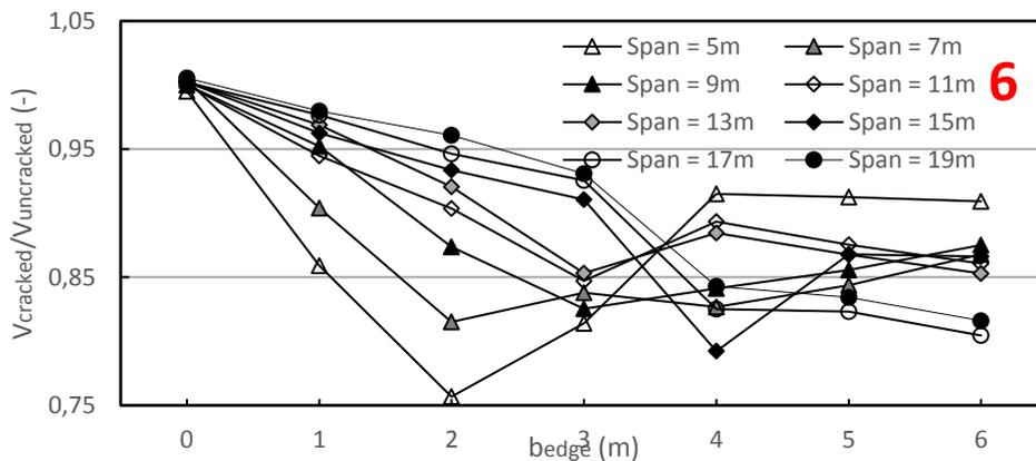
**Appendix Figure 10-7 - Comparison of shear force due to total loads near the edge of the support (cracked divided by uncracked)**
