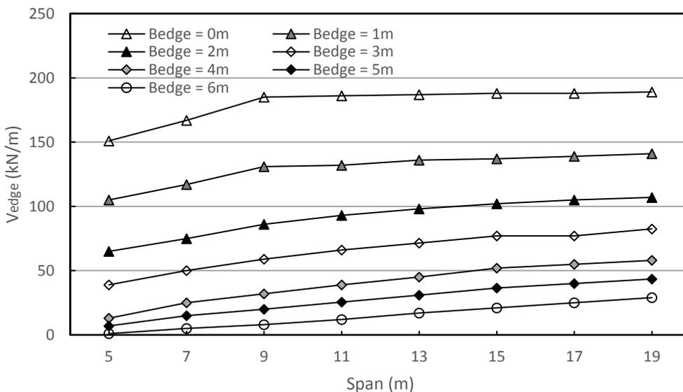
**Figure 7-9 – Shear force near the edge of the slab for an uncracked slab.**
