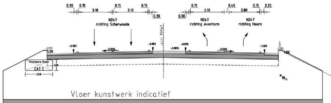
Figure 9-2 - Transverse cross-section at mid-span
