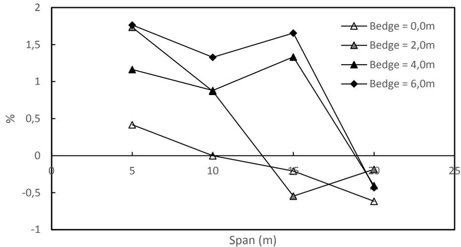
**Figure 7-11 - Difference of the occurring shear force by load configuration 1 (set at 0%) and 2**
