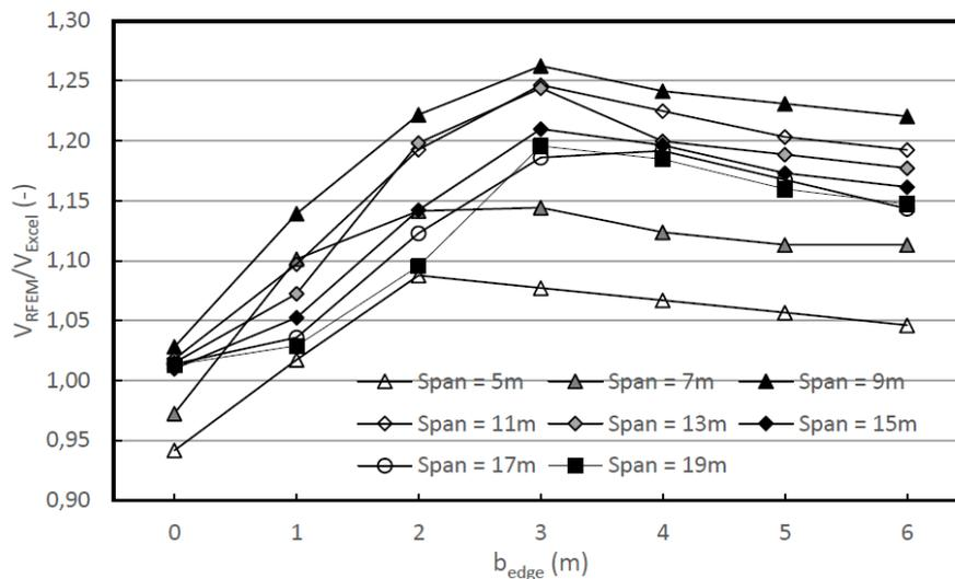
**Figure 8-6 - Difference between the occurring shear force near the middle of the slab according to RFEM divided by Excel (load transfer mechanism (b))**
