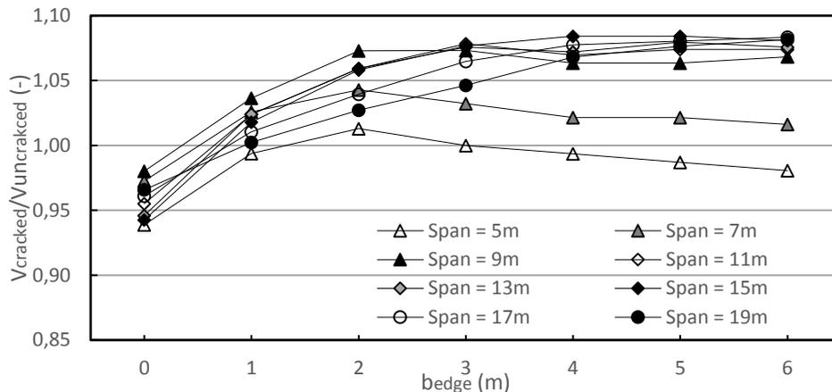
**Figure 7-4 - Comparison of shear force due total loads near the middle of the support (cracked divided by uncracked)**
