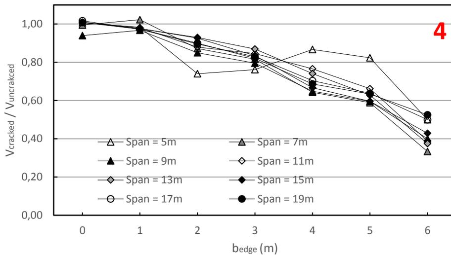
**Appendix Figure 10-5 - Comparison of shear force due to axle loads near the edge of the support (cracked divided by uncracked)**
