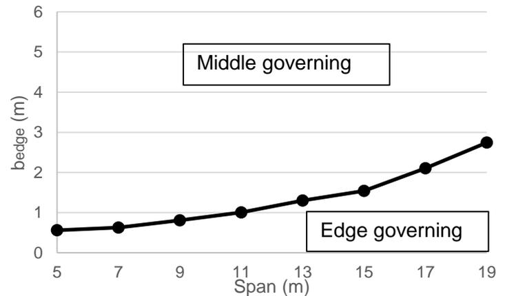
**Figure 7-16 - Graph for the determination of the governing part of the support (cracked prefab slab)**
