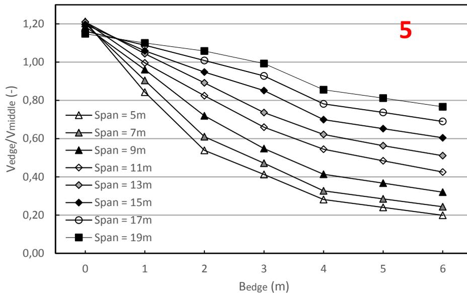
**Appendix Figure 10-12 - Comparison of shear force near the edge divided by the shear force near the middle of the support due to total loads (cracked slab)**
