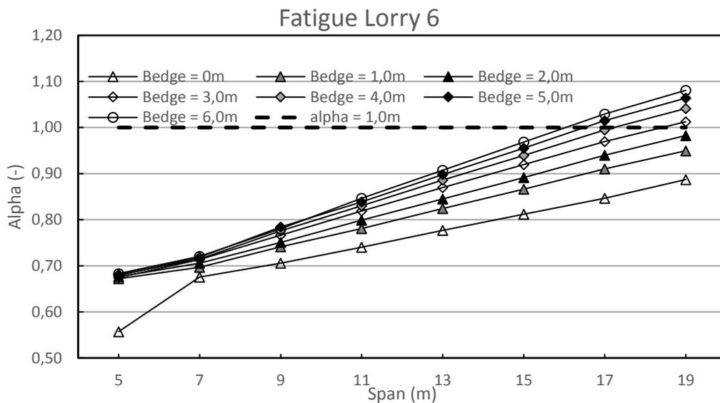
**Appendix Figure 9-5 - A factor (flexural moment) for the comparison of Load Model 1 and fatigue load model 6 for different spans and edge widths**
