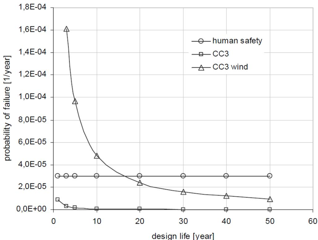
**Figure 3-13 - Annual failure probability as a function of the design working life for new structures (CC3) [23]**
