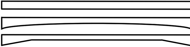
**Figure 3-2 - longitudinal cross-section slab bridge (constant, arched and inflected)**
