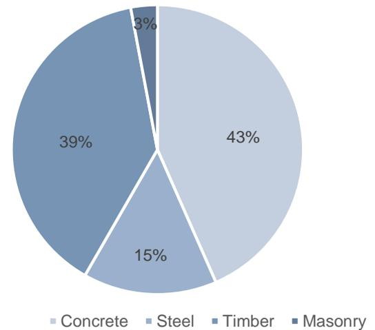
**Figure 2-4 - Average distribution of the building material of bridges per municipality**
