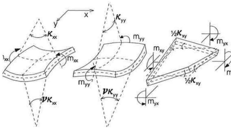
**Figure 5-3 - Due to transverse contraction a flexural moment leads to curvature in the transverse direction [44]**
