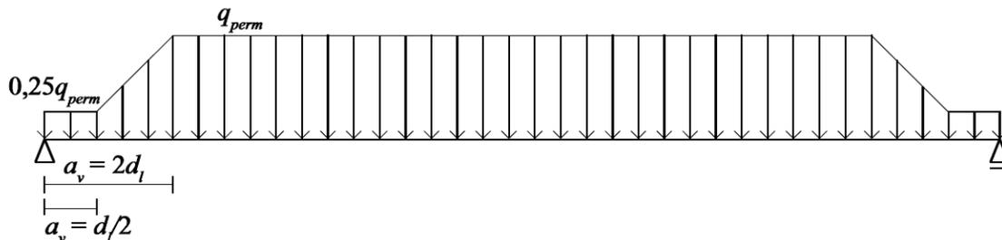
**Figure 7-6 - Resulting distributed load for permanent loads when  $\beta(x)$  is taken into account [33]**
