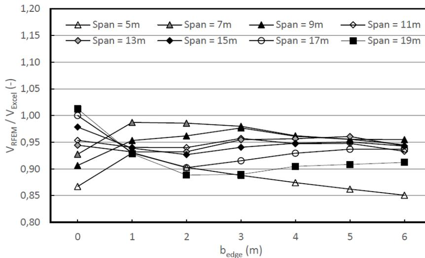
**Appendix Figure 14-2 - Comparison shear force RFEM and Excel near the middle of the support for cracked slabs**
