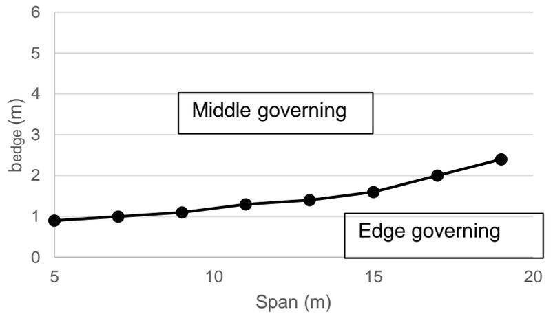
Figure 7-17 - Graph for the determination of the governing part of the support (uncracked in-situ slab)
