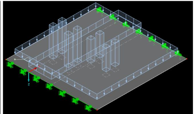
**Figure 7-1 - Example determining maximum shear stress near edge support.  $b_{edge} = 3m$ , Span = 12m**
