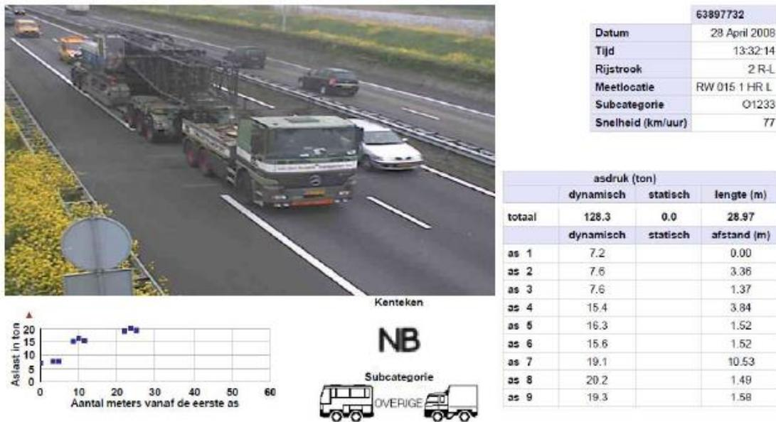
Figure 3-18 - Example of a long, heavy, special vehicle [27]
