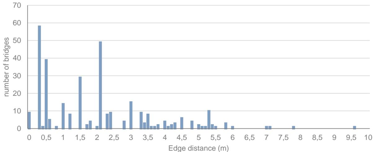
**Figure 2-6 – Edge distance ( $b_{edge}$ ) from the outer side of the carriageway to the edge of the deck (10 municipalities)**
