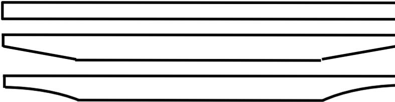
**Figure 3-3 - Transverse cross-section of a slab bridge (constant, decreasing thickness constant, decreasing thickness arched)**
