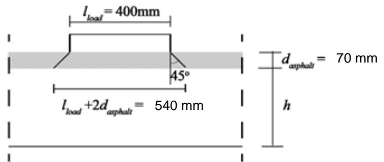
Figure 4-9 - Vertical load distribution of the wheel load through the wearing surface, adapted from [31]
