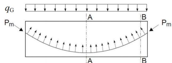
Figure 3-3 - Parabolic prestressing tendon profile [57]
