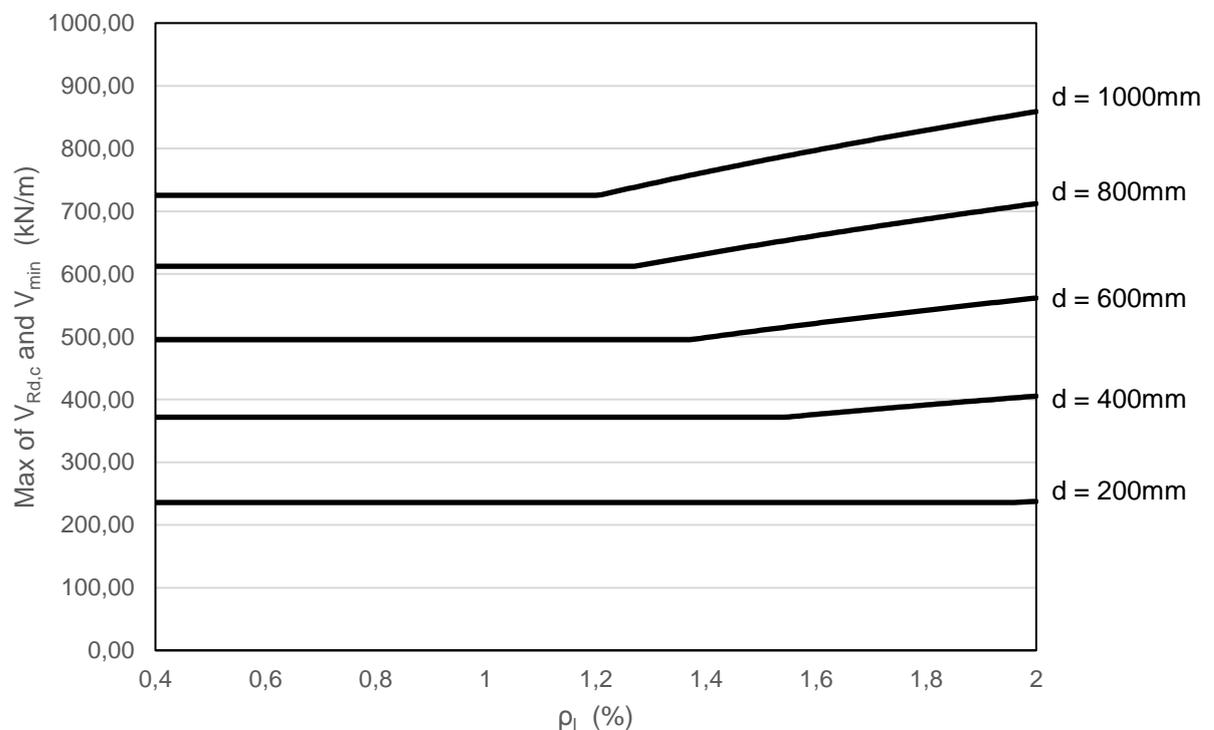
**Figure 8-16 - The maximum value of  $V_{Rd,c}$  or  $V_{min}$  for different effective depths and reinforcement ratios ( $f_{yk} = 240\text{ N/mm}^2$ )**
