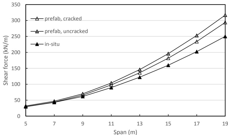
**Figure 7-7 – Shear forces due to self-weight for prefabricated (cracked and uncracked) and in-situ cast slabs for the edge of the support ( $b_{edge} = 6m$ )**
