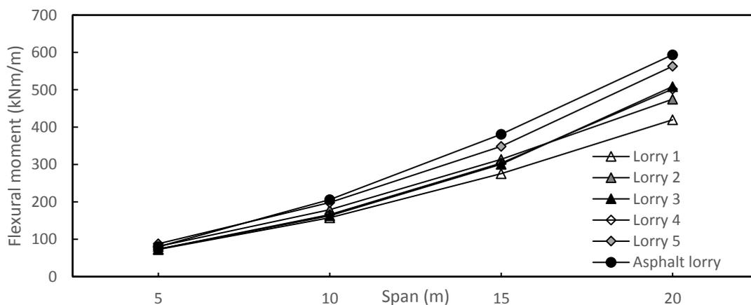
Appendix Figure 8-2 - Flexural moment for an edge distance of 3m for different fatigue load models
