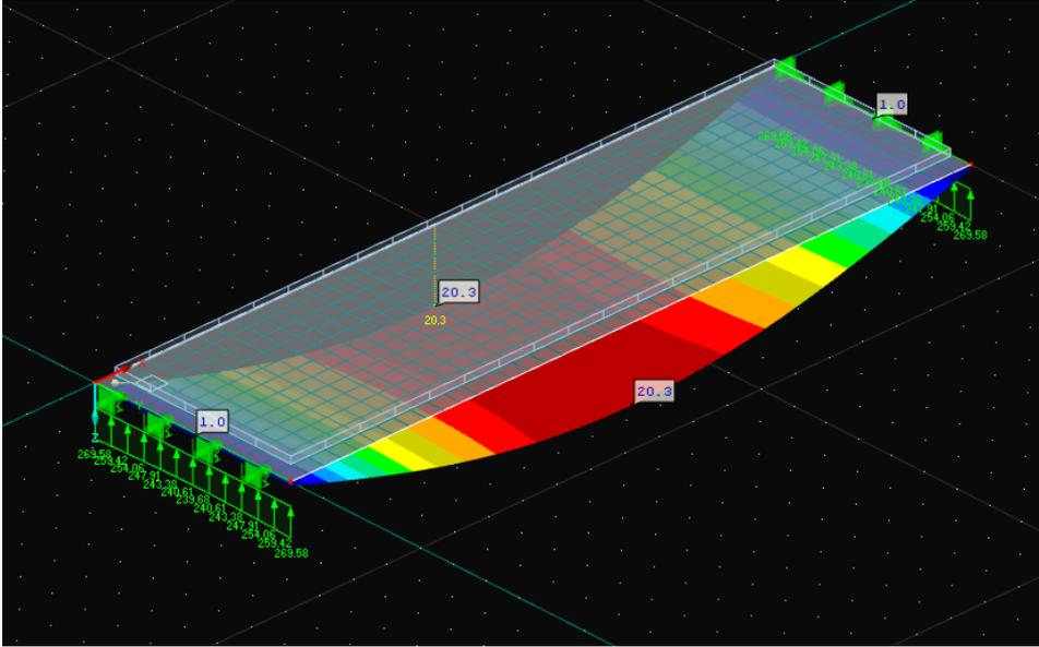
**Appendix Figure 7-4 - Deflection by self-weight, 1,0 mm at support, span: 20m**
