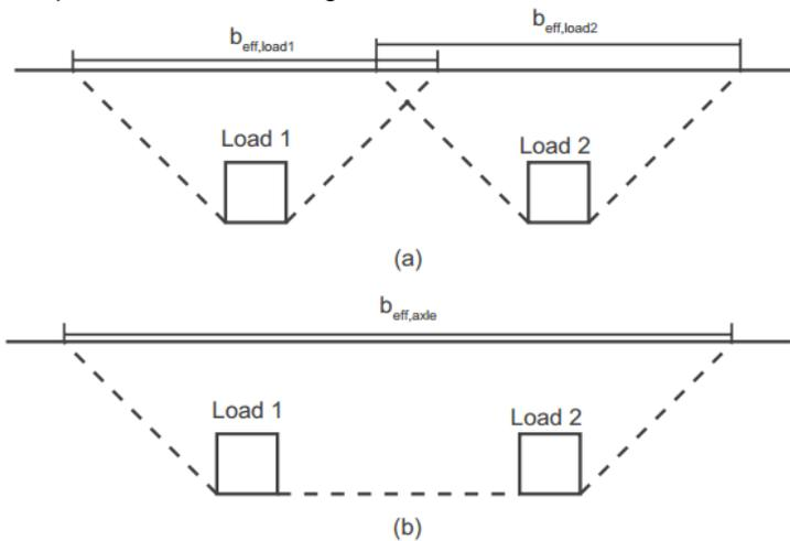
Figure 4-5 - a) effective width determined per wheel print. b) effective width determined per axle [34]
