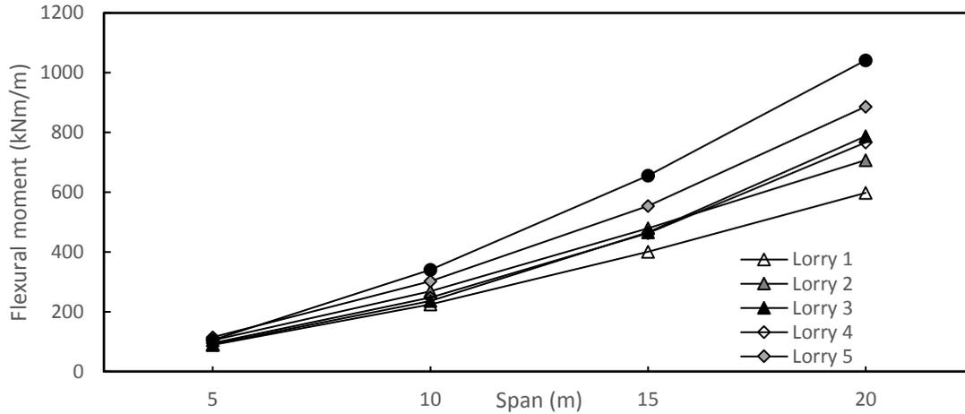
Appendix Figure 8-3 - Flexural moment for an edge distance of 6m for different fatigue load models
