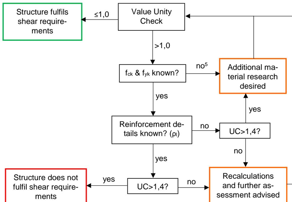
Figure 8-17 – Block diagram for the interpretation of the Unity Check
