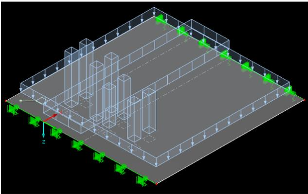
**Figure 7-2 - Example determining maximum shear stress near middle support.  $b_{edge} = 3m$ , Span = 12m**
