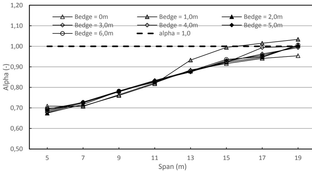
Appendix Figure 9-13 - A factor (Shear force) for the comparison of Load Model 1 and the Fatigue Lorry 6 for different spans and edge widths
