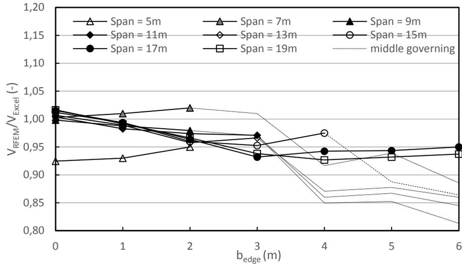
**Figure 8-11 – Comparison shear force RFEM and Excel near the edge of the support for uncracked slabs**
