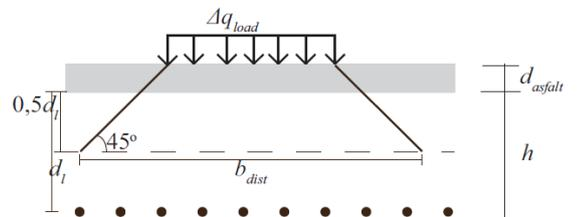
Figure 4-12 - Load spreading and contribution for the increased load on the first lane [31]
