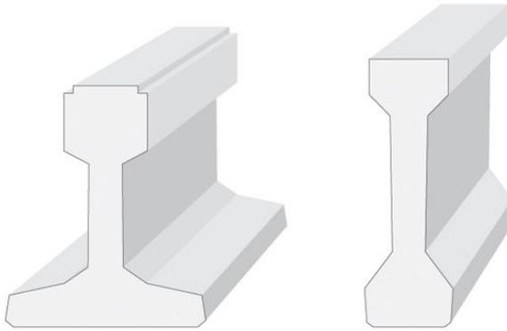
**Figure 3-5 - Example of an M-beam<sup>6</sup> (I-beam with wide bottom flange) and an I-beam (source: [http://www.scib.com.my/prestressed\\_beam.html](http://www.scib.com.my/prestressed_beam.html))**
