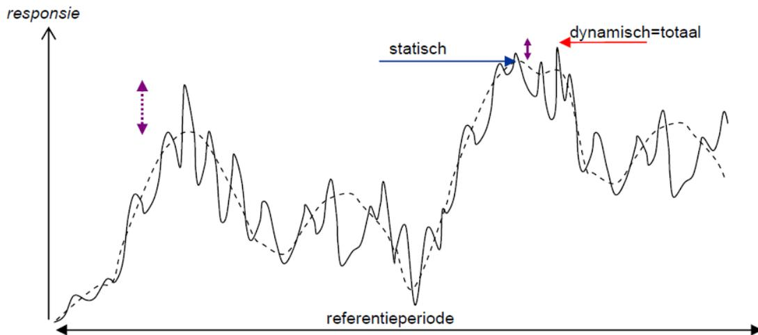
**Figure 5-13 - Definition dynamic amplification factor. Dashed line: static response. solid line: dynamic response [28]**
