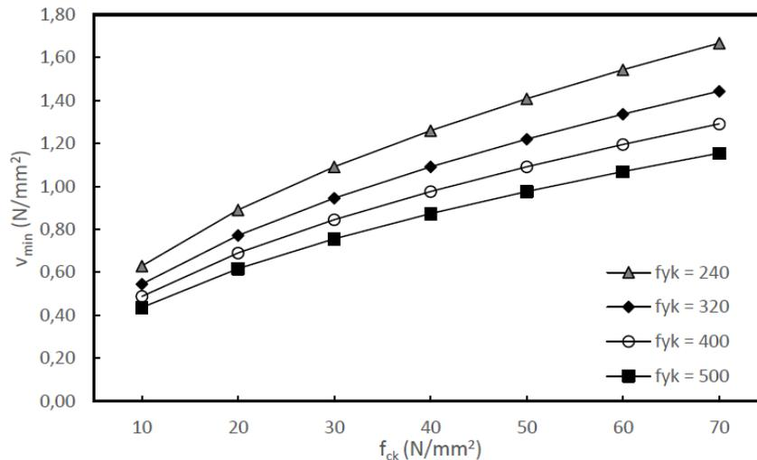
**Figure 8-8 -  $v_{min}$  for different values of  $f_{yk}$  and  $f_{ck}$**
