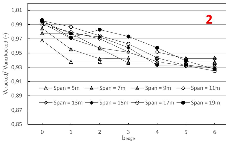
Appendix Figure 10-3 - Comparison of shear force due to self-weight near the edge of the support (cracked divided by uncracked)
