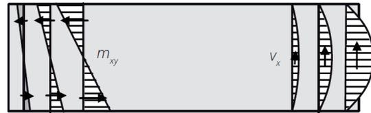
Figure 5-6 - Visualisation of the torsional moment and shear force in a thick strip [47]
