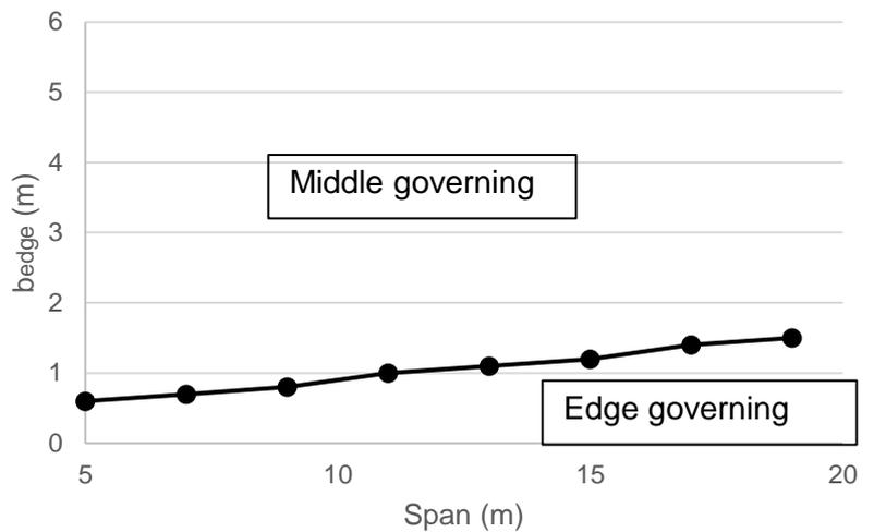
Figure 7-18 - Graph for the determination of the governing part of the support (cracked in-situ slab)
