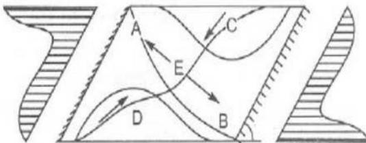
Figure 3-6 - Direction and magnitude of moment flow in skewed bridge decks [16]
