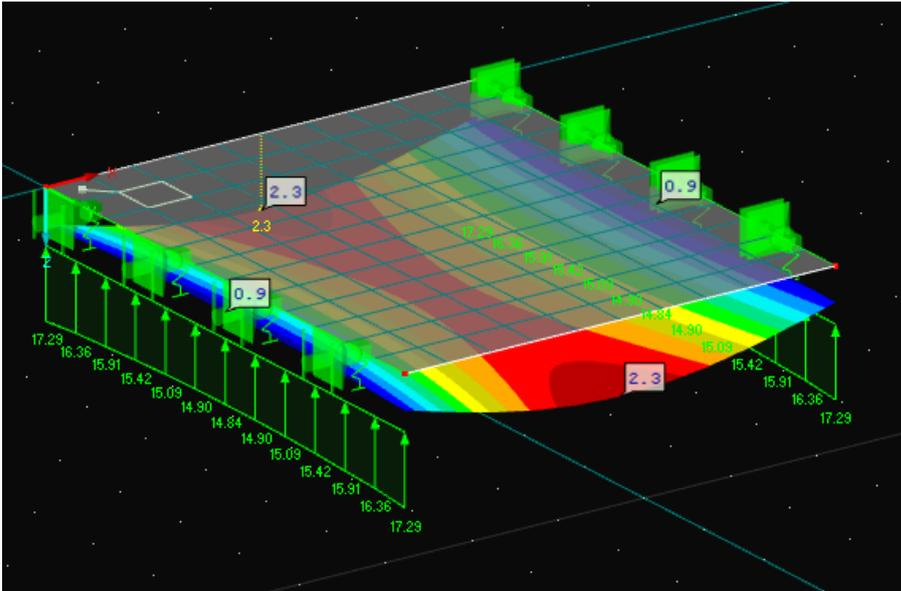
Appendix Figure 7-1 – Deflection by self-weight, 0,9mm at support, span: 5m
