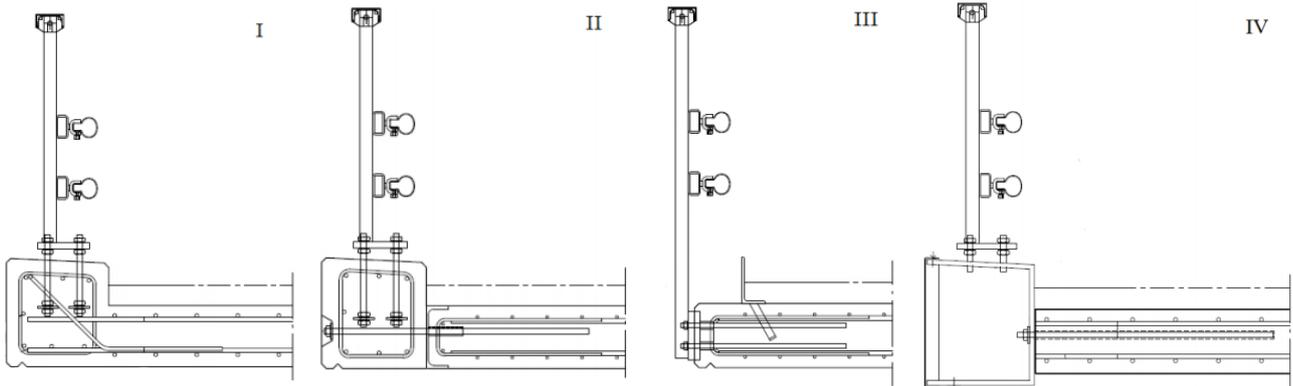
Figure 3-7 – Different types of edge beams
