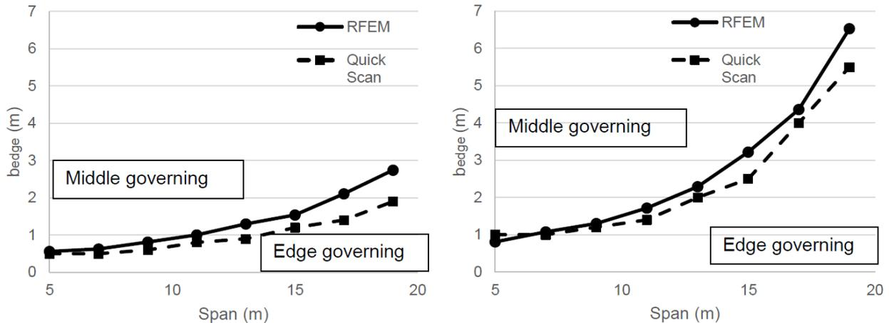
**Figure 8-13 - Graph for the determination of the governing part of the support. RFEM results compared to Excel results. Left: cracked slab. Right: uncracked slab**
