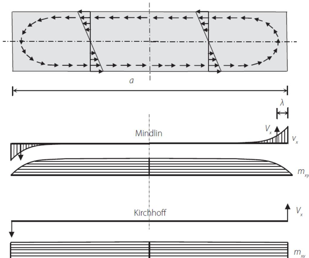
Figure 5-7 - Shear force and torsional moment according to Mindlin and Kirchhoff [47]
