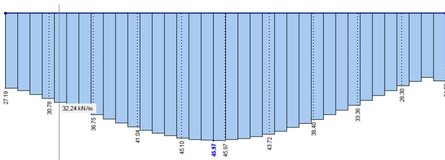
Appendix Figure 6-1 – Shear force due to LM1 axles. (span: 19m,  $b_{edge} = 6m$ ,  $E_y = 33 \text{ GPa}$ ,  $h = 950 \text{ mm}$ )
