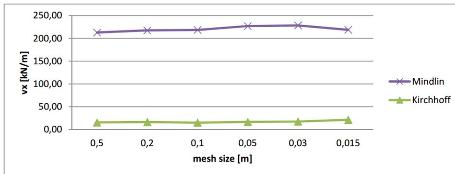
**Figure 5-8 – Maximum shear force on the edge of a thin (200mm) plate for 'Mindlin' and 'Kirchhoff' [48]**
