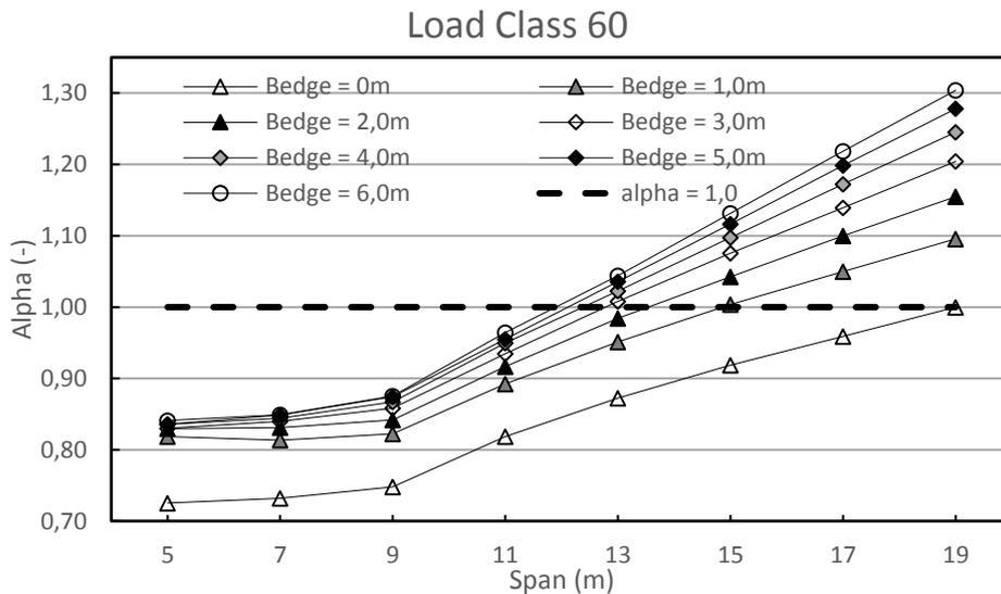
**Figure 6-5 -  $\alpha$  factor (flexural moment) for the comparison of Load Model 1 and Load Class 69 for different spans and edge widths**
