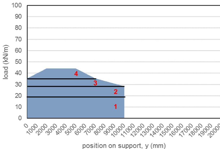
Figure 8-4 – Example of the calculation of the shear force due to UDL loads (Span = 15,0m,  $b_{edge} = 2,0m$ )
