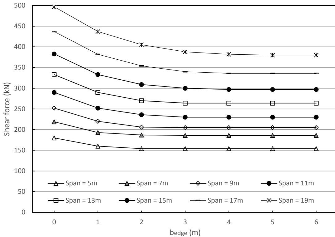
**Figure 7-12 - Shear force near the middle of the support for different spans and edge distances (uncracked)**
