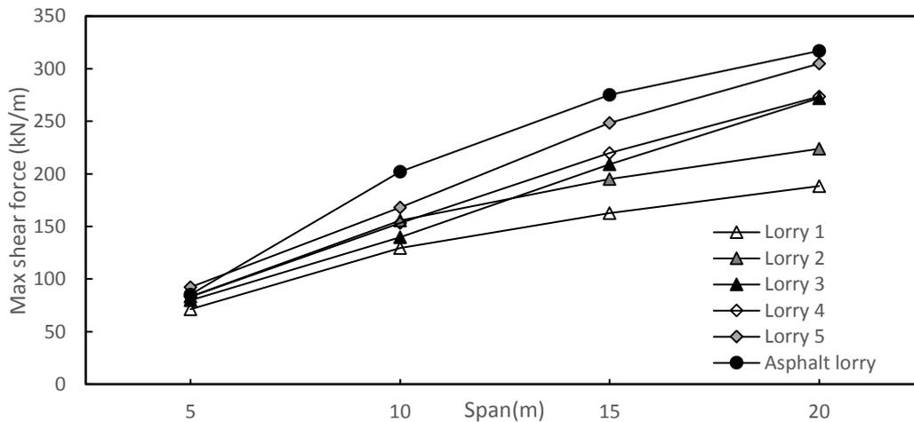
Appendix Figure 8-4 – Shear force for an edge distance of 0m for different fatigue load models
