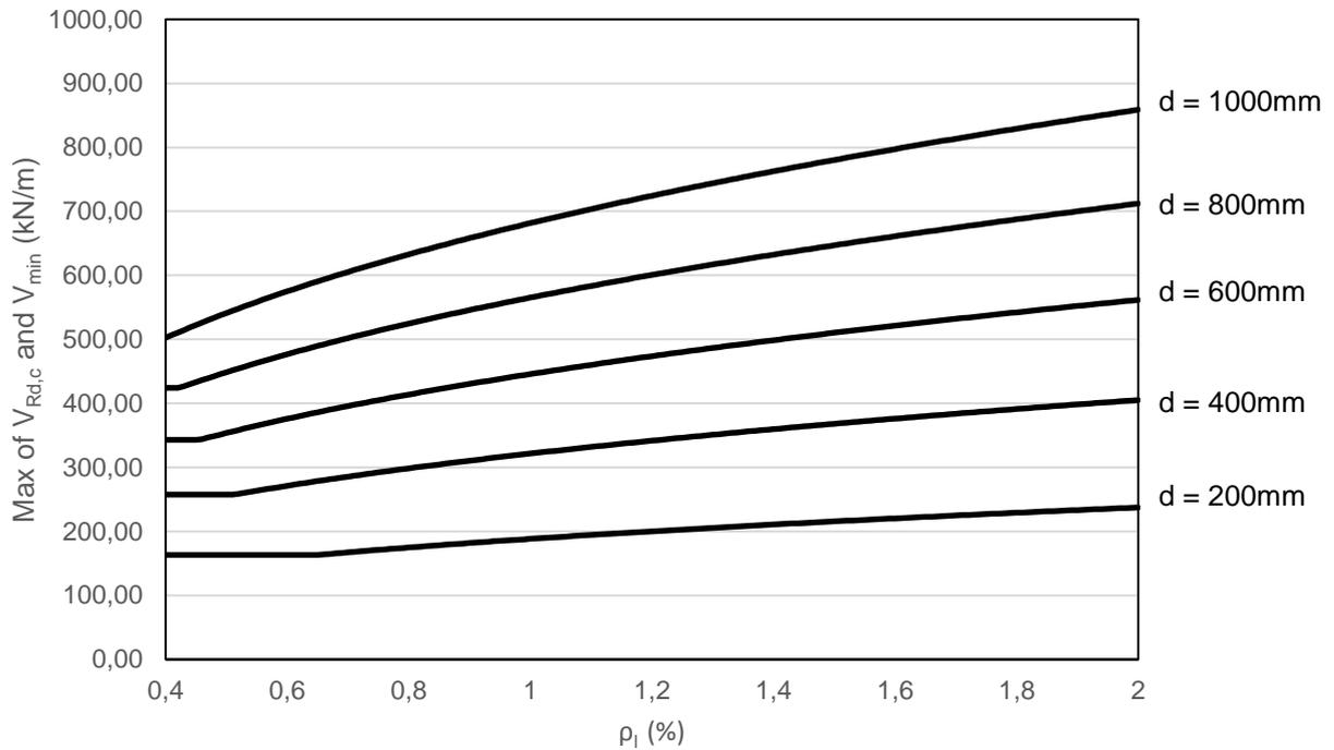
**Figure 8-15 – The maximum value of  $V_{Rd,c}$  or  $V_{min}$  for different effective depths and reinforcement ratios ( $f_{yk} = 500\text{ N/mm}^2$ )**
