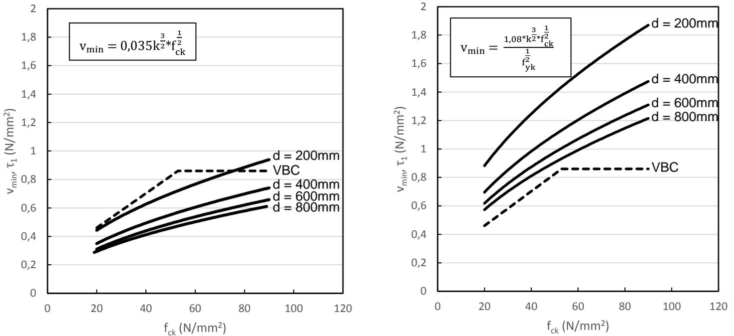
Figure 4-15 -  $v_{min}$  according to EC2 and VBC (left) and according to equation 6.8 (RBK) and VBC (right) for a yield strength of  $f_{yk} = 240 \text{ N/mm}^2$  [39]
