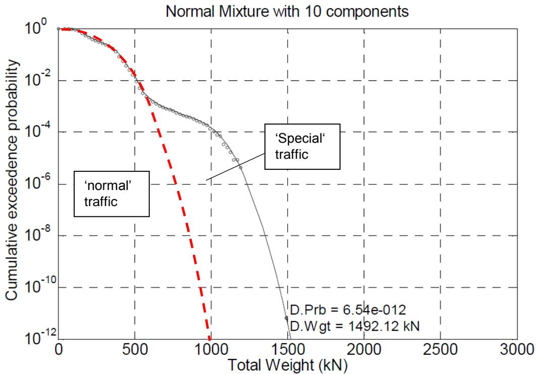
Figure 3-19 – Fitted analytical distribution of the vehicle weight (adapted from [24] and [28])
