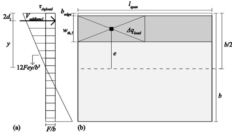
Figure 4-11 - Model for contribution of increased loading in the first heavily loaded lane as compared to other lanes assuming a triangular stress distribution over the support
