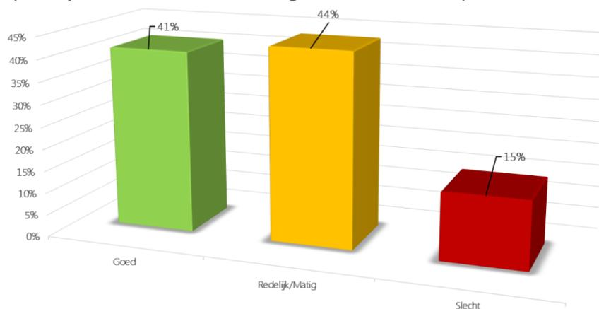
**Figure 2-3 - State of the concrete bridges after inspection (green = good, yellow = moderate, red = bad) [1]**
