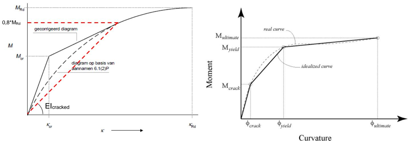
Figure 3-8 –  $M - \kappa$  diagram according to EC2 (left);  $M - \kappa$  diagram (simplified) for reinforced concrete (right) [20]
