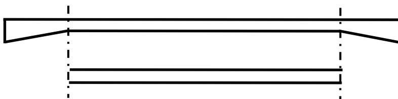
**Figure 8-7 - Illustration of the assessment of a varying longitudinal cross-section**
