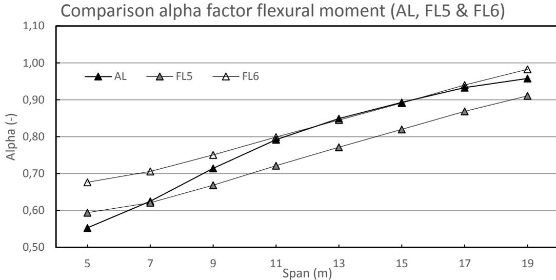
**Figure 6-6 -  $\alpha$  factors (flexural moment) for the comparison of Load Model 1 and AL, FL5 and FL 6 different spans. Edge width = 2m**
