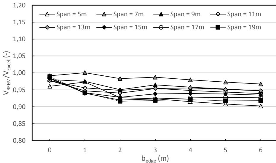
**Figure 8-12 - Comparison shear force RFEM and Excel near the middle of the support for uncracked slabs**
