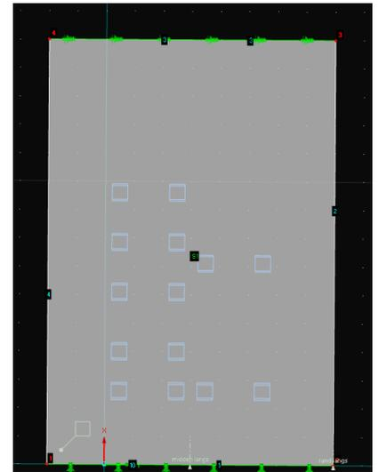
Figure 6-2 - Load model: asphalt lorry (with a normal truck on lane 2)
