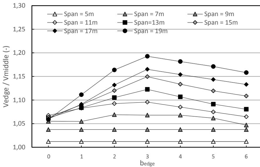
Appendix Figure 10-8 - Comparison of shear force near the edge divided by the shear force near the middle of the support due to self-weight (cracked slab)
