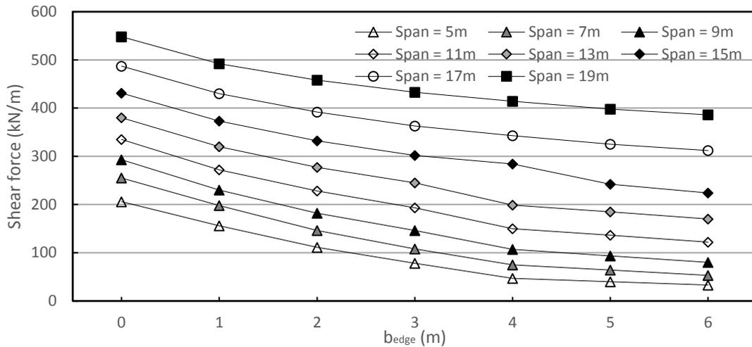
Figure 7-14 – Shear force near the edge of the support for different spans and edge distances (uncracked)
