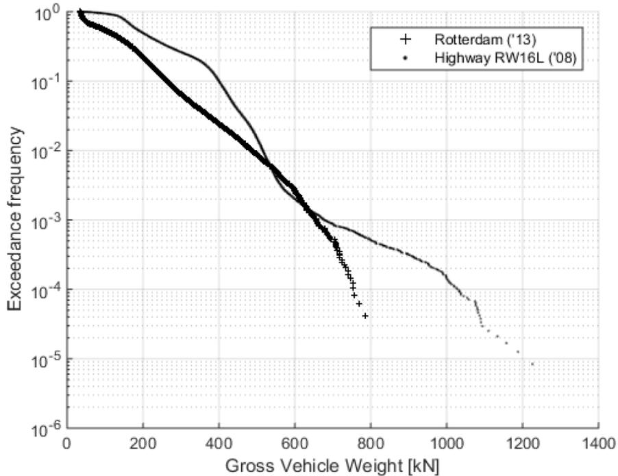
Figure 3-15 - Vehicle load distributions in Rotterdam and RW16-L [27]
