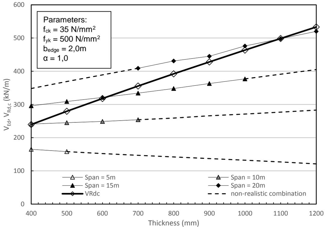
**Figure 8-9 - Shear force and shear capacity for varying thickness**
