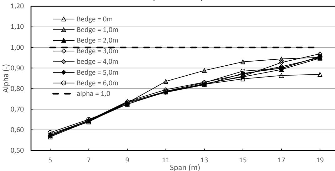
**Appendix Figure 9-11 - A factor (Shear force) for the comparison of Load Model 1 and the Asphalt Lorry for different spans and edge widths**
