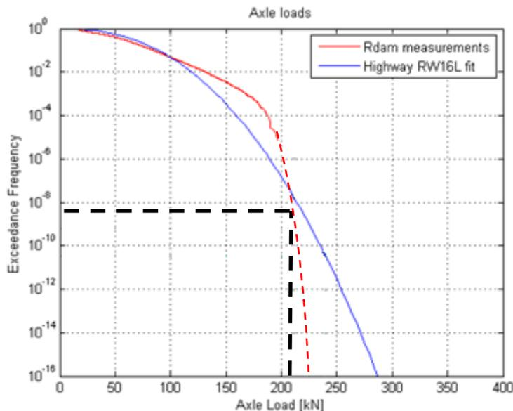
**Figure 3-17 - Comparison of axle load distributions: Dutch highways (fit), Rotterdam (empirical), existing bridges (as calculated:  $5 * 10^{-9}$ ) [26]**
