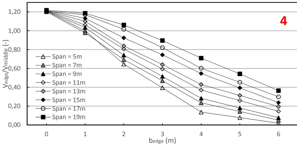
**Appendix Figure 10-11 - Comparison of shear force near the edge divided by the shear force near the middle of the support due to axle loads (uncracked slab)**
