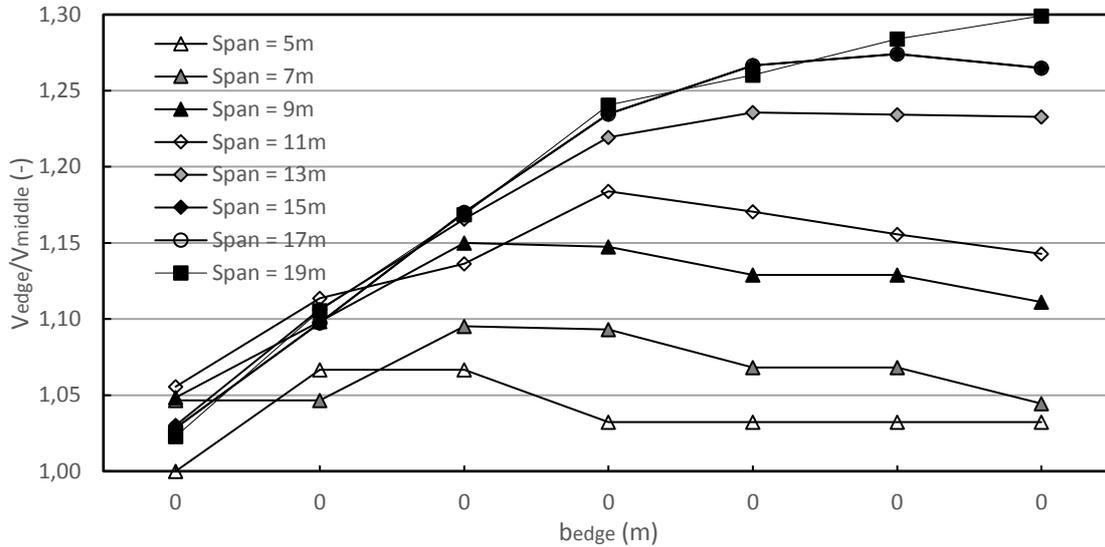
**Figure 7-5 – Shear force near the edge of the support over the shear force near the middle of the slab due to permanent loads for different spans and edge distances (uncracked slab)**
