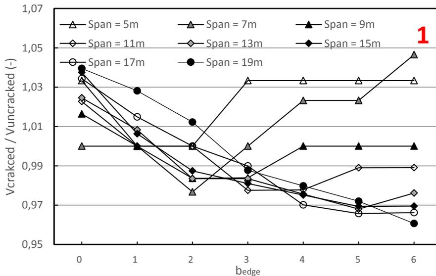
Appendix Figure 10-2 - Comparison of shear force due to self-weight near the middle of the support (cracked divided by uncracked)
