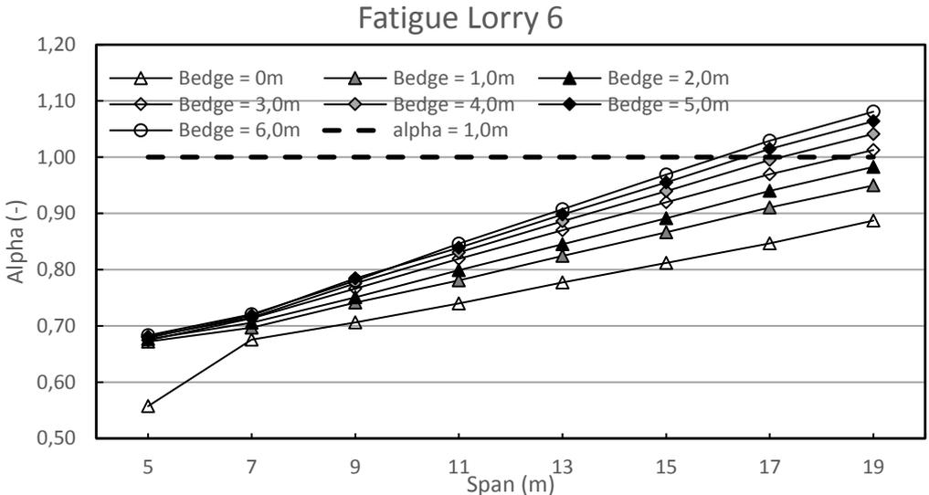
Figure 6-4 -  $\alpha$  factor (flexural moment) for the comparison of Load Model 1 and fatigue load model 6 for different spans and edge widths
