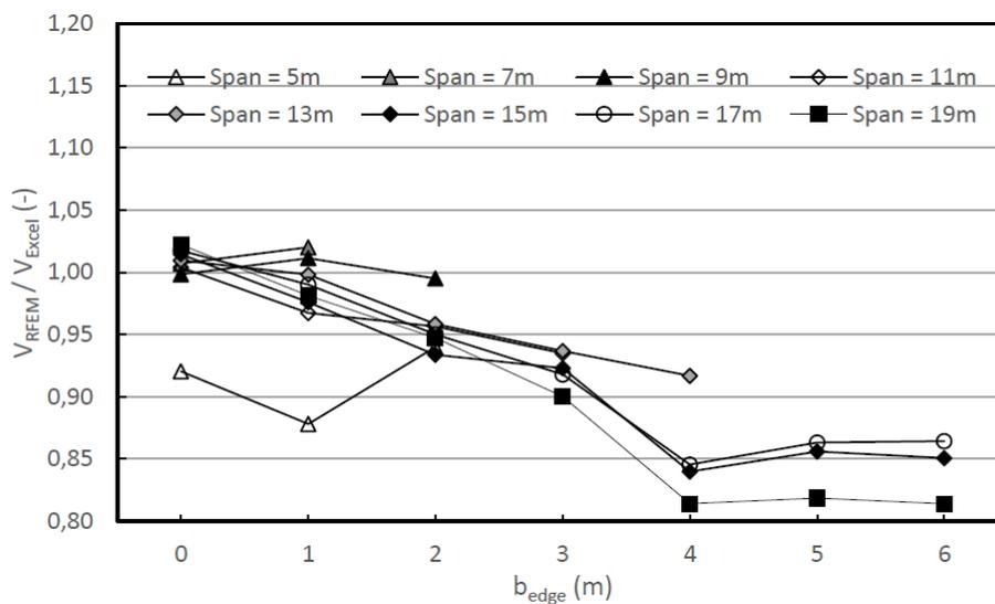
**Appendix Figure 14-1 - Comparison shear force RFEM and Excel near the edge of the support for cracked slabs**
