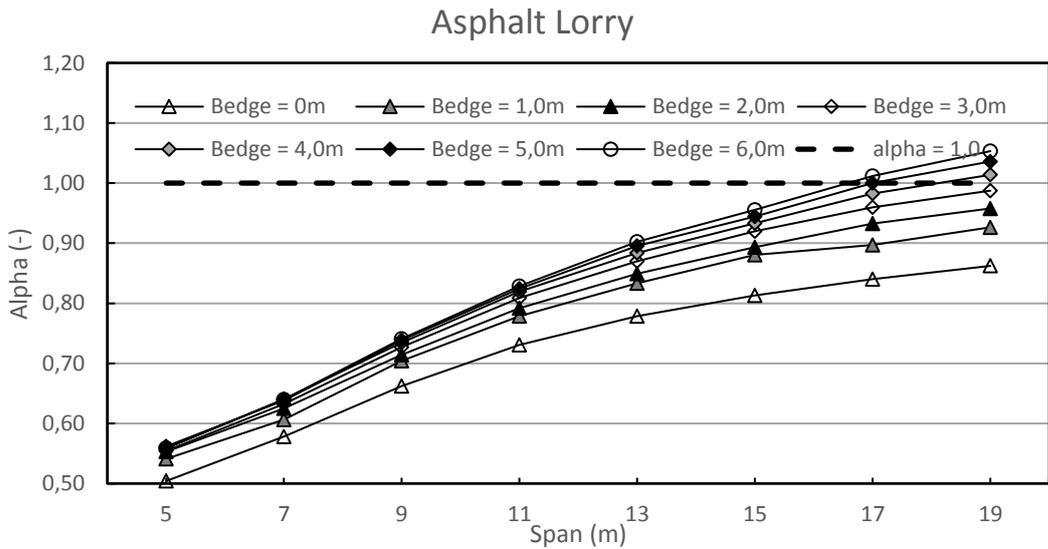
**Appendix Figure 9-3 - A factor (flexural moment) for the comparison of Load Model 1 and the Asphalt Lorry for different spans and edge widths**
