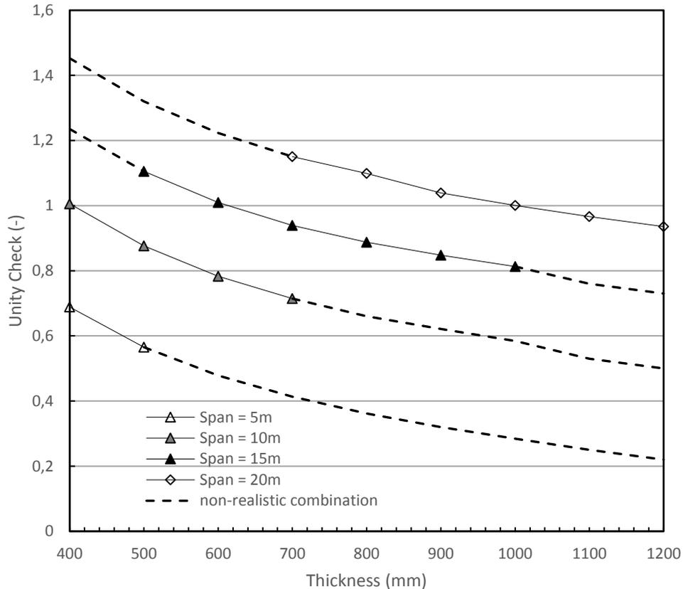
**Figure 8-10 - Unity check for shear force for varying thickness**
