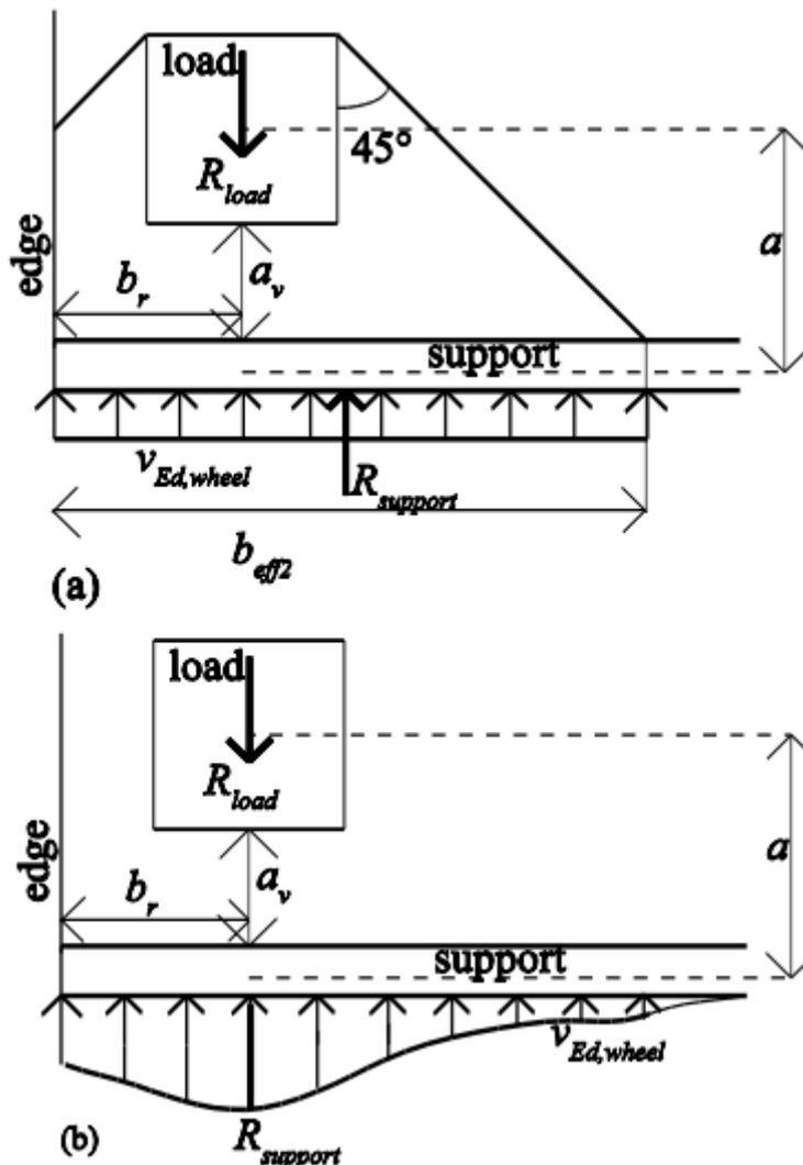
Figure 4-4 - Shear force for wheel loads close to the edge: (a) Different location of resultant of shear force over support  $R_{support}$  and applied wheel load  $R_{load}$ ; (b) Real stress distribution at the support, in which the moment imbalance is not occurring anymore. [31]
