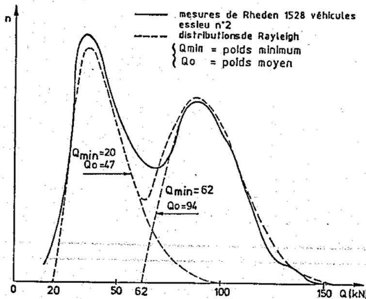
Figure 3-14 - Axle load distributions for Eurocode calibration [26]
