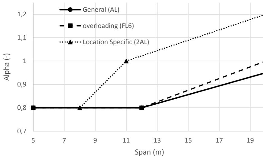
Appendix Figure 9-7 - General  $\alpha$  factor for flexural moment, small edge widths
