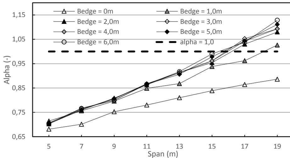
Appendix Figure 9-10 - A factor (Shear force) for the comparison of Load Model 1 and Load Class 45 for different spans and edge widths
