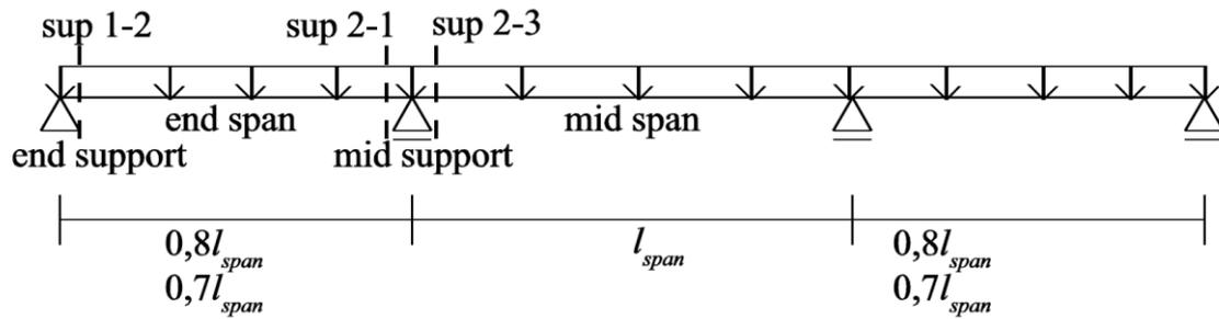
Figure 4-14 – Considered sections for a typical three span bridge [31]
