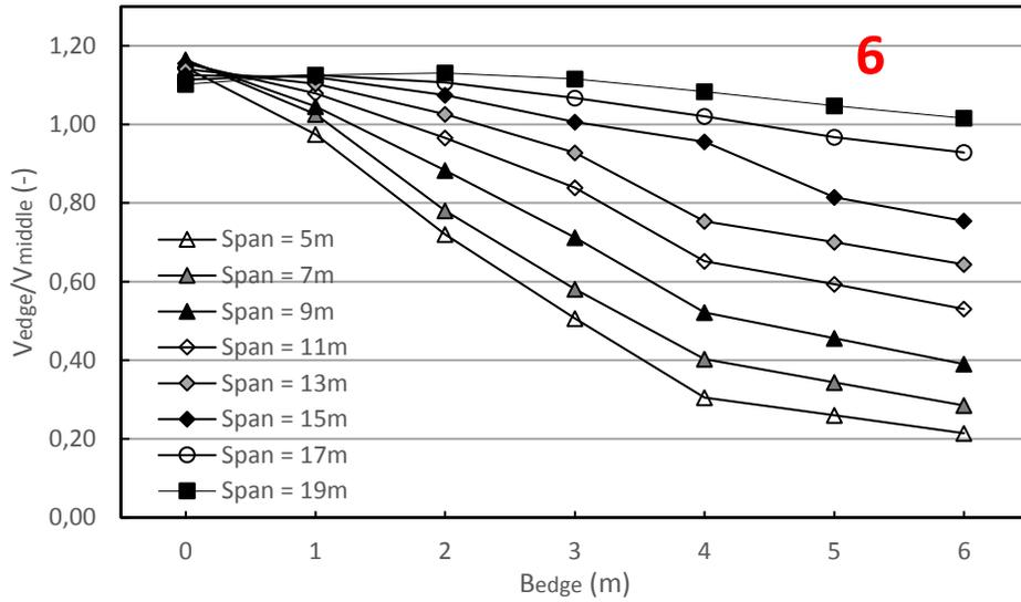
**Appendix Figure 10-13 - Comparison of shear force near the edge divided by the shear force near the middle of the support due to total loads (uncracked slab)**
