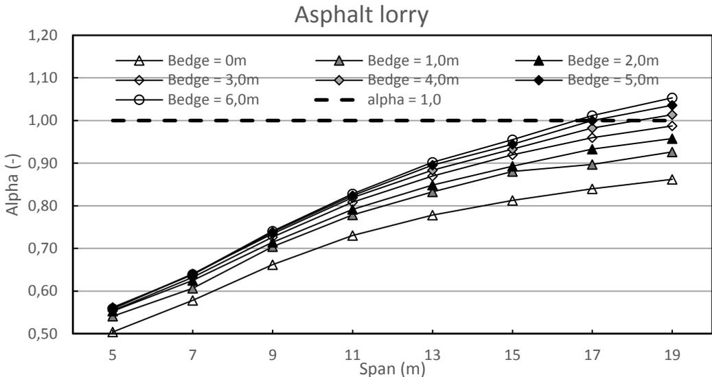
Figure 6-3 -  $\alpha$  factor (flexural moment) for the comparison of Load Model 1 and the asphalt lorry for different spans and edge widths
