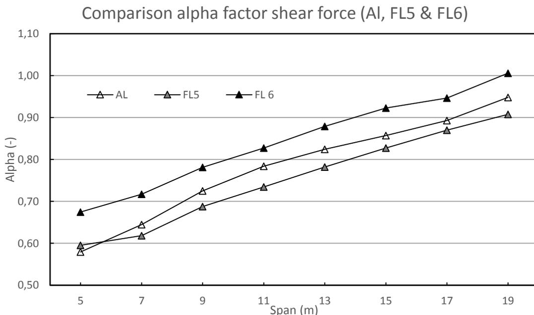
**Figure 6-10 -  $\alpha$  factors (Shear force) for the comparison of Load Model 1 and AL, FL5 and FL 6 different spans. Edge width = 2m**
