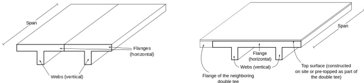
**Figure 3-1 - Example of a T-beam (left) and a double T-beam (right) (source: <https://en.wikipedia.org/wiki/T-beam>)**
