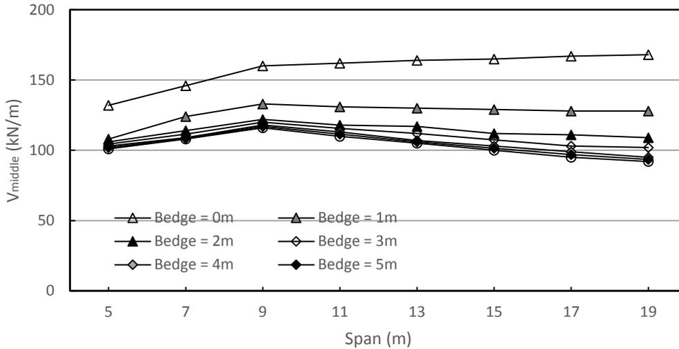
**Figure 7-8 – Shear force near the middle of the slab for an uncracked slab.**
