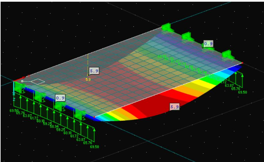
Appendix Figure 7-2 - Deflection by self-weight, 0,9mm at support, span: 10m
