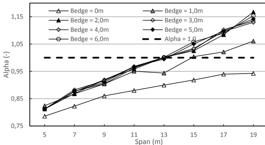
Appendix Figure 9-9 - A factor (Shear force) for the comparison of Load Model 1 and Load Class 60 for different spans and edge widths
