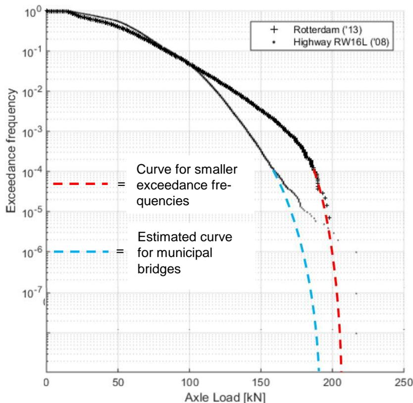
Figure 8-14 - Hypothetical path of the graph for axle loads of 'normal traffic' <sup>4</sup>
