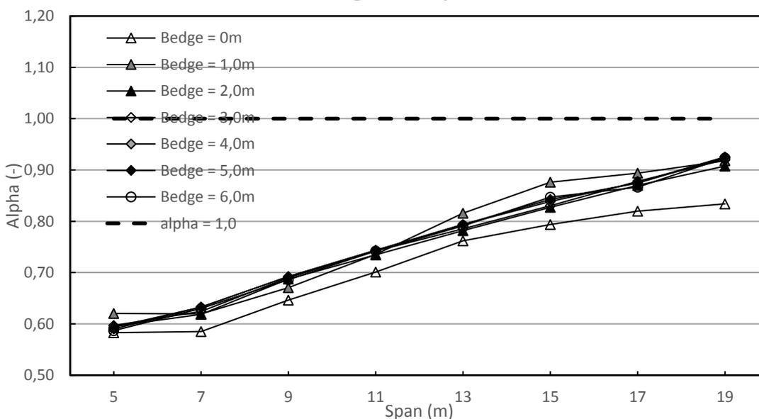
**Appendix Figure 9-12 - A factor (Shear force) for the comparison of Load Model 1 and the Fatigue Lorry 5 for different spans and edge widths**
