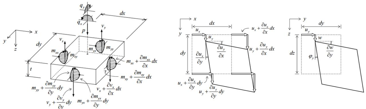
**Figure 5-2 - positive loads and stress resultants [44] Figure 5-1 - Displacements and deformations of an elementary plate part [44]**
