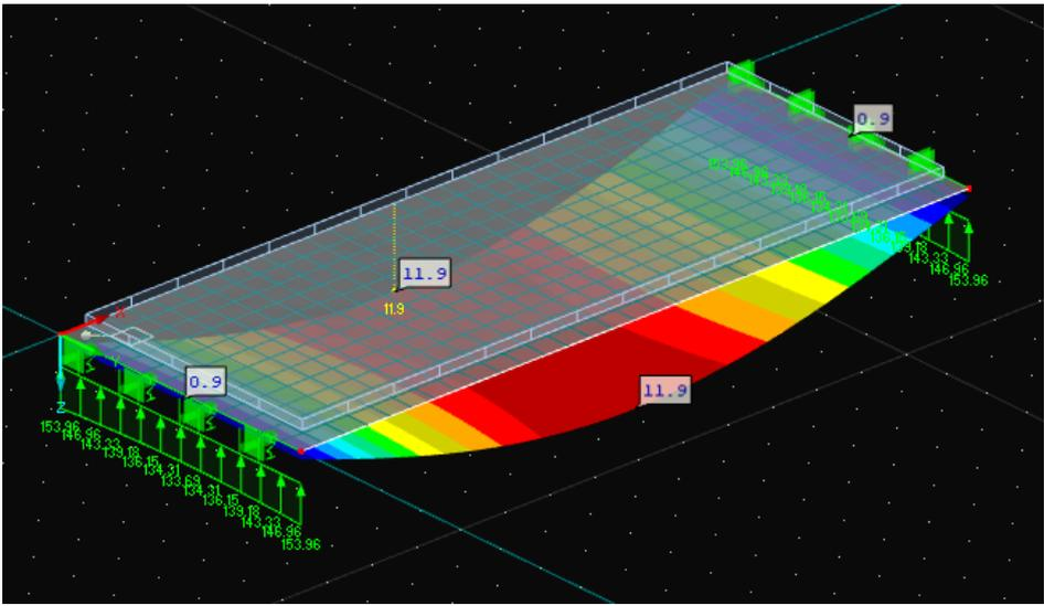
**Appendix Figure 7-3 - Deflection by self-weight, 0,9mm at support, span: 15m**
