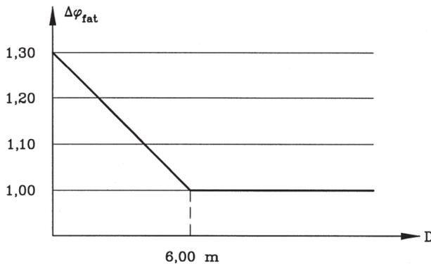
**Figure 5-12 - The dynamic factor for the distance  $D$  from the expansion joint [2]**
