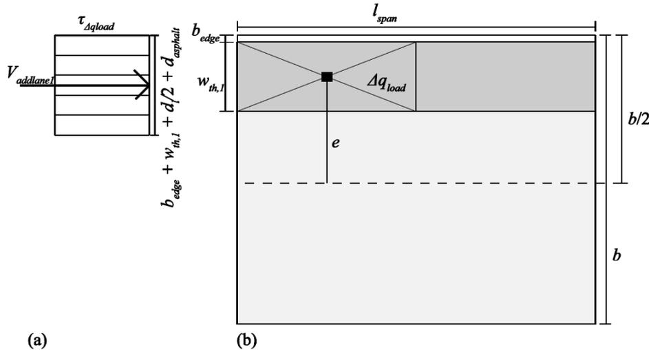
Figure 4-13 – model for the contribution of increased loading in the first heavily loaded lane. a) assumed stress distribution b) sketch of the top view with location of the first heavily loaded lane
