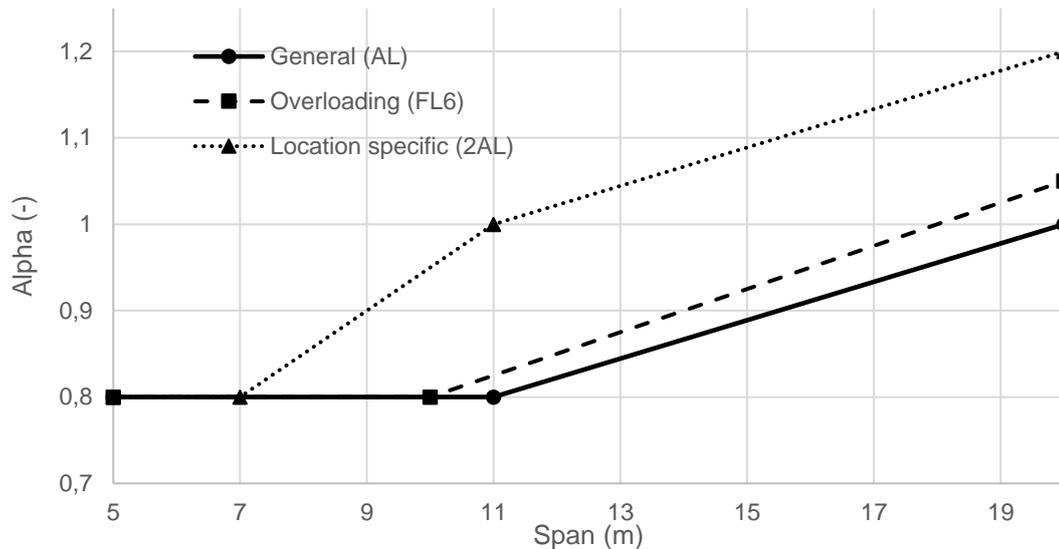
**Figure 6-11 - A factor for general municipal bridges, overloaded bridges and bridges with location specific loading**
