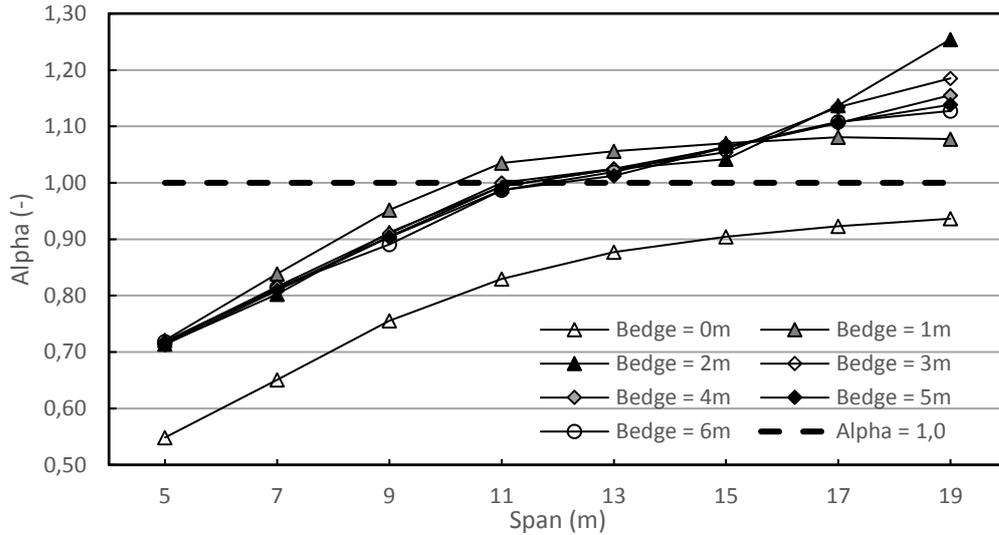
**Appendix Figure 9-14 -  $\alpha$  factor (Shear force) for the comparison of Load Model 1 and two asphalt lorries for different spans and edge widths**
