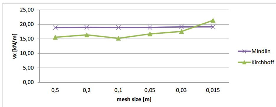
**Figure 5-9 - Maximum shear force on the edge of a thick (2250mm) plate for 'Mindlin' and 'Kirchhoff' [48]**
