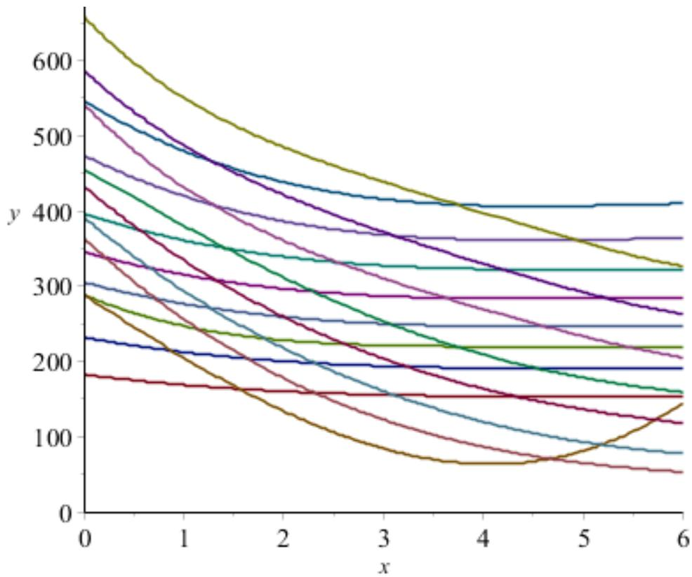
**Appendix Figure 13-2 - Calculation of the intersection of graphs for shear force near the middle and near the edge of the slab (cracked slab)**
