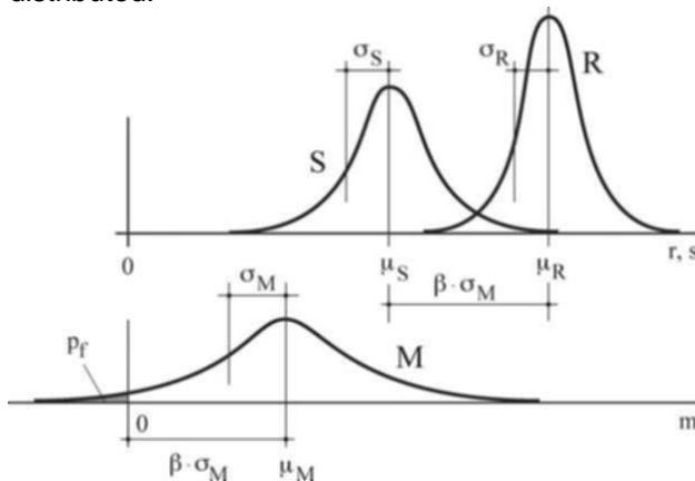
**Figure 3-10 – Visualisation of the equation  $M = R - S$  [25]**
