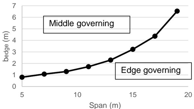
Figure 7-15 - Graph for the determination of the governing part of the support (uncracked prefab slab)
