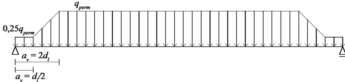
Figure 8-3 - Resulting distributed load for permanent loads when  $\beta(x)$  is taken into account [36]
