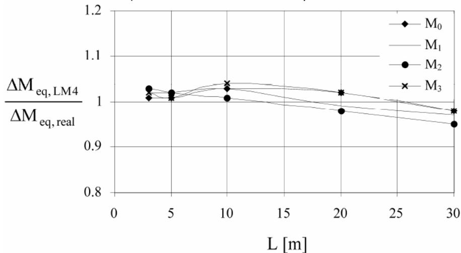
**Figure 5-11 - Accuracy of fatigue load model 4 [8]**
