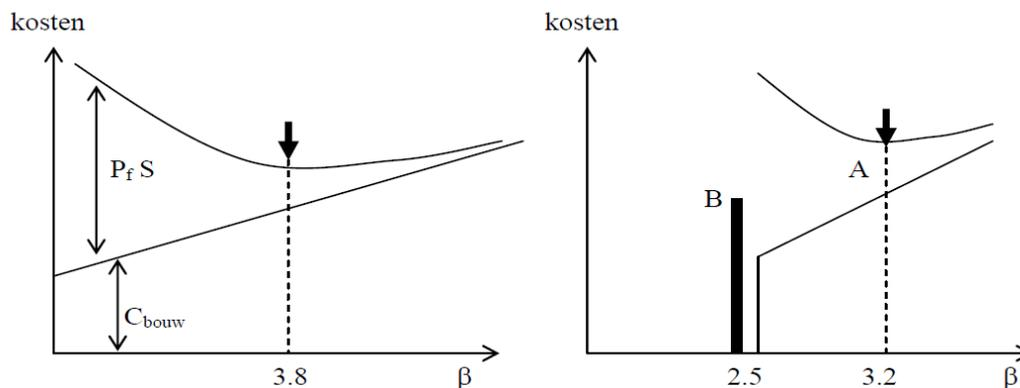
Figure 3-12 - Optimization of building and repair costs (right: new structures, left: existing structures) [22]
