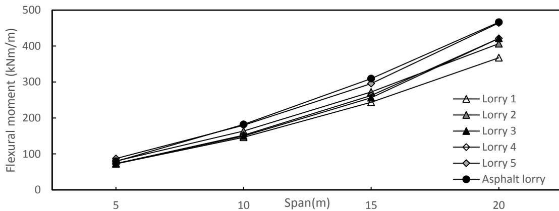
Appendix Figure 8-1 - Flexural moment for an edge distance of 0m for different fatigue load models
