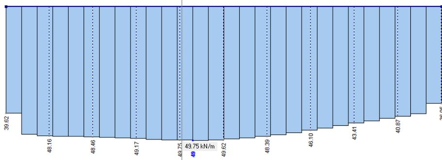
Appendix Figure 6-3 - Shear force due to LM1 axles. (span: 19m,  $b_{edge} = 4m$ ,  $E_y = 33 \text{ GPa}$ ,  $h = 950 \text{ mm}$ )
