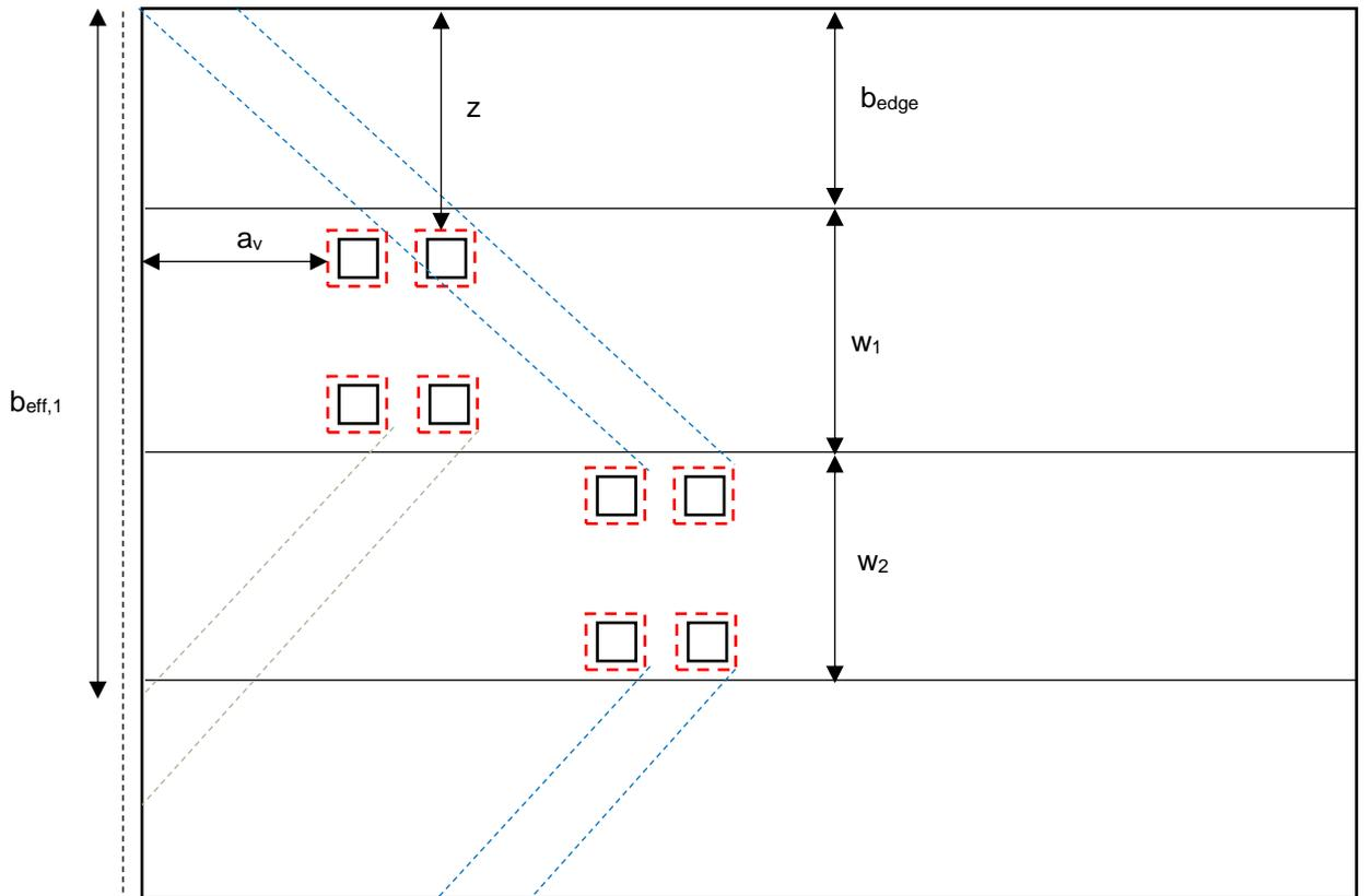
**Figure 8-2 - Load configuration for the maximum shear force near the edge of the support**
