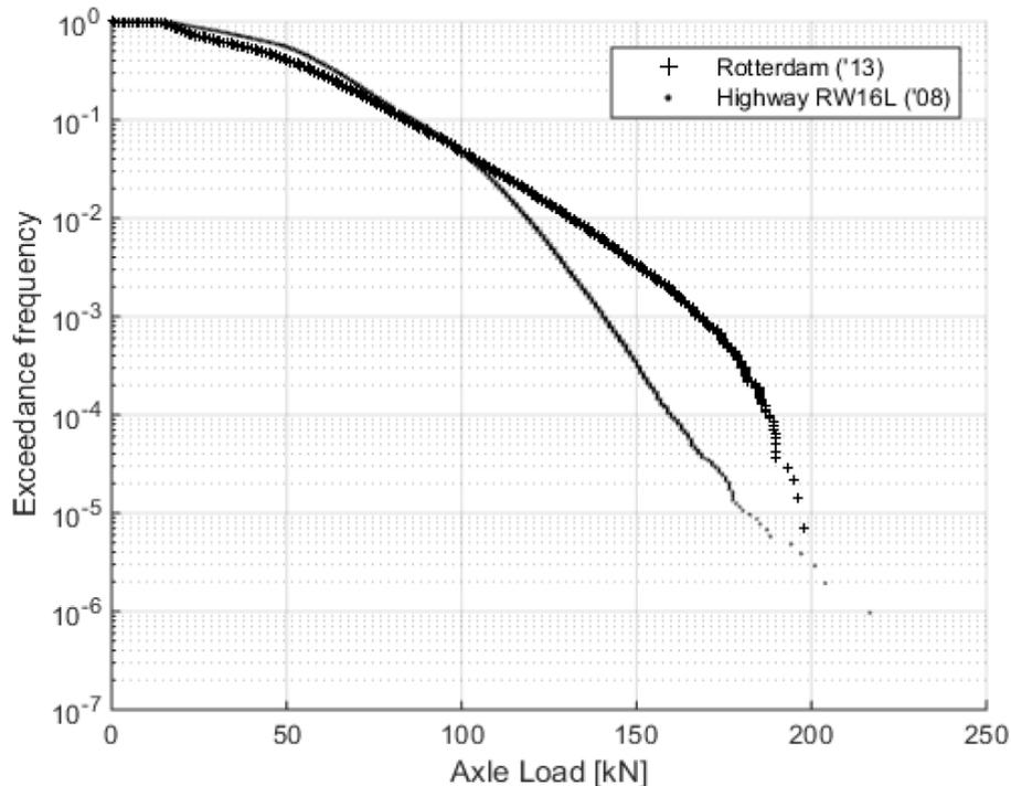
Figure 3-16 - Axle load distributions in Rotterdam and RW16-L [27]
