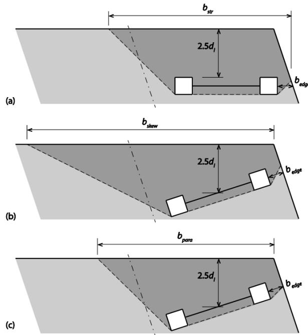
**Figure 4-7 - Possible ways to determine the effective width of a single axle in shear for a skewed slab [35]**
