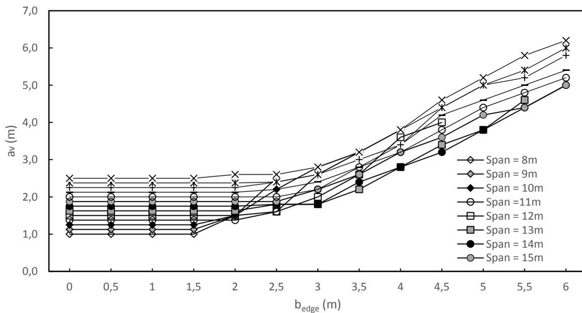
Appendix Figure 12-1 –  $a_v$  values for lane 1 for different spans and edge widths
