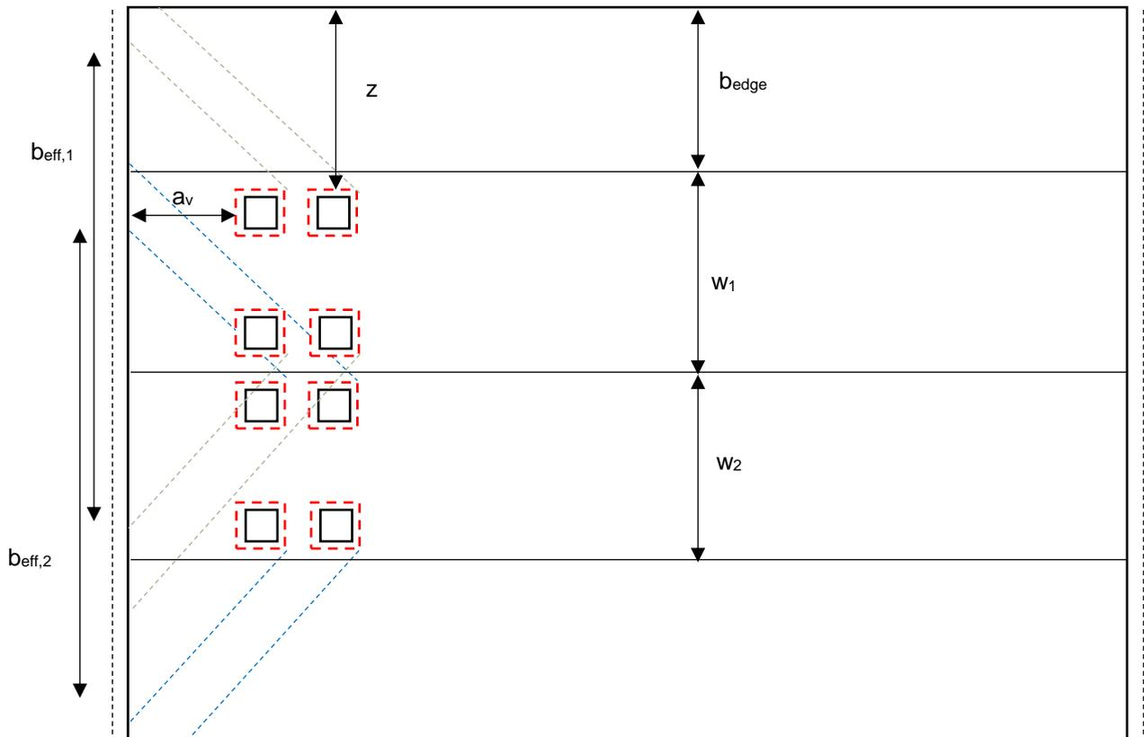
**Figure 8-1 - Load configuration for the maximum shear force near the middle of the support**
