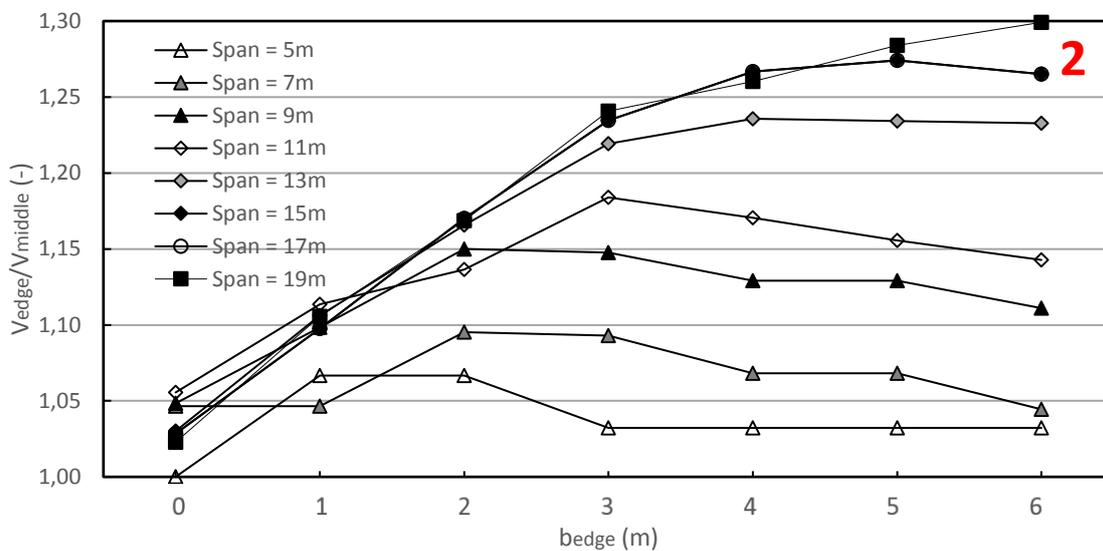
Appendix Figure 10-9 - Comparison of shear force near the edge divided by the shear force near the middle of the support due to self-weight (uncracked slab)
