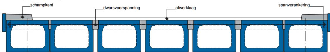
Figure 3-2 - cross-section SKK bridge [14]
