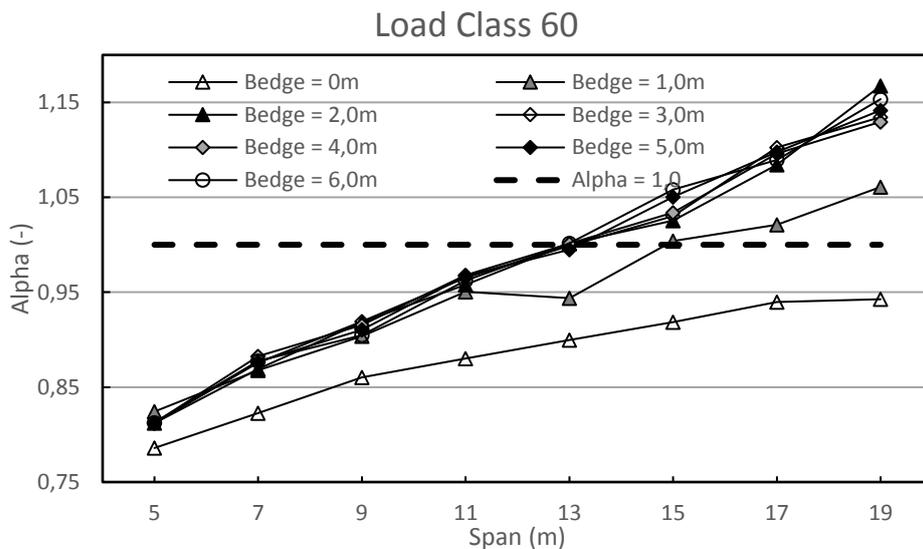
**Figure 6-9 -  $\alpha$  factor (Shear force) for the comparison of Load Model 1 and Load Class 60 for different spans and edge widths**
