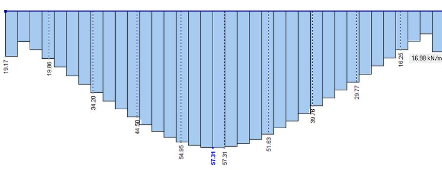
Appendix Figure 6-2 Shear force due to LM1 axles. (span: 19m, bedge = 6m,  $E_y = 11 \text{ GPa}$ ,  $h = 950 \text{ mm}$ )
