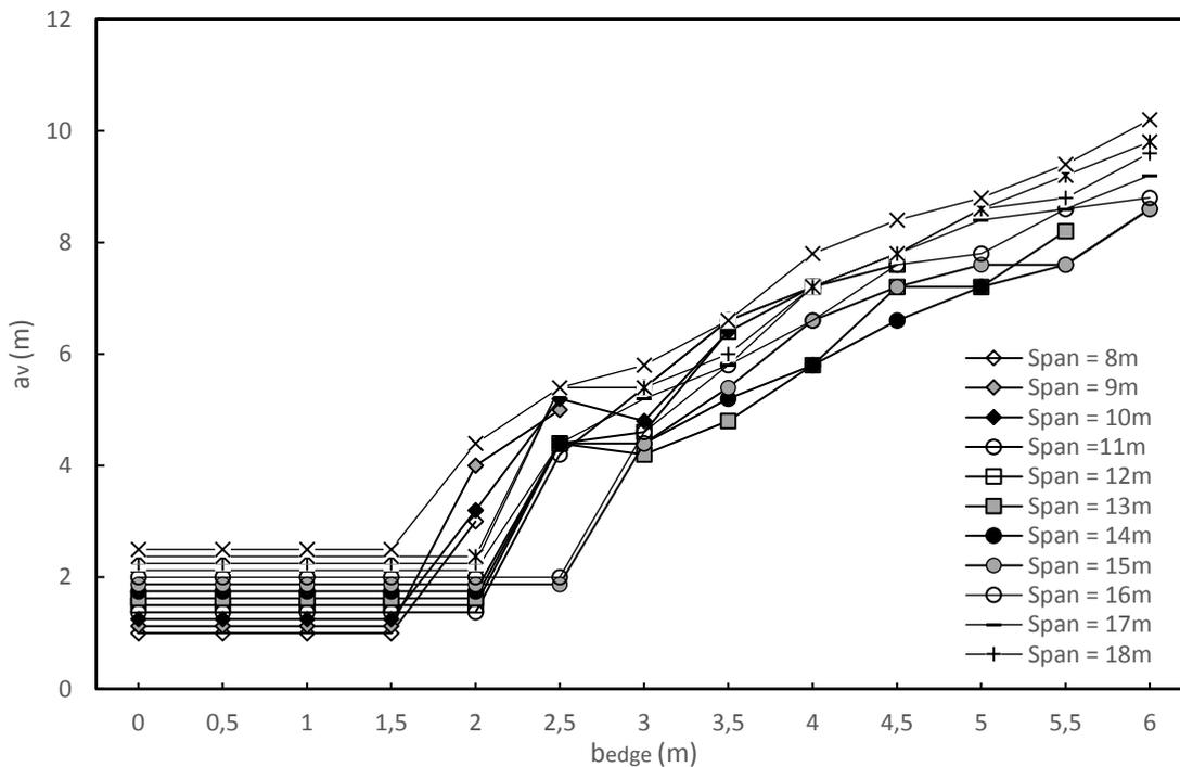
Appendix Figure 12-2 -  $a_v$  values for lane 2 for different spans and edge widths
