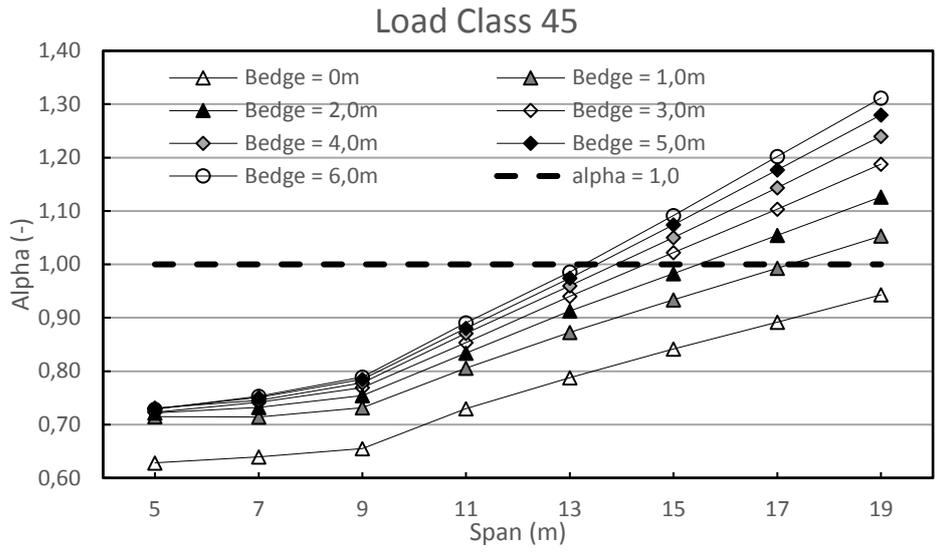
**Appendix Figure 9-2 - A factor (flexural moment) for the comparison of Load Model 1 (CG2) and Load Class 45 for different spans and edge widths**
