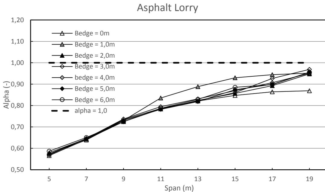
**Figure 6-7 -  $\alpha$  factor (Shear force) for the comparison of Load Model 1 and the Asphalt Lorry for different spans and edge widths**
