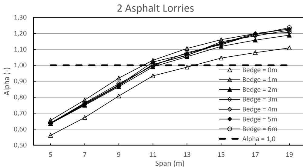
**Appendix Figure 9-6 - A factor (flexural moment) for the comparison of Load Model 1 and two Asphalt Lorries (location specific) for different spans and edge widths**
