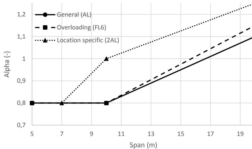
Appendix Figure 9-8 - General  $\alpha$  factor for flexural moment, large edge widths
