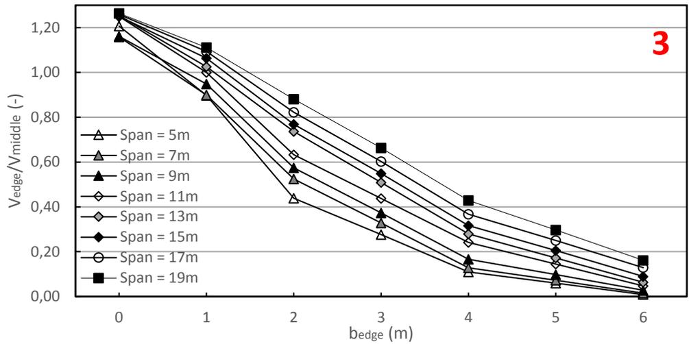
**Appendix Figure 10-10 - Comparison of shear force near the edge divided by the shear force near the middle of the support due to axle loads (cracked slab)**
