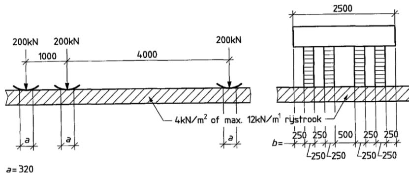
**Figure 5-10 - Axle configuration of load class 60 [51]**
