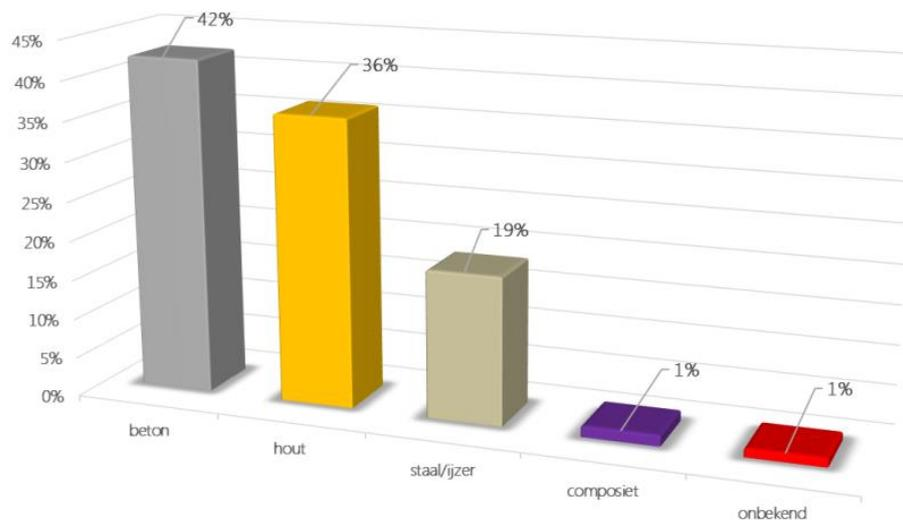
**Figure 2-1 - Structural material bridges. (Translation from left to right: concrete, timber, steel, composite, unknown) [1]**
