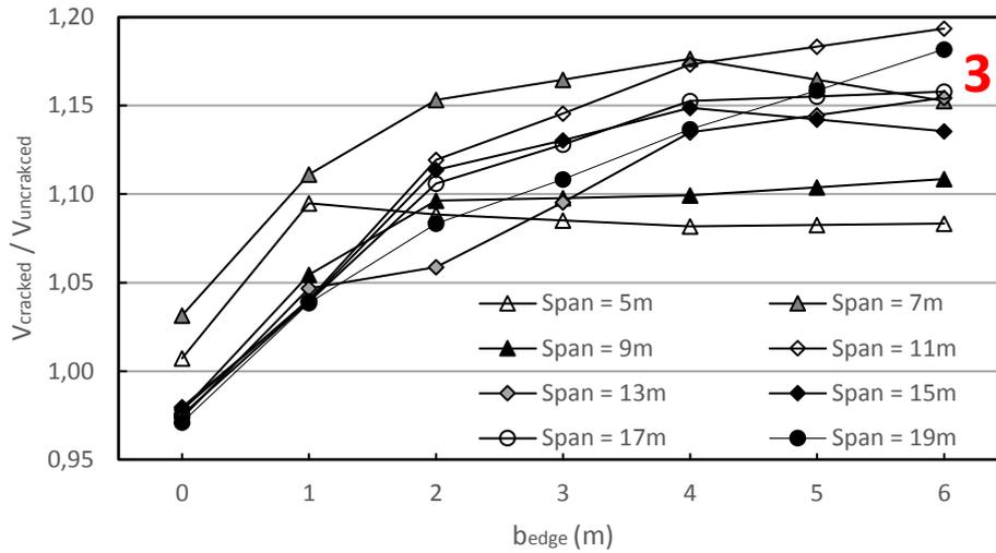
**Appendix Figure 10-4 - Comparison of shear force due to axle loads near the middle of the support (cracked divided by uncracked)**
