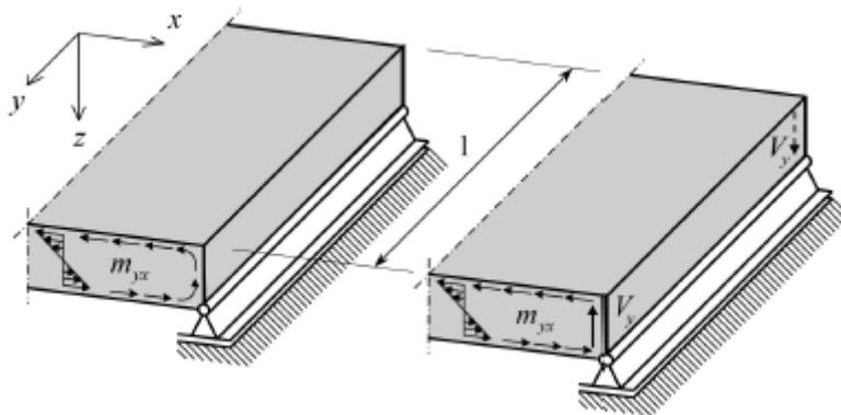
**Figure 5-4 - Constant twisting moment at the edge [45]**
