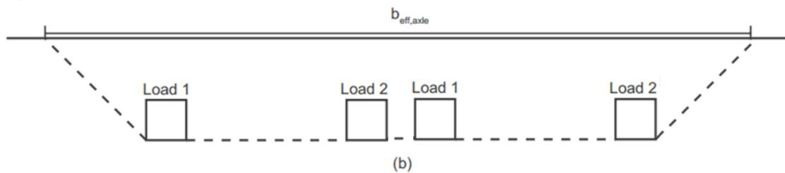
Figure 4-6 - Effective width of 2 axles together
