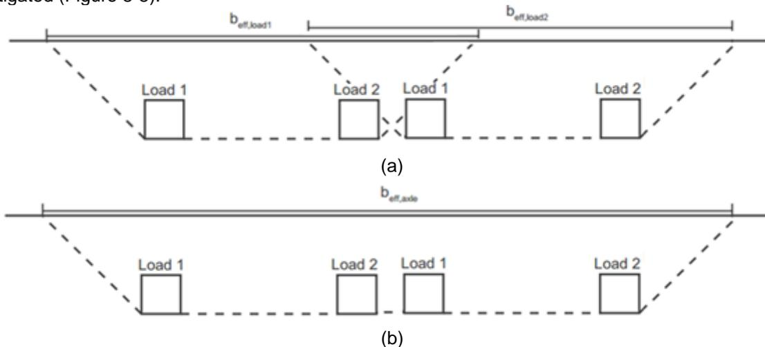
**Figure 8-5 – Effective width of two axles separately (a) and two axles together (b)**
