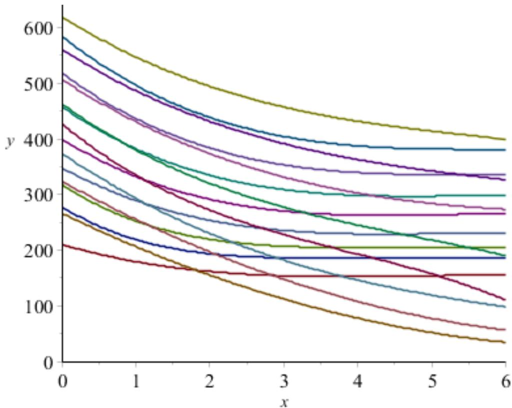
**Appendix Figure 13-1 – Calculation of the intersection of graphs for shear force near the middle and near the edge of the slab (uncracked slab)**
