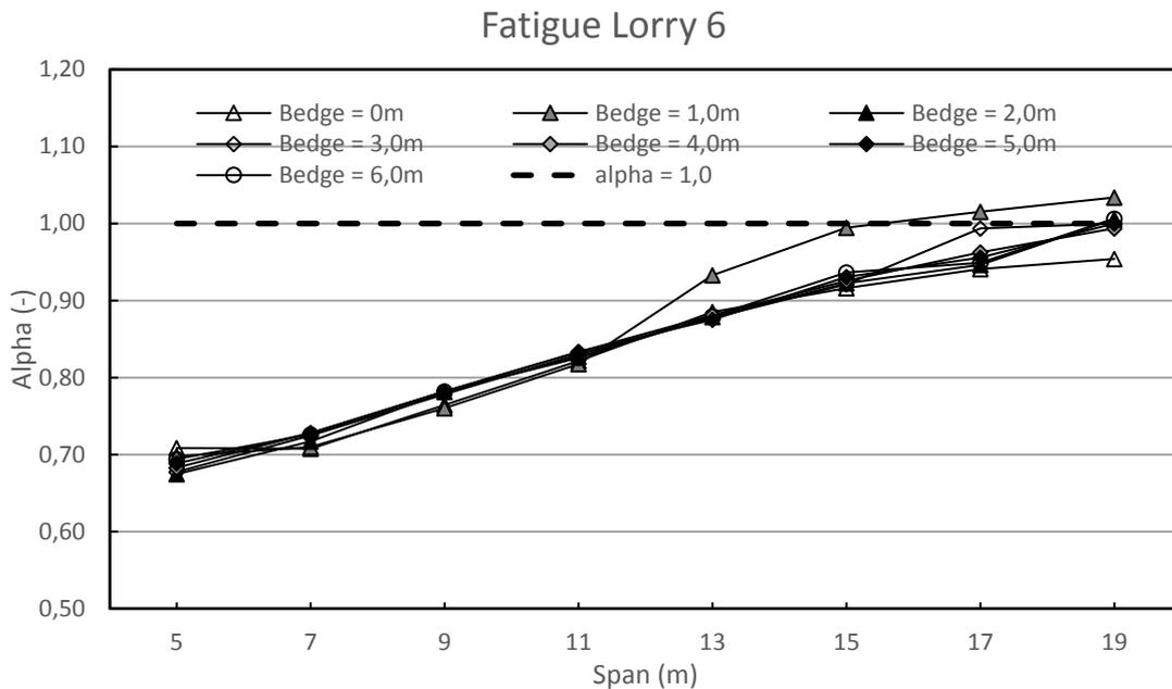
**Figure 6-8 -  $\alpha$  factor (Shear force) for the comparison of Load Model 1 and the Fatigue Lorry 6 for different spans and edge widths**
