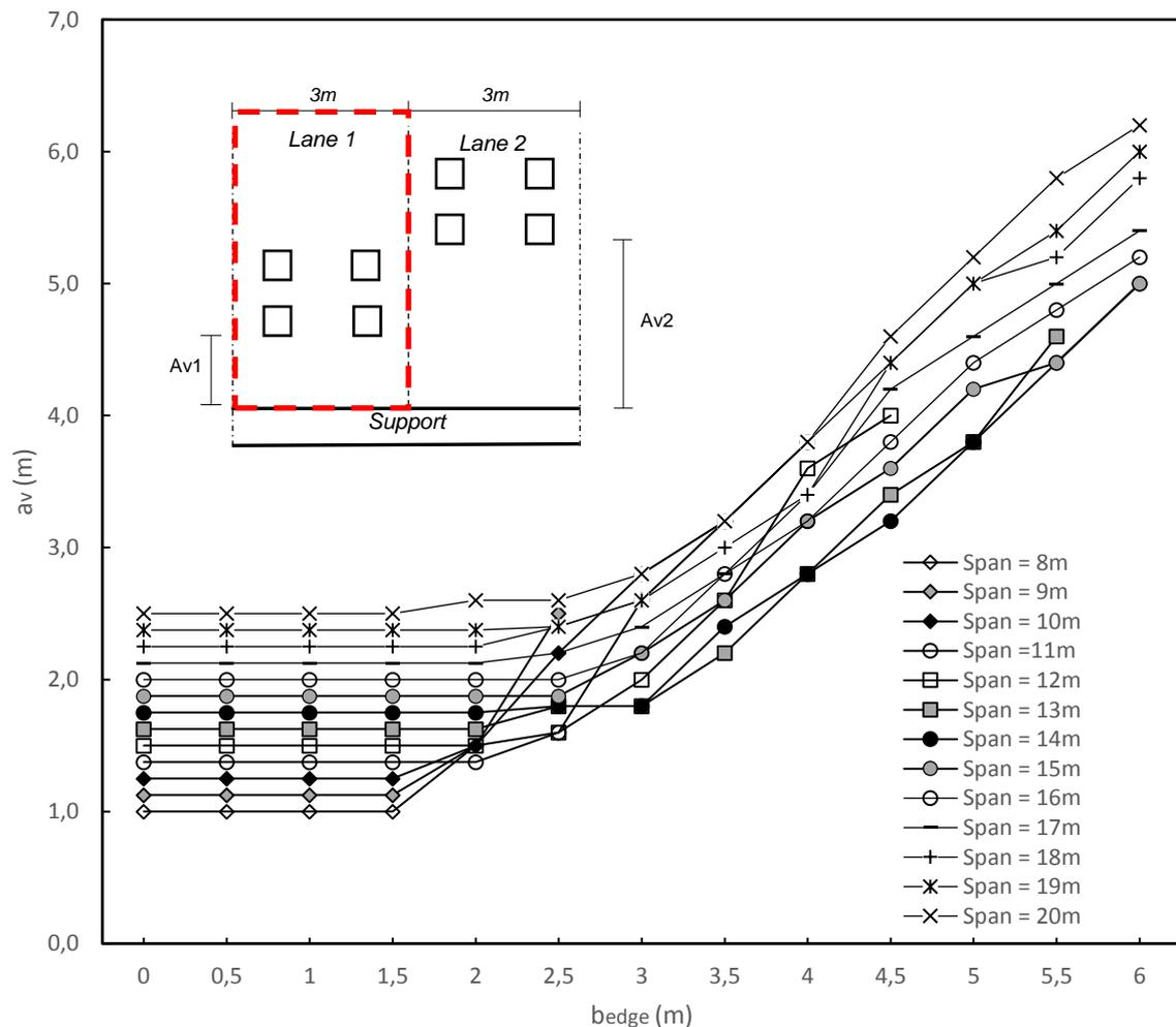
**Figure 7-13 -  $a_v$  lane 1 for different spans and edge distances**
