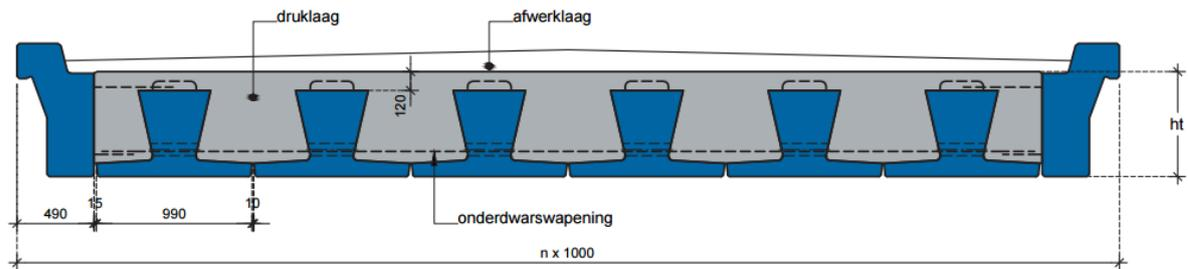
Figure 3-5 - cross-section SJP bridge [14]
