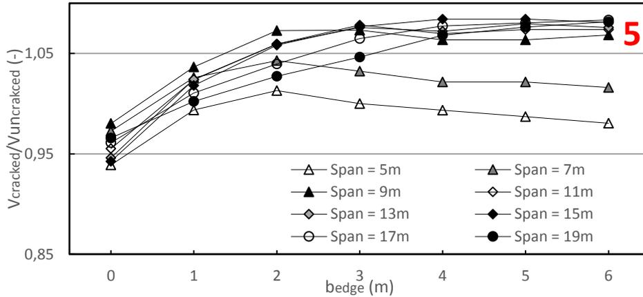
**Appendix Figure 10-6 - Comparison of shear force due total loads near the middle of the support (cracked divided by uncracked)**
