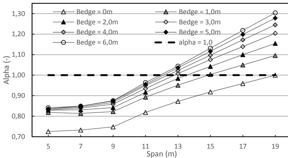
**Appendix Figure 9-1 - A factor (flexural moment) for the comparison of Load Model 1 (CC3) and Load Class 60 for different spans and edge widths**
