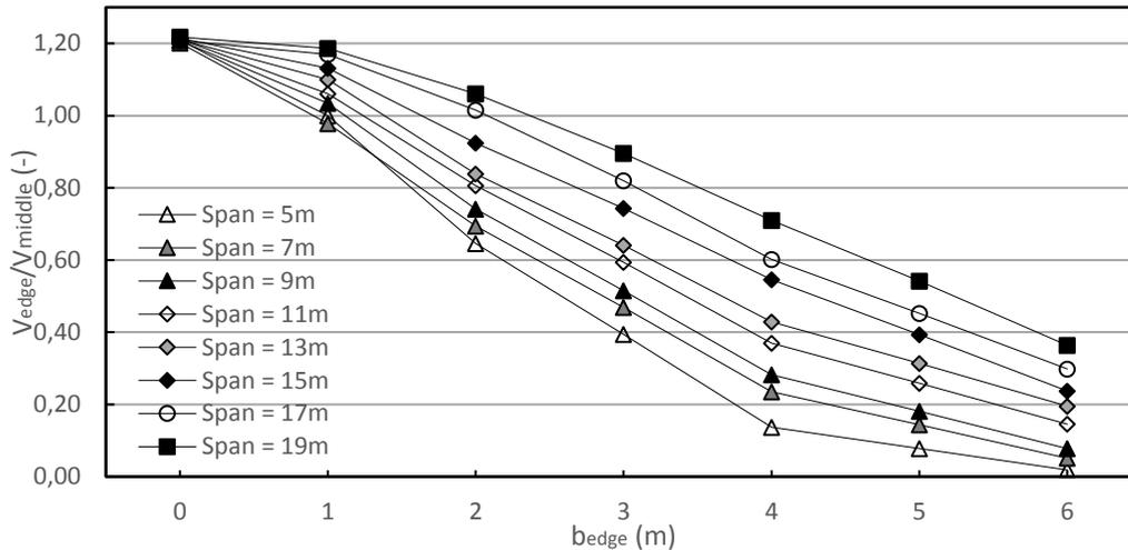
**Figure 7-10 - Shear force near the edge of the support over the shear force near the middle of the slab due to axle loads for different spans and edge distances (uncracked slab)**
