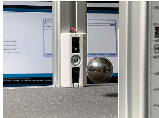
Figure 3. Three different sensor holders are available, the stacked sensors allow to determine the instantaneous velocity.
