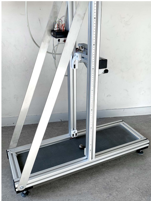
Figure 2. The experimental setup consists of a tall frame with a sensor adjustable in height at the top and one fixed at the bottom.
