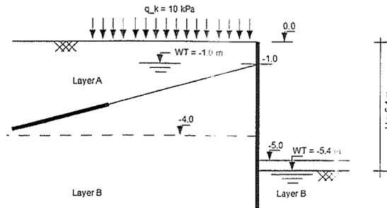
Figure 2: Geometry of the embedded sheet pile wall
