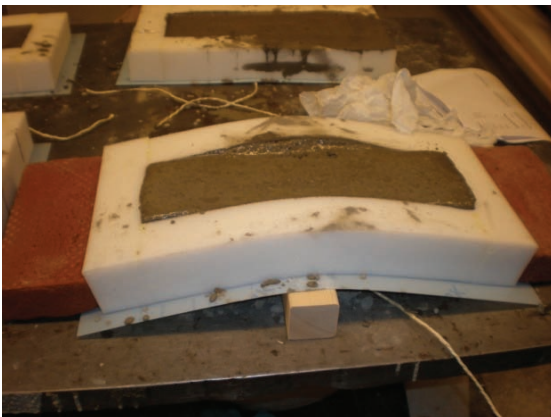
Figure 7: Small-scale test for curved elements; the yield value of the mixture is too low as can be seen from the concrete level
