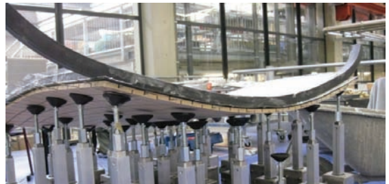
Figure 3: Actuator mould tested by Huyghe and Schoofs (Huyghe & Schoofs, 2009)
