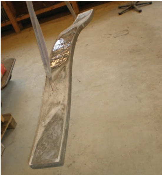
Figure 8: Single-curved Element 5 after demoulding
