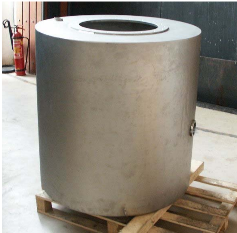
Figure 5: The stainless-steel vessel of DELPHI. The small flange on top of it will be used to mount two floats to control the water level inside. The small flange at the right of the vessel can be used in future for special purposes. The acrylic vessel that contains the fuel pins in storage will be mounted on top of this vessel.
