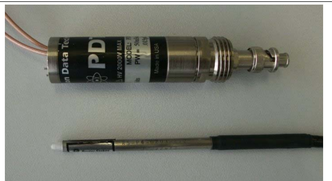
Figure 9: The gas-filled detector tube and amplifier/pulse shaper in use at DELPHI. The diameter of the detector is 6 mm only.
