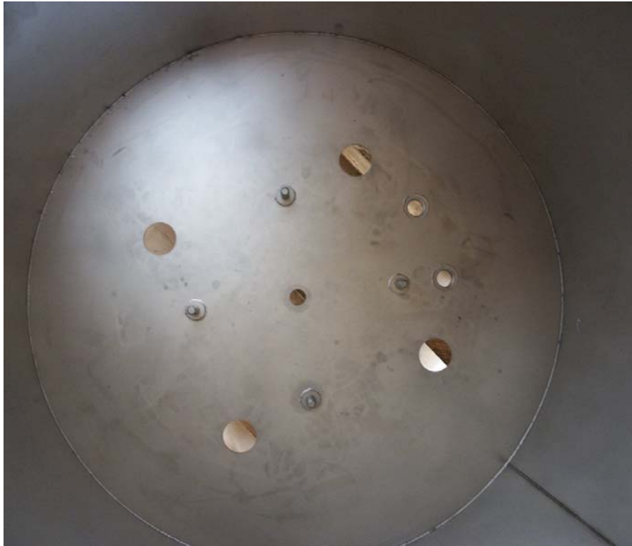
Figure 6: The bottom of the steel vessel. The four large holes will be used to insert spotlights, the central hole to connect a stainless steel tube for the source and the two remaining holes to fill and drain the vessel.
