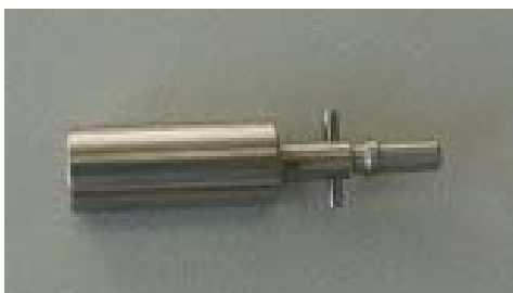
Figure 1A: The stainless-steel head for a fuel pin.
