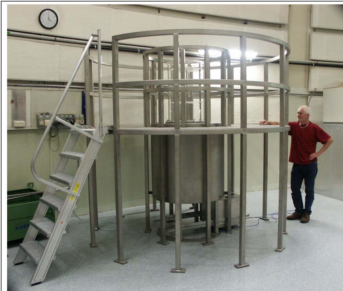
Figure 10: The main parts of DELPHI assembled together. Inside the loading platform, the steel vessel is mounted below which the drawer mechanism and the shielding box are seen. On top of the steel vessel, the acrylic vessel is mounted. Because of its transparency, this vessel is less visible.
