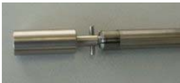
Figure 1B: The stainless-steel head grabbed by the special handling.
