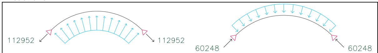
A. Principle 1 (Arched Structural System)
