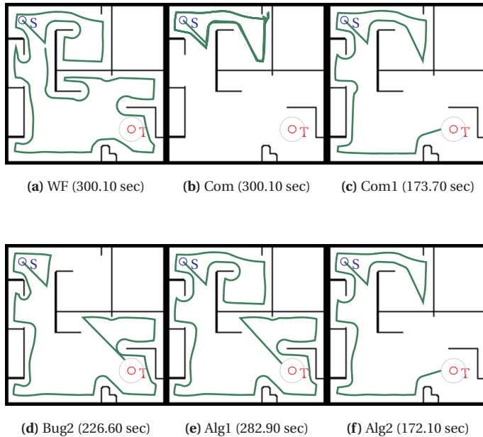
Figure 4.10: Behaviors of the implemented a) wall-follower (WF) and Bug Algorithms (BAs): b) Com, c) Com1, d) Bug2, e) Alg1 and f) Alg2 in one generated environment. The BA starts in the top left corner at Start (S) and ends within 1 meter radius from the Target (T), with a time-limit of 300 seconds.
