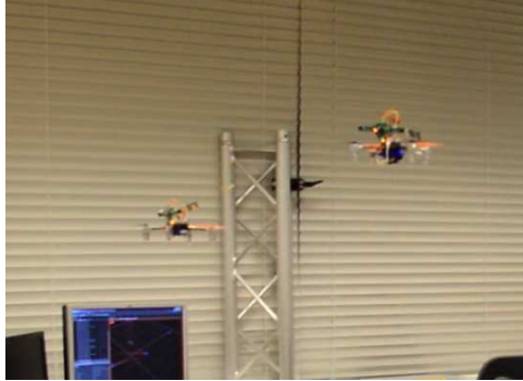
Figure 3.1: Two pocket drones (40 g each) flying autonomously in a real-world indoor environment using only on-board sensing and processing.
