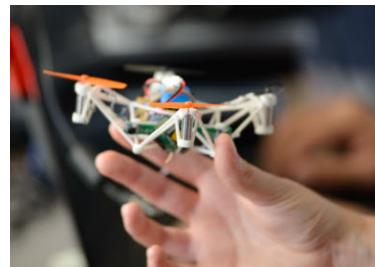
(b) 3D printed frame with a Lisa-MXs autopilot
