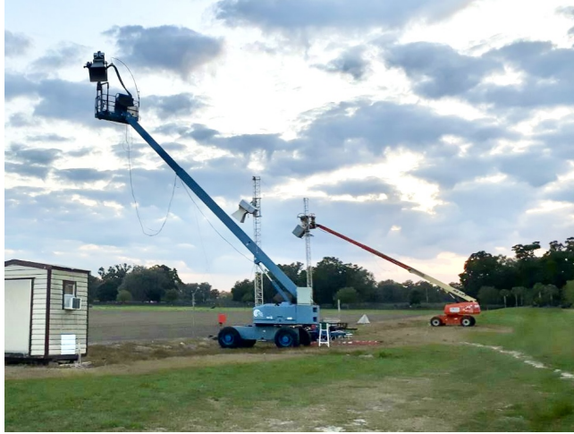
Figure 2.2.: The University of Florida L-band Automated Radar System (UF-LARS) is mounted on the blue crane
