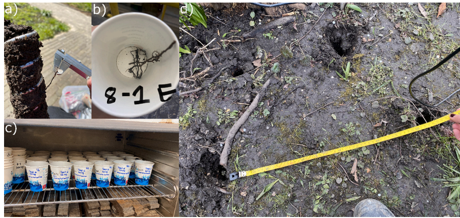
Fig. 3. Collection and processing of corkscrew extraction samples. a) Root diameter measurement using calipers. b) Root collection from the extracted soil sample. c) Water content measurements and drying of roots in an oven. d) Holes formed in the embankment after corkscrew extraction.
