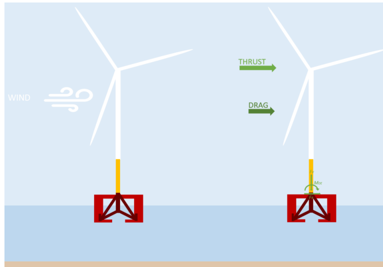
Figure B.1: Wind Forces during Transport Stage
