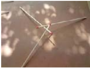
Fig.2 Basic reciprocal principle. (Larsen O.P., 2008)
