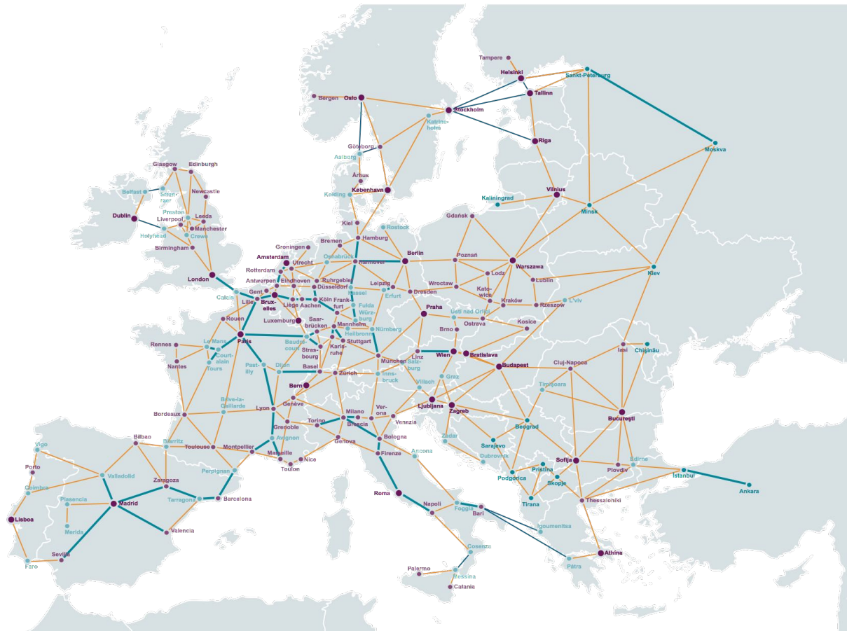
Figure 2.5 – Modelled railway network 2015. (Dark green = HST, orange = conv., blue = ferries), (Own elaboration).
