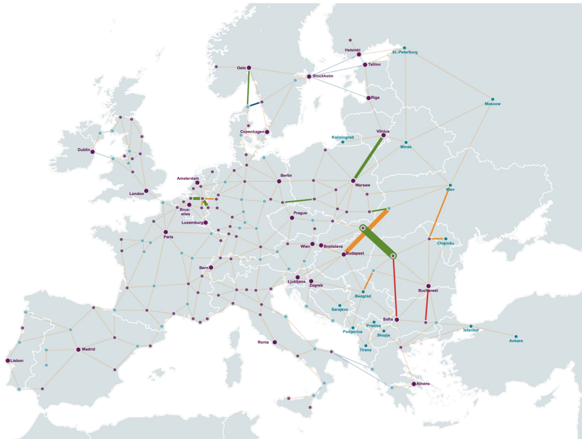
Figure 4.8 – International links with transfers; green = optimised transfers, orange = average waiting time, red extreme wait for transfer, (Own elaboration).
