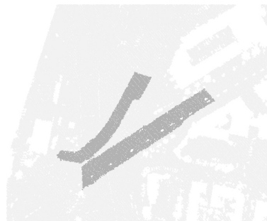
If a bridge segment boundary contains more than one across edge it is labeled as bridge. In the figure above the two overpasses have been identified.
