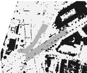
After the bridges are identified the macro objects (detected earlier) are put back into the point cloud.
