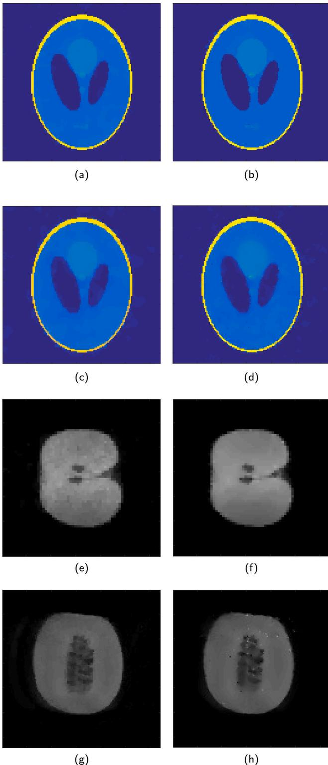
**Fig. 12.** Images of the Shepp-Logan phantom using simulated data with an SNR of 20 (top row) and an SNR of 5 (second row), an apple based on measured data (third row), and a melon based on measured data (bottom row), using additive regularization (left column) and multiplicative regularization (right column).
