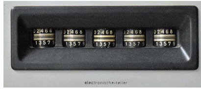
Figure 7. E1T based counter from the console of the former nuclear reactor
