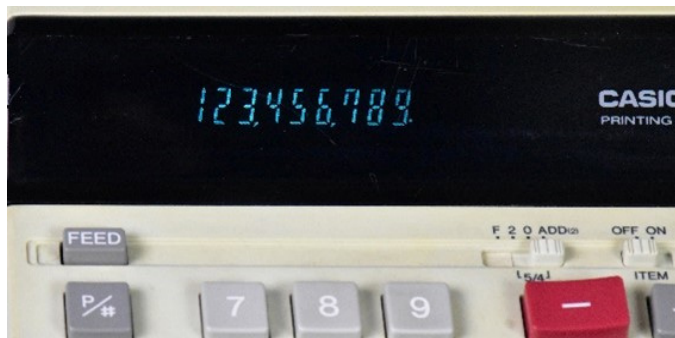
Figure 12. Casio FR 310 Printing Calculator using seven-segment indicators
