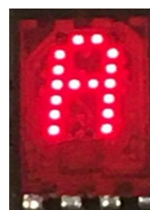
Figure 14. HP 5082-7340 4 by 7 led dot hexadecimal indicator (not to scale)
