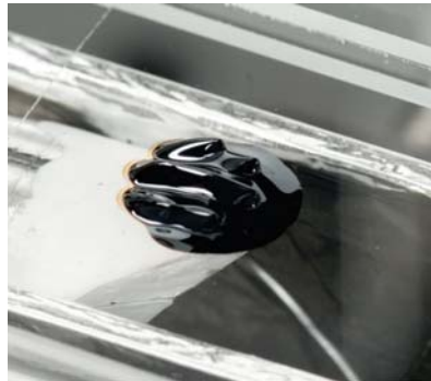
Figure 3.9: Visualization of the magnetic field by ferrofluid. Spikes are formed on the ferrofluid since the stray flux coming out of the magnet unit is bended upwards.
