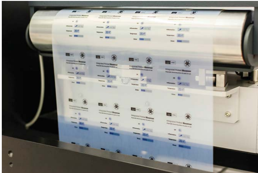
Figure 1.4: A foil roll that contains rows of “integrated printed biosensors”. Courtesy of Acreo Swedish ICT [10].
